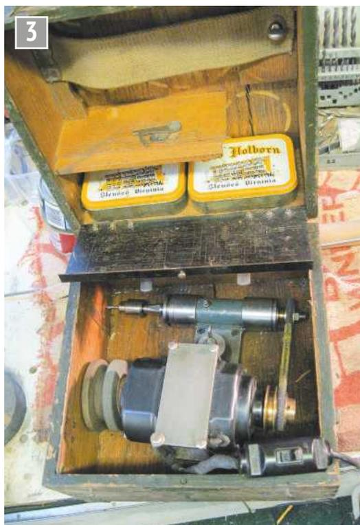
The tool-post grinder in its massive wooden box.
