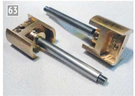
63 Completed crossheads and piston rods.
