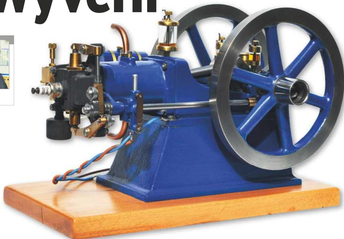
**E**dgar T. Westbury's Wyvern open crank internal combustion engine is typical of many of his designs in that the camshaft is driven by crossed helical gears, often called skew gears. As in most four stroke engines, the camshaft rotates at half the engine speed so the camshaft drive incorporates a 2:1 reduction. The skew gears give a convenient change of direction so that the rotation of the camshaft is at right angles to the crankshaft, allowing
