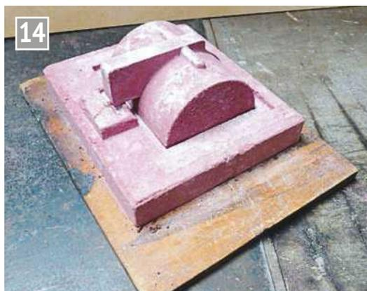
The core ready to be assembled with the outer.
