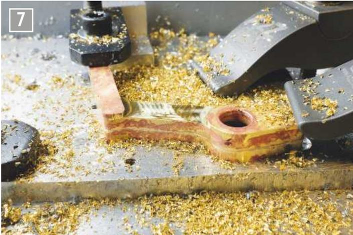
Second CNC machining operation. An aluminium jig is held to the table by two clamps; a further two clamps holds the turret to this jig. One can see that the radii cut in this second operation closely match the radii of the first cut.
