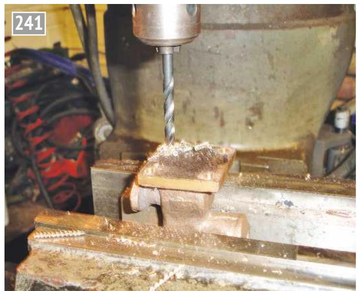
*Drilling the pump body.*
