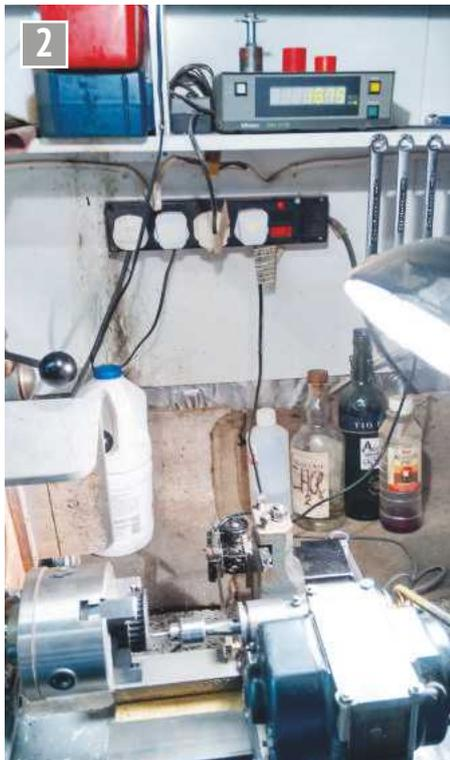
*A view of the read-out from the cross-slide. A 6 inch Mitutoyo calliper is cable connected to a Model SD-D1E display and is about 20yrs old.*
