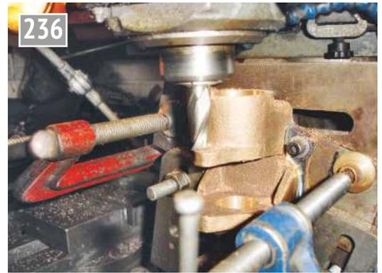
*Machining the seating for the nut.*
