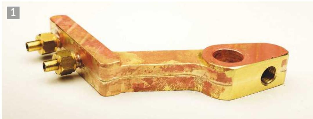
**1** Completed turret awaiting painting, fitting and hydro testing. Connections on the left are for pressure gauge and lubricator; on the right is the hole for the holding bolt and the tapped hole for injector steam valve.
