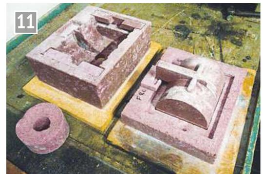
The sump core and mould.
