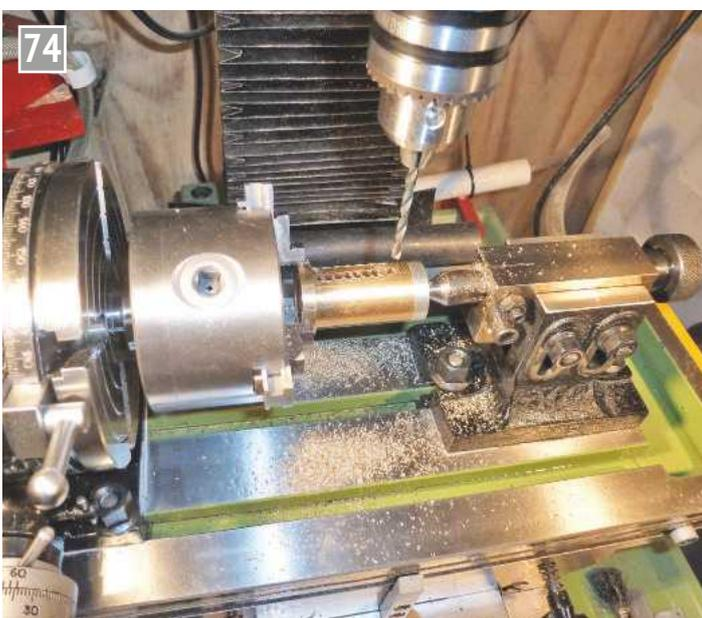
74 *Initial drilling of the guide side apertures.*
