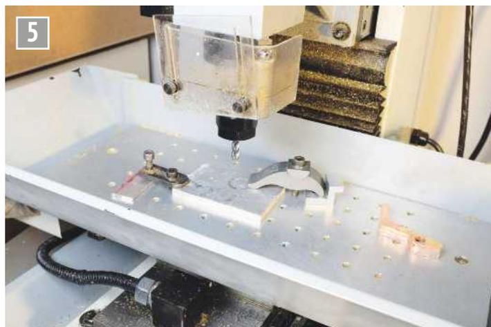
For the second CNC operation, a bit of aluminium was used to create a pocket to hold the embryo turret for further machining. Creating a pocket this way keys the part to the table such that it is automatically aligned for further CNC machining.
