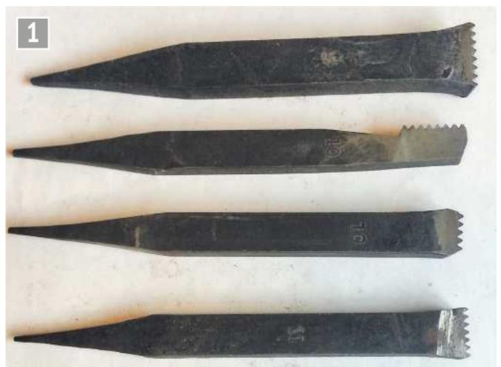
The application of zero rake angle applied to screw thread chasers.
