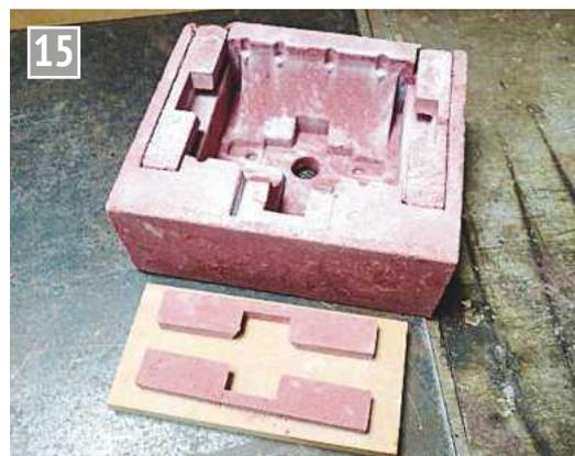
The assembled sump mould.
