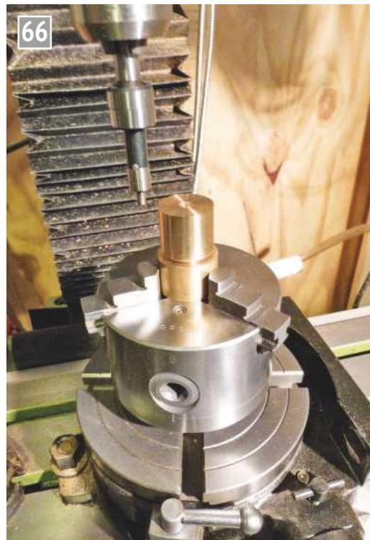
66 Using an edge finder for a datum on the outside of the crosshead.
