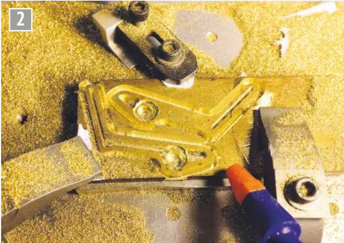
Brass sheet being cut with a 3mm endmill; air jet used to clear away swarf.
