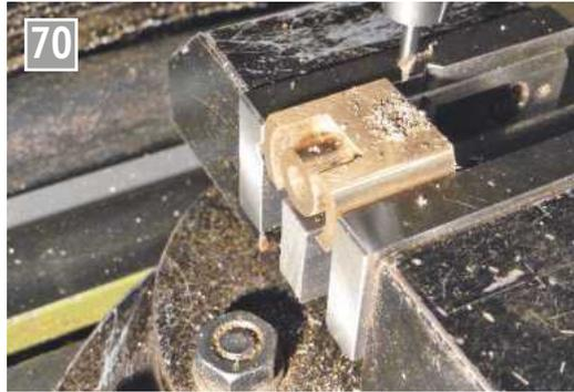
70 Centre drilling the crosshead for the wrist pin hole.
