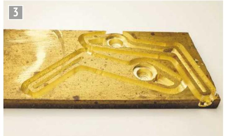
Finished cutting outlines and interior passages. Requires cleaning up and separating by skimming material off of the underside, leaving parts and remaining support material interconnected by holding tabs.
