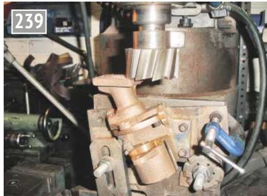
*Machining the pump body.*
