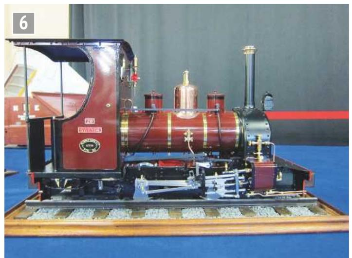
The well tanks occupy much of the front end of the locomotive, beneath the smokebox.
