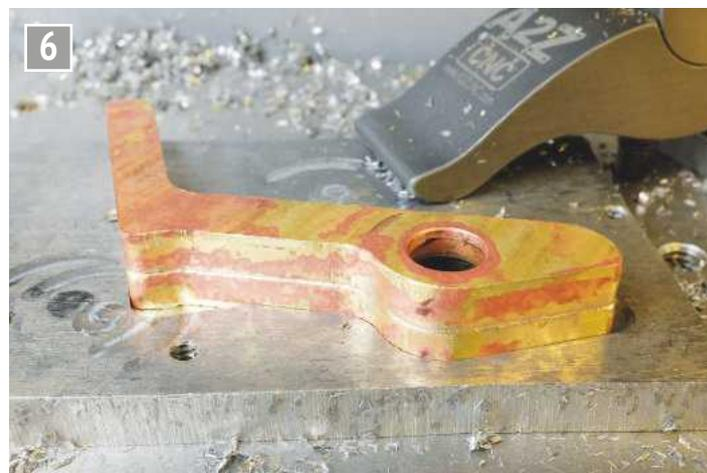
Turret bedded into the pocket. The pocket does not trap 100% of the turret but holds enough securely and in alignment. On the bottom left and right hand sides one can see that the pocket extends past the turret. This simplified the need to accurately de-burr the entire bottom of the turret.
