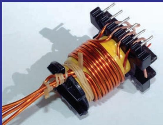
Then on go the secondaries. As with the primary winding, this should be nice and tight. The rubber bands are removed before adding the final layer of tape. As before, fit PTFE sleeving over the wire ends before terminating them to the bobbin pins.
