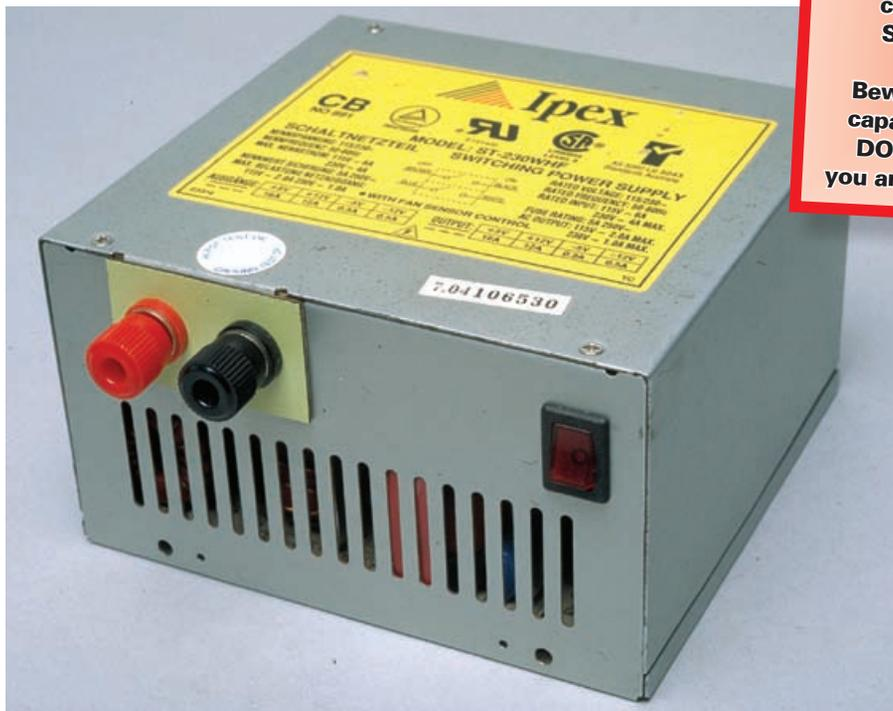
One of the nice things about using an old PC power supply is that it already comes in its own case, complete with fan. Some even include the mains switch – though none will have the large binding post terminals! This is a typical XT/AT-type supply, rated at about 230 watts (and therefore capable of 13.5V at 17A). You often find these PCs junked in council clean-ups, etc.
