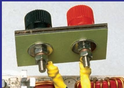
Add a pair of polarised terminals on their own mounting plate and fasten it to the power supply case, as shown at right.
