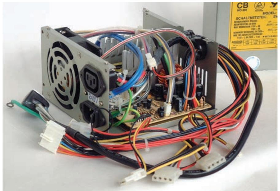
**Here's what you should find when you lift the lid on the switch-mode power supply. Usually it's only four or so screws to get this far. All of the external cabling will be removed. Never run the supply with the lid removed unless testing – and then only with extreme care. These things can be lethal!**
