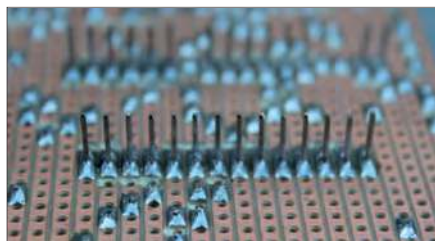
Fig.4. Close up of the underside of the DM showing soldered pin strip J11.
