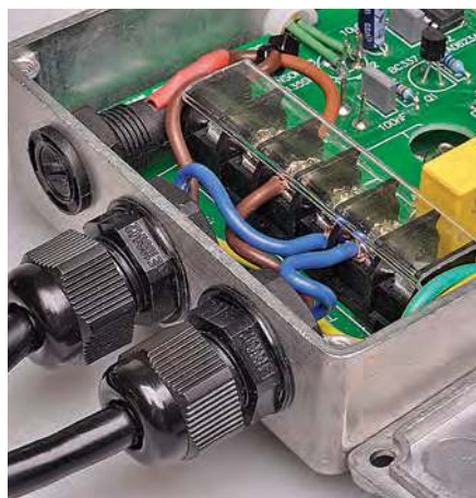
Close-up view of the mains input and output section of the Heater Controller . Don't forget to place the protective shroud over the mains terminal block.
