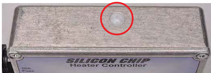
Fig.4: this diagram and the photos at right and below show how the sensor is mounted, with its lens emerging through an 11mm hole drilled through the side of the case.
