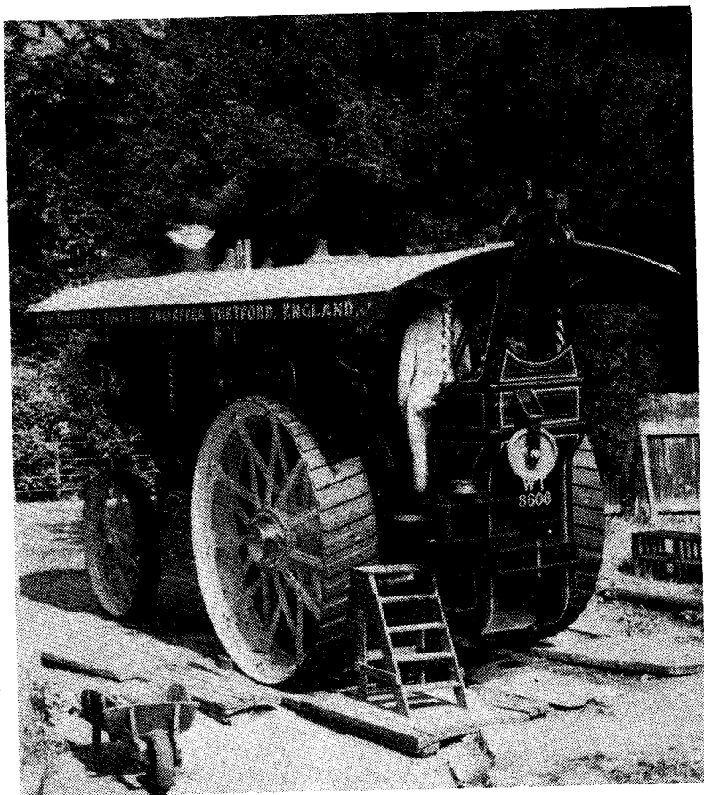
The engine has a crane turret and pulleys to allow use of winding rope
