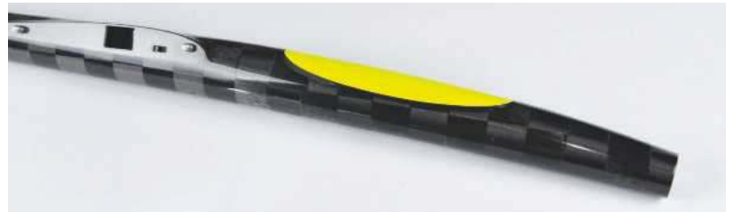
Droop snoot! The fuselage bends at the front to take up the correct down thrust.
