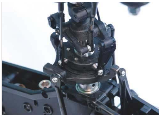
A new design swashplate is supplied, with a plastic lower half and metal upper.
