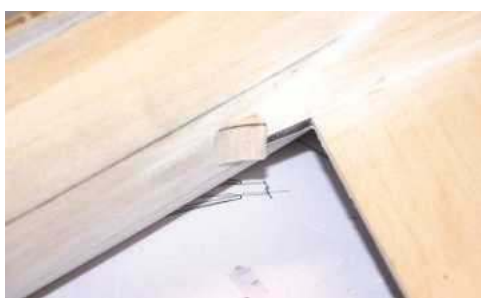
Tidy up at the back by adding the rear wing fillets.
