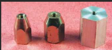
Sometimes you need to make a spinner adapter from ye rough-hewn hex bar.
