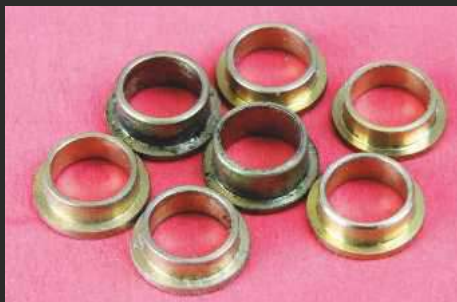
These oily shaft adapters are home made. The shiny ones didn't fit my engines!
