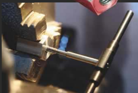
Turning a spinner adapter is a doddle on any lathe. You can tap any size, too.
