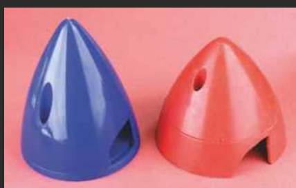
Plastic spinners can be variable in quality. Nylon is better, but not best.
