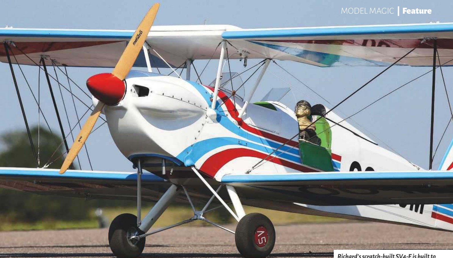
Richard's scratch-built SV4-E is built to 1/3rd scale, spans 110" and weighs 32lbs.
