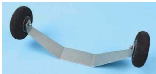
Although a Dural undercarriage is shown on the plan one could easily be fashioned from piano wire, or even dispensed with for rough field use.
