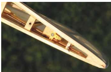
Concealed linkages. The rudder plugs into the yellow servo arm, whilst the elevator hooks onto the protruding bit of piano wire, so there are no external horns on the tail surfaces to get caught in their travel bag. It all makes sense, eventually.
