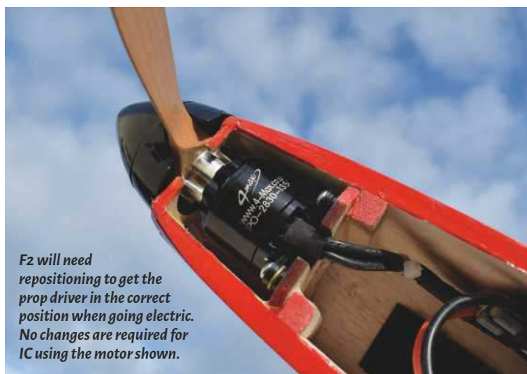
After a quick phone call to 4-Max, George recommended this motor and speed controller as suitable for the Sssshhwept.
