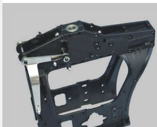
Side frames bolted together with the elevator lever assembly. The frames are exactly the same as my 24-year old ZXX!
