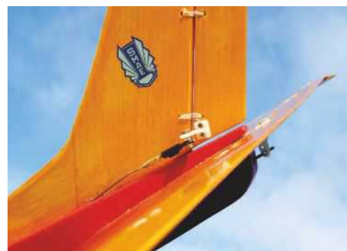
Tail and fin are simple sheet items but don't forget the slot in the tailplane otherwise you will have great difficulty fitting the elevator pushrod.
