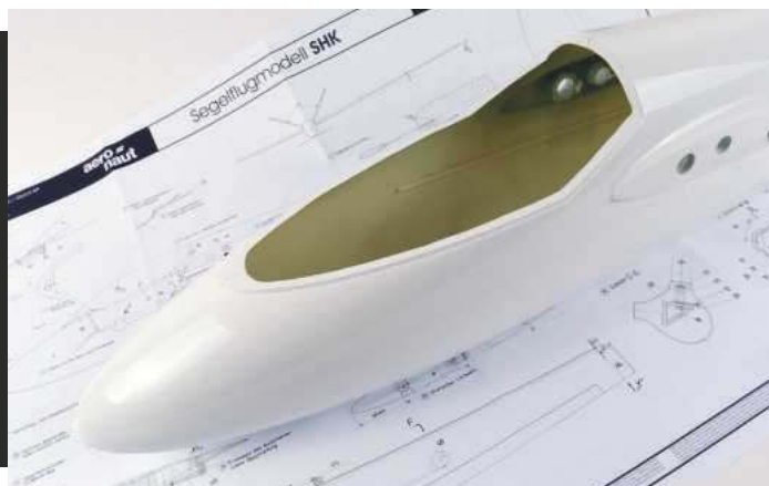
The gel-coated fuselage is moulded using glass fibre. The finish is excellent.
