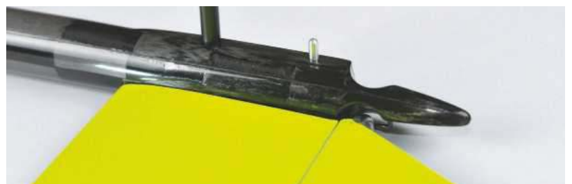
The elevator halves simply slide onto a carbon rod and a short metal incidence peg. Note the rounded cut-outs to give clearance for the control horns.
