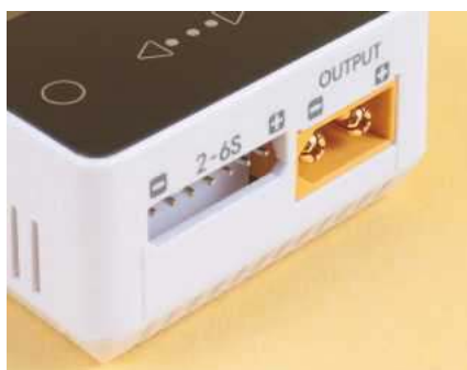
XT60 sockets are used for input and output. Note the servo and USB terminals too.
