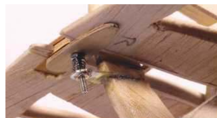
Beneath the tailplane, the 2mm bolt passes through a matching nut that's secured to the fin. The little spring prevents it all from shaking loose in use.
