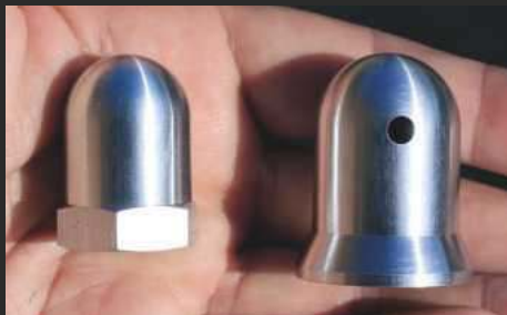
Two of Nick Banks' designed early four stroke cover nuts from bar stock and hex.
