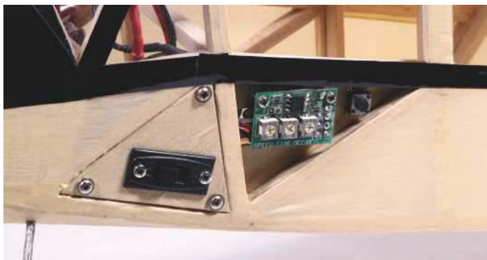
The motor's arming switch and control circuitry are easily reached just prior to hand launching. The three adjustment pots do their jobs very well.
