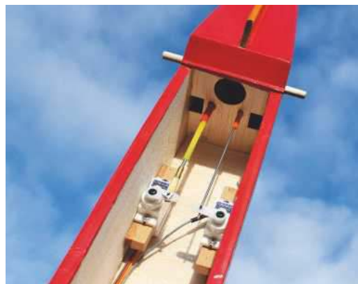
There's no shortage of space for 9g servos. As always ensure that the linkages are as direct as possible, especially if using piano wire pushrods.
