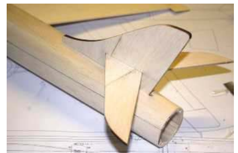
Test fit of the tailplane and fin before shaping.
