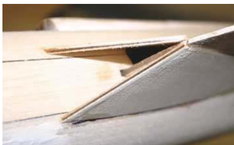
Intake edges are lined with 3mm square scraps of lite ply to strengthen the intake lips.
