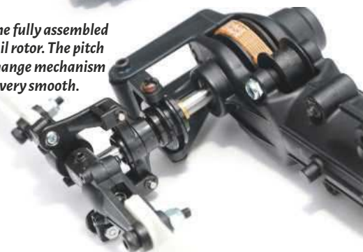
Hirobo supply the tail rotor spindle ready assembled.
