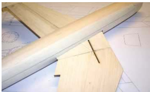
The wings will need to be slid into position from one side. A little fettling may be needed to get them to fit properly.
