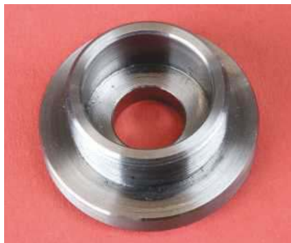
The mild steel baseplate has a recess in the boss to accept a standard socket - sweet!
