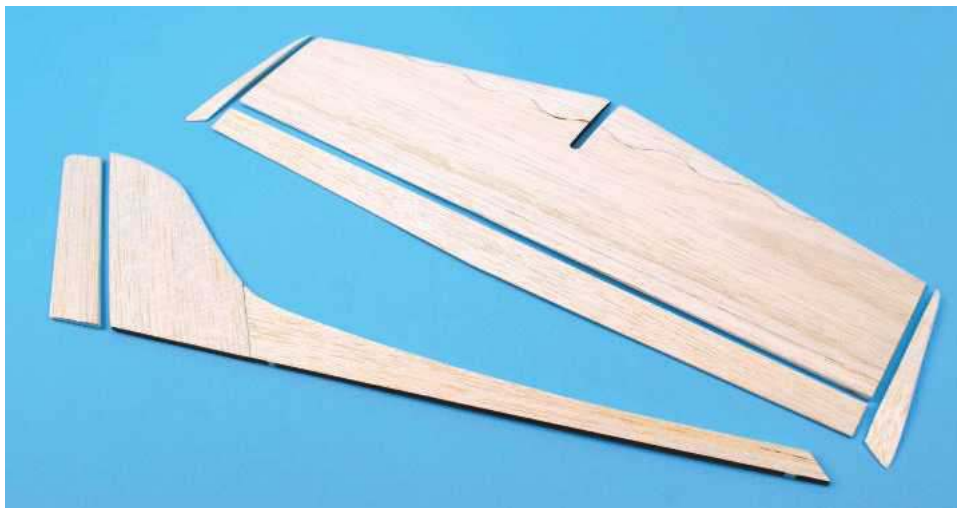
Tail and fin are simple sheet items but don't forget the slot in the tailplane otherwise you will have great difficulty fitting the elevator pushrod.
