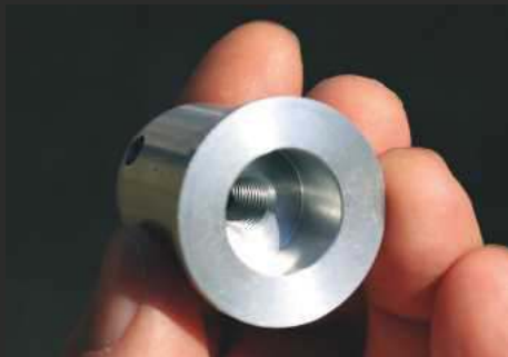
Round stock hollow dome spinner. Note the clearance for the lock nuts.
