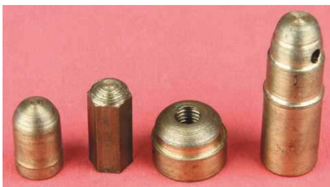
Home-brew heavy dome nuts and an early ali spinner from my lathe.
