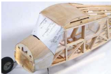
A scrap of paper becomes a template for the curved windscreen. I like templates, I do!
