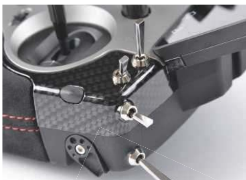
This top corner view shows one of the momentary switches fitted to the edges of the carbon effect case.
