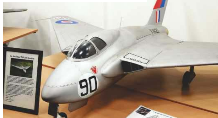
Jamie Cuff's Westbury Kits/Jetline Models DH 108 Swallow . A JetCat P80 provides the necessary thrust.
