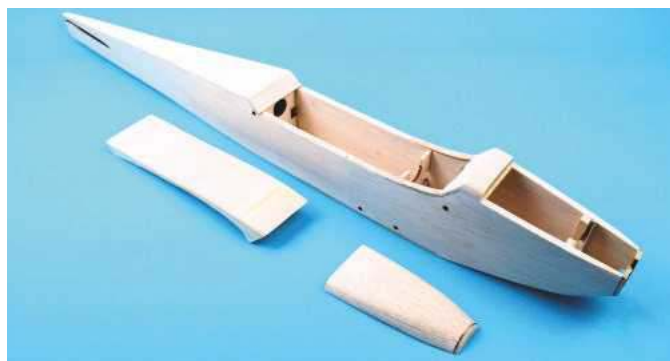
Although basically a box fuselage, Sssshwpt involves a little more work to construct than simpler trainers of the day.
