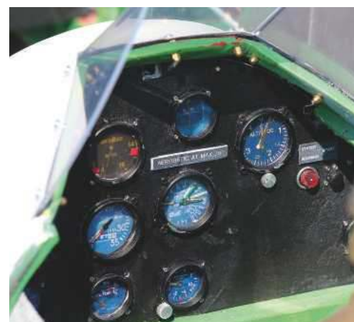
Richard home 3D printed all the instruments. Watch hands are from ebay.
