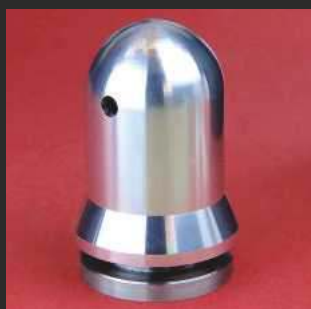
Nick Banks' elegant spinner solution for internally threaded crankshafts.
