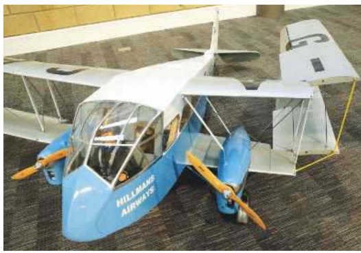
John Rickett's DH Dragon 84 spans 11' 10" (3.6m) and is fitted with two Laser 155 engines.
