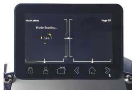
Loading the current model memory as the Linux systems boots up. It takes around 25 seconds to complete.
