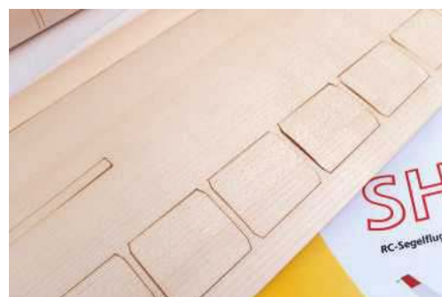
Laser cut wing and tail sheeting is beautifully done.
