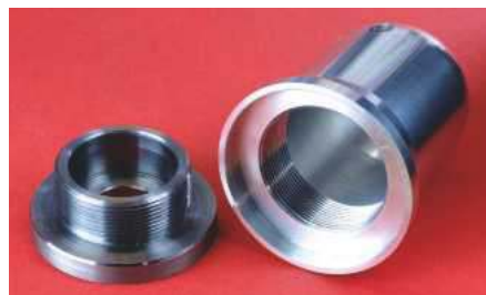
A Banks new cover nut from mild steel baseplate with its 6000 series aluminium dome.
