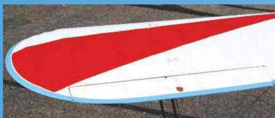
Ailerons are on all four wing panels, complete with scale control runs.
