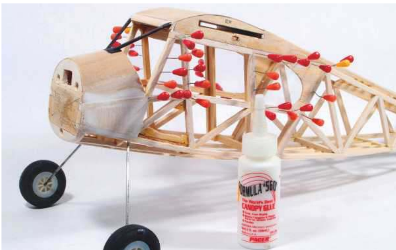
Here's the side glazing being attached to the fuselage. Canopy glue and lots of pins are my preferred method. I left the central panel open to allow access to the internal wiring.
