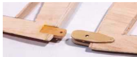
The ply plates on the TE of the tailplane sandwich together to keep them in place.
