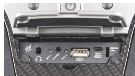
Flip up panel below the power button reveals a series of sockets and ports.
