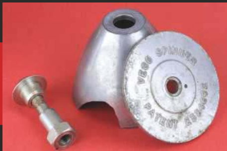
Veco were early adopters of aluminium spinners. Note the fixing arrangements.
