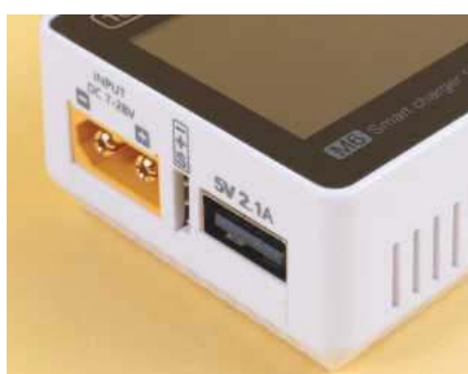
XT60 sockets are used for input and output. Note the servo and USB terminals too.
