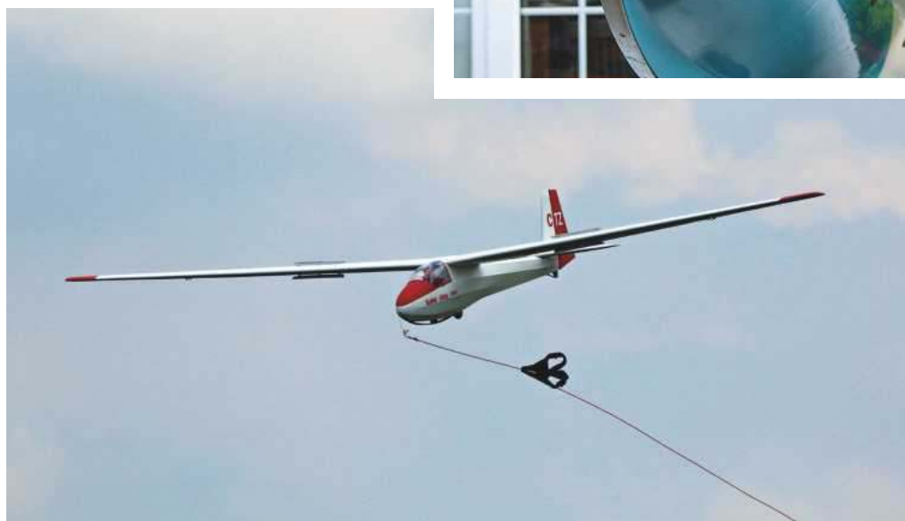
One of the more minor consequences of a non-functioning release - a trailing tow line and embarrassment for the glider's pilot!
