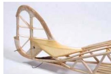
Starting with the trickiest bit to cover, cream Litespan was bullied into adhering to that concave area at the base of the fin. Makes the rest of the model seem very easy!
