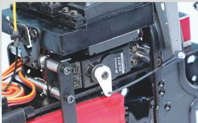
Another JR DS811 fits under the servo tray, working the collective pitch lever.
