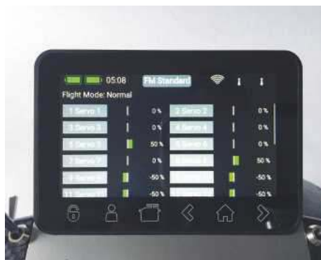
The servo monitor operates in real time, with no delay.
