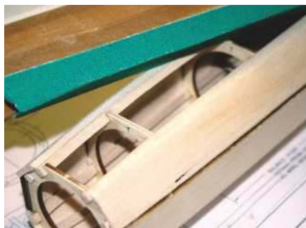
Bevel the edges of the side sheeting before adding the top and bottom pieces.
