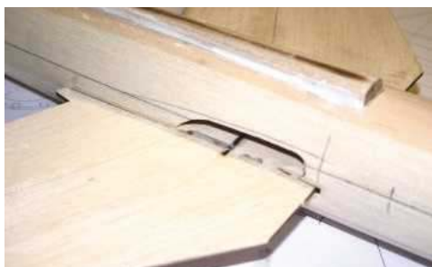
Intake openings are cut in the fuselage sides above and below the wing.
