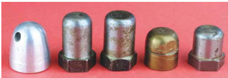
Home-brew heavy dome nuts and an early ali spinner from my lathe.
