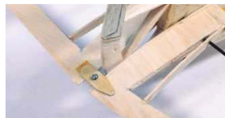
The halves of the tailplane are locked together by a 2mm bolt, passing through those ply tongues aft of the fin.
