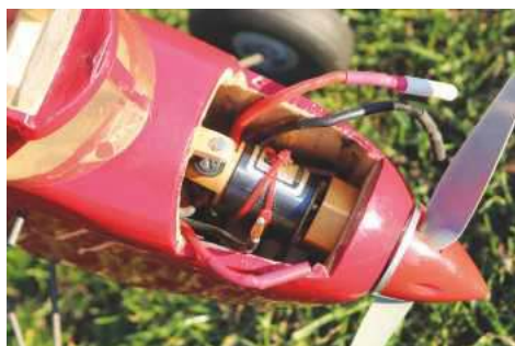
The height of technology at the turn of the century, an Astro15G no less. Lots of gear noise and carbon dust. The yellowed windscreen is a collector's item these days.
