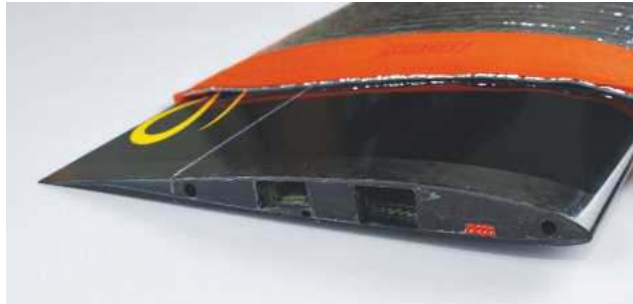
Far left: Aileron and flap servo extension leads are factory fitted. Just visible is the pushrod to activate the internal Integrated Drive System.
