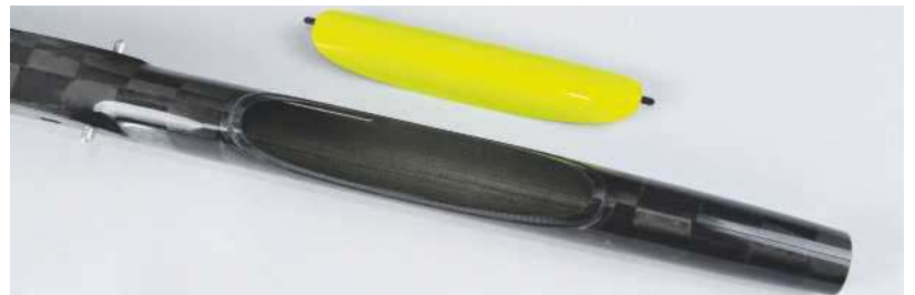
The hatch is handed, so make sure to mark it inside to ensure a good fit.
