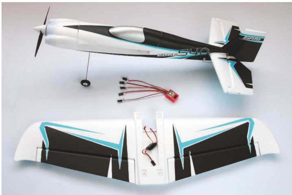
It's truly ready to fly - just fit the wing, Rx and flight controller (orange unit) and slot in the U/C.
