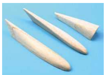
Vortex tips and cowl fairing are carved from balsa block. A bit of proper aeromodelling!
