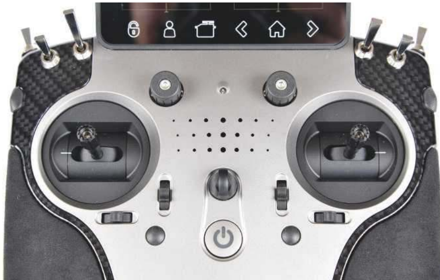
Main sticks units are machined from solid metal, with fully adjustable sticks and ball-raced gimbals.
