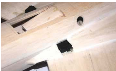
Sink the aileron servos into the fuselage sides under the wing.
