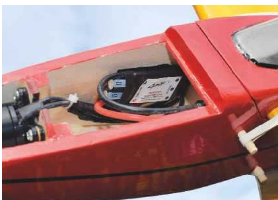
F2 will need repositioning to get the prop driver in the correct position when going electric. No changes are required for IC using the motor shown.
