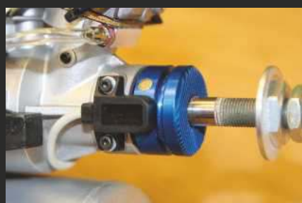
Threaded crankshafts cannot be left with just a prop nut!
