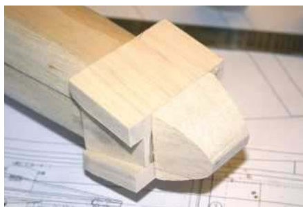
There is a lot of shaping around the nose and the balsa is there to be cut into to create the smooth curves of the Hunter.
