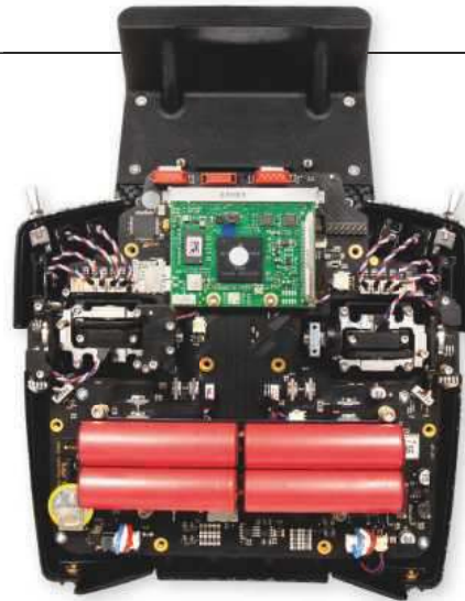
Inside view showing the internal layout and the two separate Li-ion battery packs. More redundancy is built in by using duplicate power regulation circuits. Photo: PowerBox
