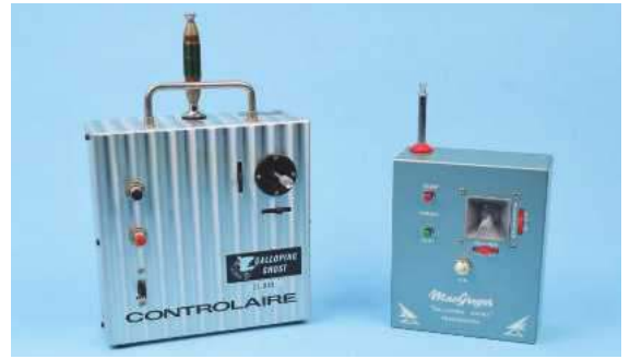
A couple of examples of popular Galloping Ghost transmitters - the US manufactured Controilaire on the left and a good old British MacGregor on the right.
