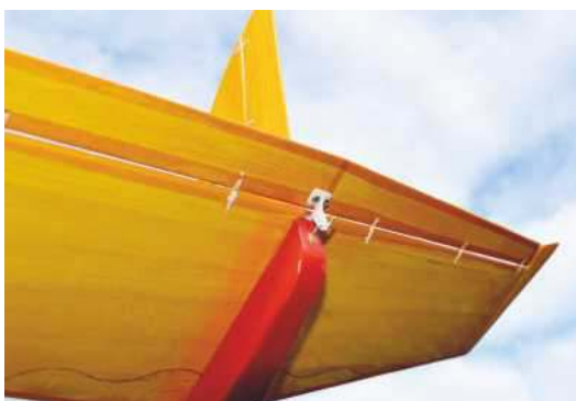
Tail and fin are simple sheet items but don't forget the slot in the tailplane otherwise you will have great difficulty fitting the elevator pushrod.
