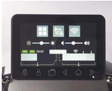
Swiping down from the top edge of the screen reveals the set-up menus.
