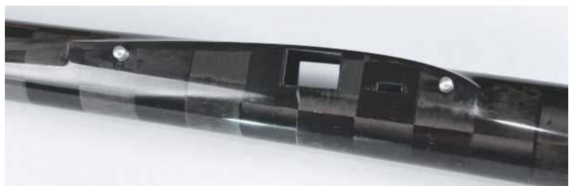
Wing mount detail showing the incidence pegs and the holes for the wing joiner and servo connectors. Use of spread tow fabric results in a smart chequerboard finish.
