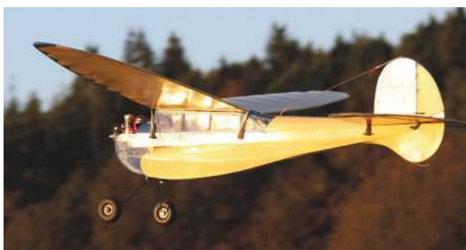
The doped Airspan, although fragile, reflects the afternoon sun in a way that the matt Litespan on my model never can.
