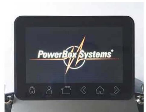
As when switching on, you need to press the power button twice to turn the system off. The PowerBox logo appears, to confirm that the Tx is shutting down.
