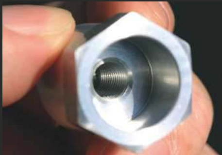
Hex stock hollow dome spinner. Note the thread for the retaining set screw or bolt.
