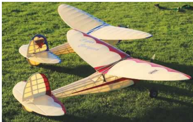
The joy of a built-up structure allied to a translucent covering medium. The Super Scorpion isn't a beginner's build by any means but is very rewarding all the same.
