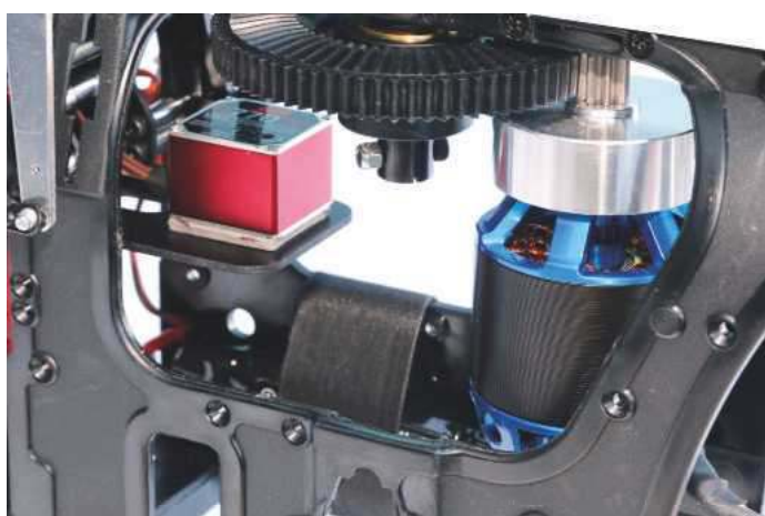
I fitted a JR G770 gyro on the gyro platform inside the chassis.
