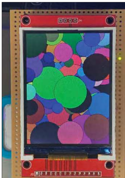
Fig.6. Typing the command GUI TEST LCDPANEL should result in the display of this animated test-pattern.
