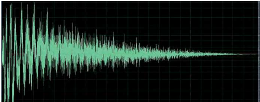
Fig.1. Roland TR909 Snare drum hit – note the large amount of noise in the signal.
