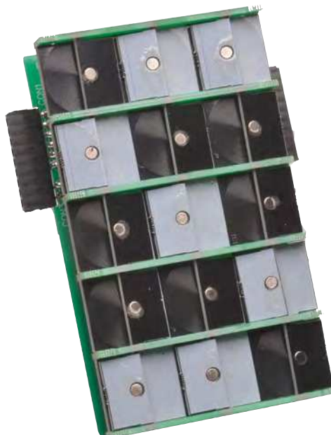
One complete unit – here displaying the letter 'S' – sits upright of its own accord. We have fitted a small length of female header strip to CON1 and CON3 to allow connections to be made with jumper wires. See video: siliconchip.com.au/Videos/Flip-dot
