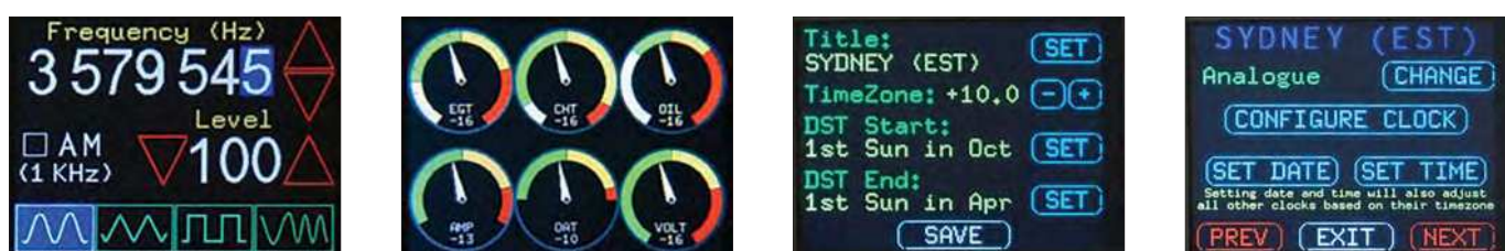
Fig.1. The 2.8-inch touchscreen used this month lets you create impressive interactive user interfaces.
