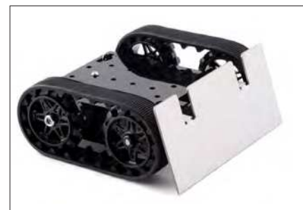
Fig.16. The Micromite Robot Buggy featured next month is based on the excellent Zumo chassis.
