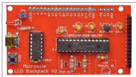
Fig.15. The BackPack PCB is a low-cost, yet extremely useful module to explore this month's topics.
