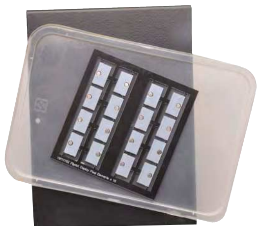
A small amount of epoxy resin is all that is needed to hold the magnets in the flaps. The steel panel (underneath) keeps the magnets flush, and the plastic inbetween stops the magnets sticking to the steel.
