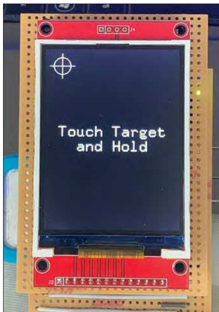
Fig.7. The touchscreen is calibrated with the command GUI CALIBRATE . Use a stylus (eg, a pen lid) and follow the on-screen instructions; ensure you accurately touch the centre of each 'target'.
