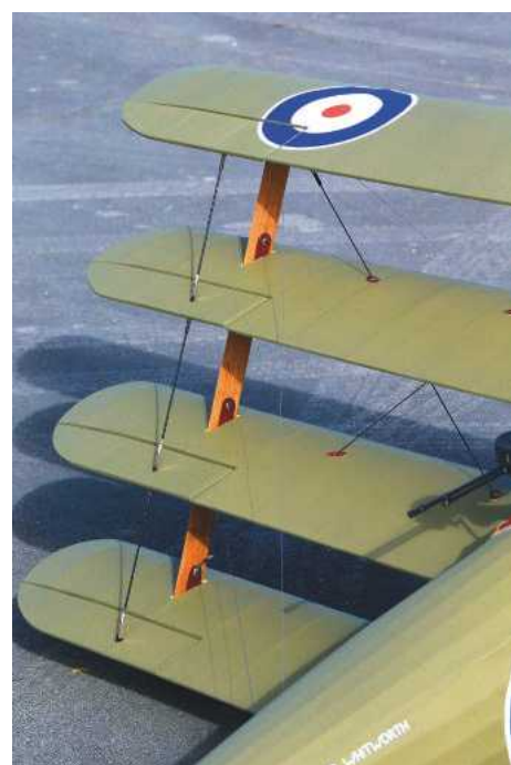
No nonsense ailerons and pushrods! Rib tapes are from ripped Solarfilm.
