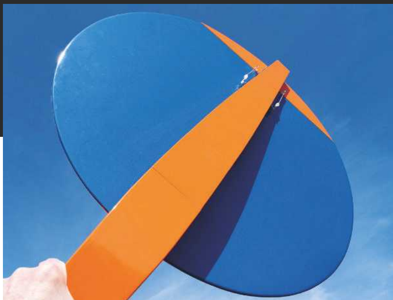
Use a contrasting colour scheme on the underside so you can orientate the model at distance.
