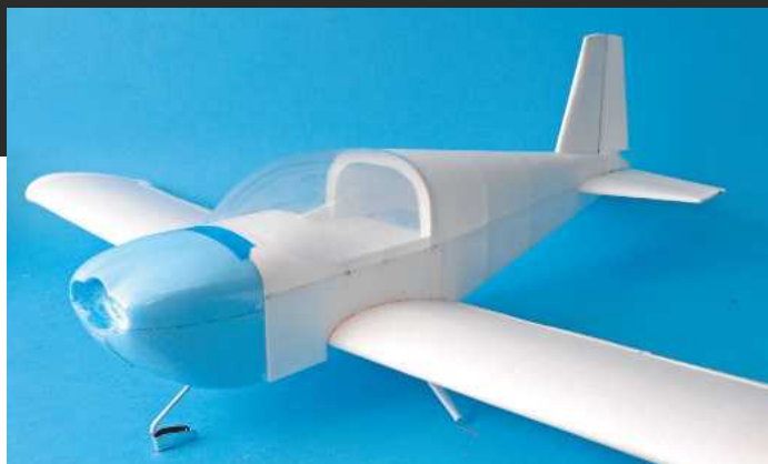
A quick inspirational assembly shot. The model at this point (not including the cowl) weighs 58g and includes four servos in the wing. My target weight is sub 110g for the 800mm span model.
