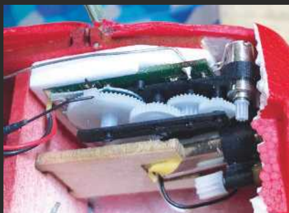
The control surface wire push has a joggle to fit the radio servo output.
