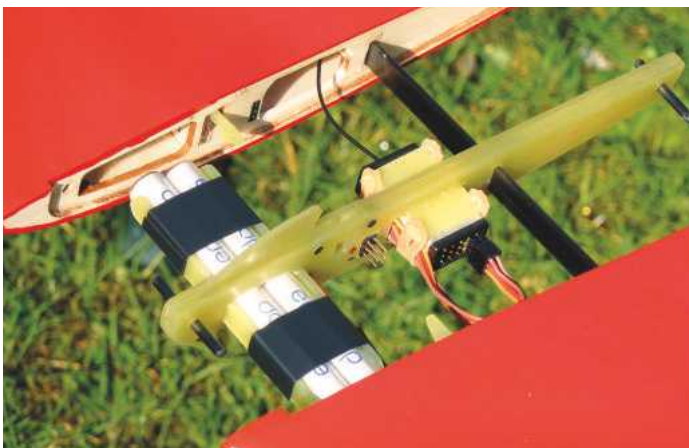
Assembly at the slope is easy. The wings self-lock onto the central rib and the electrics are lived up ready for flight.
