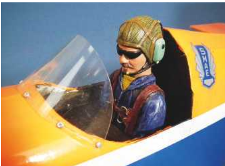
Above: Windscreen is a simple piece of plastic held down with tiny screws and canopy glue.
