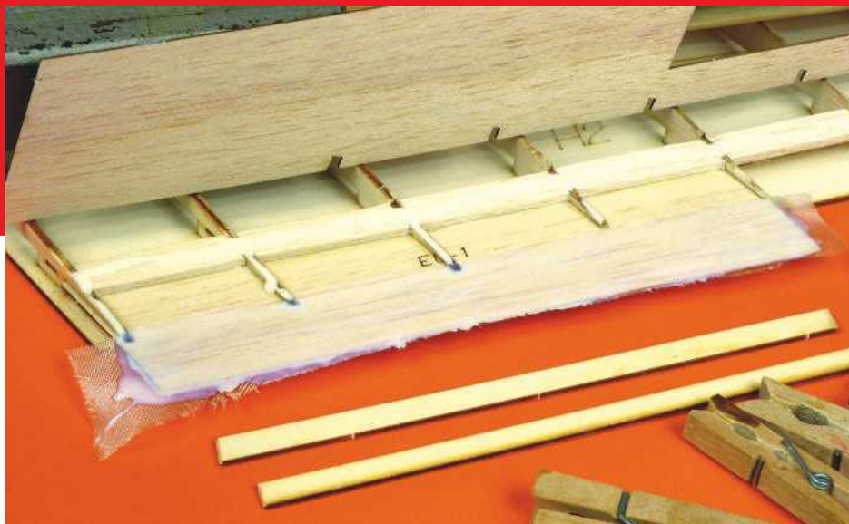
I added some glass cloth and Aliphatic glue to the top and bottom sheets in the first three bays to strengthen the sheeting. I could see this area being squeezed while assembling and dismantling the model so thought this a prudent move!
