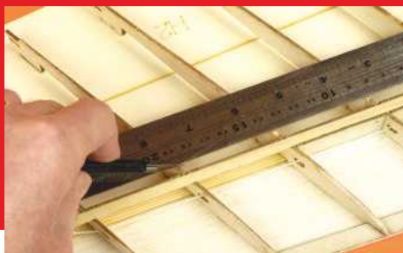
I trimmed the ribs so the top sheet butted neatly against the step in the top of the ribs.
