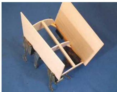
Glue the sheet on and leave the glue to dry. Then wet it and roll over the formers and glue down.
