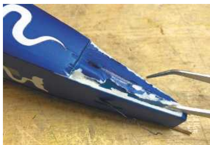
The damaged tail seat on my model before I cleaned it up with my nails.
