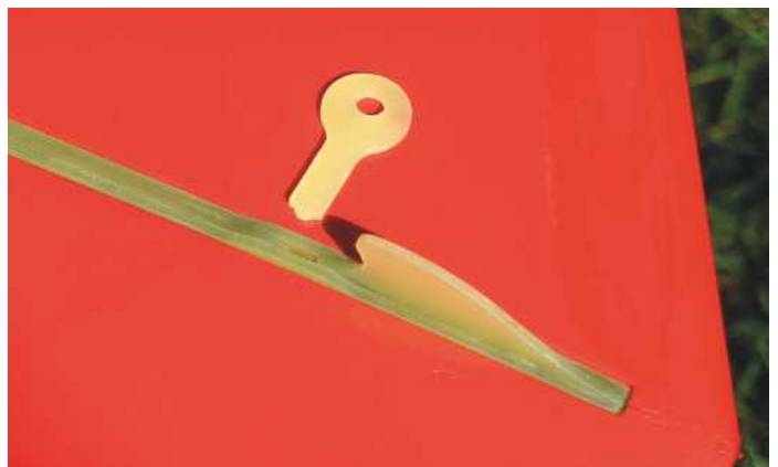
The keel protruding from the underside of the central rib is a handy grip for launching. It can also be used as a tow hook for a hi-start bungee. The key is used to separate the wings at the end of the flight and switch off the electrics.
