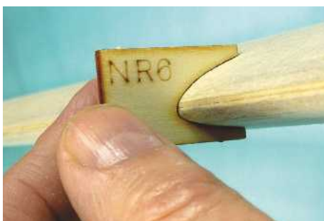
A set of four LE profile formers are supplied to ensure the wing LE is sanded to the correct shape – a nice touch!
