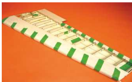
On go the TE and LE. Put the wing back into the jig and weigh down while the glue dries to keep the wings straight.
