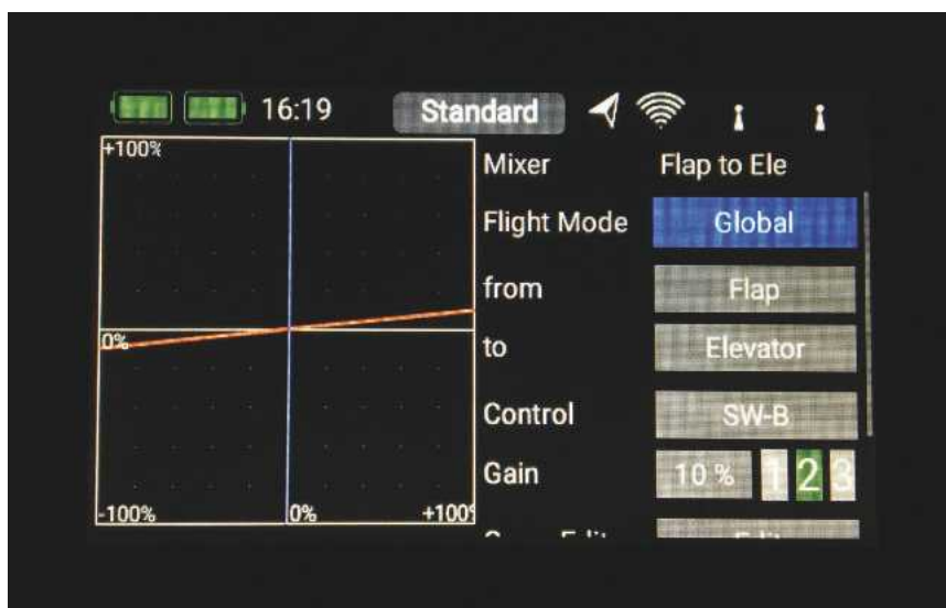
Free mixes are simple to program. Here are my inputs for some down elevator compensation when dropping flaps or using crow.
