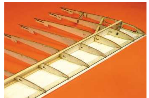
Vertical webbing being added to complete the D-Box construction. The webs are laser cut and that little dot signifies the top edge of each web.
