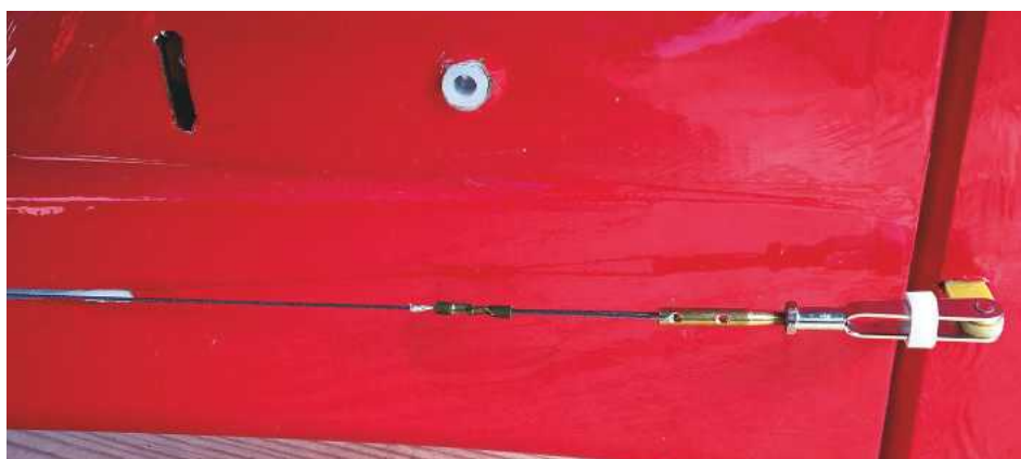
Ample adjustment is provided via turnbuckles at the rudder.
