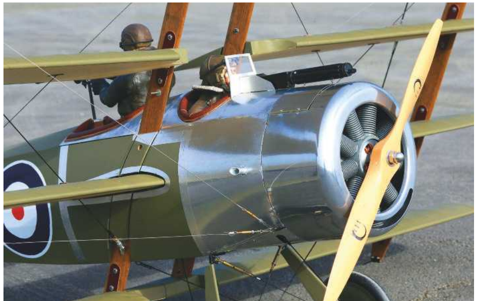
DB Models Pup cowl, which Tim polished. Cowling panels are from Flair Aluclad.
