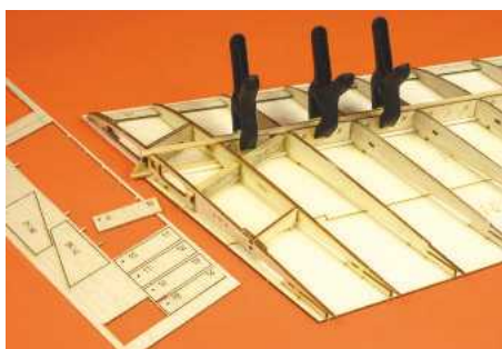
Vertical webbing being added to complete the D-Box construction. The webs are laser cut and that little dot signifies the top edge of each web.
