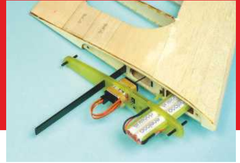
A final check of the assembly before gluing the servo sockets into the roots and adding the bottom root sheeting.
