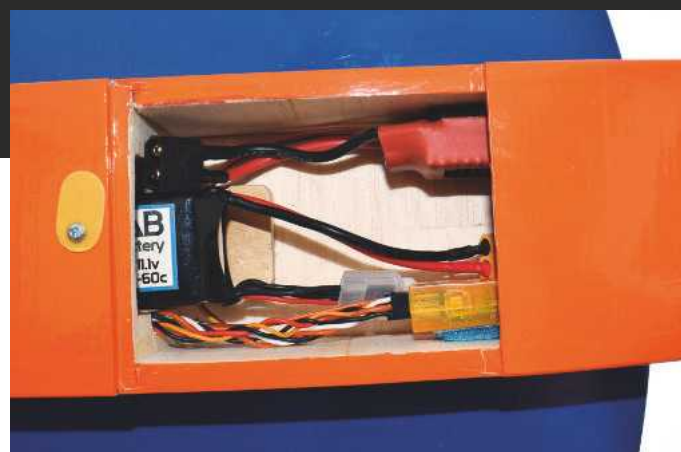
The lower fuselage hatch gives access to the LiPo. A laminate of balsa and lite ply was used as the model would be landing on it.
