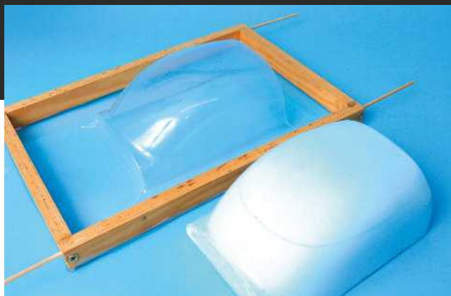
Availability issues during the lockdown means I have had to use clear styrene, which is not as clear as PETG. But needs must.
