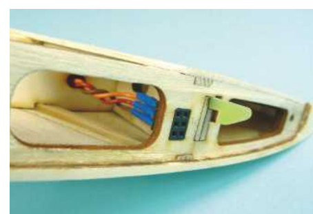
The double servo socket goes in the right-wing root. It connects the servo and also powers up the electrics when the wing is slid into place.
