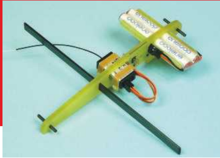
A final check of the assembly before gluing the servo sockets into the roots and adding the bottom root sheeting.
