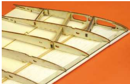
Pictures of the wing with the bottom LE sheet and bottom spar in place. The ply false LE has also been fitted.
