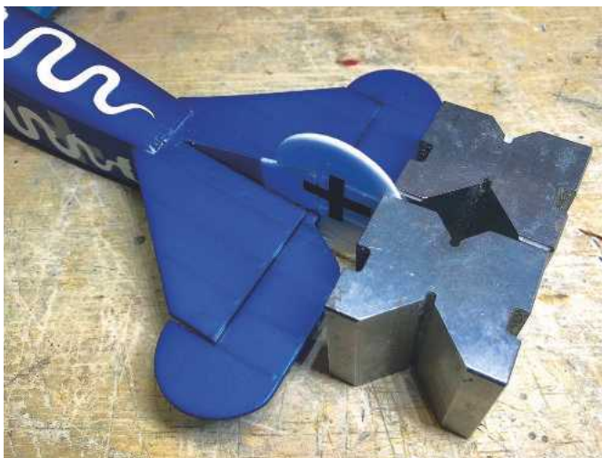
I used my engineers' blocks to glue the re-set fin square to the fuselage.
