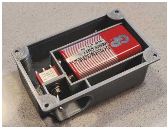
The Colour Wattmeter is powered by a 9V battery, all housed in a neat 3D printed case.
