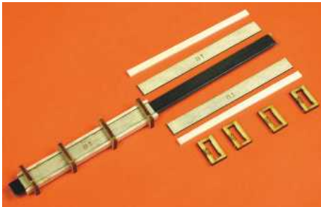
Joiner boxes have to be built up. Those square doughnuts are formers to hold it all together while the glue dries. Remember to wrap the CF joiner in tape and a coat of Vaseline or silicon grease to stop it sticking!
