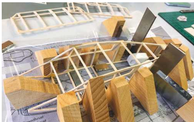
Small doesn't mean speedily built. The tricky part was fuselage alignment; those magnetic squares were a godsend.
