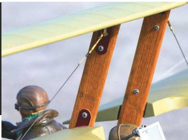
This view exemplifies the strength of the jig-built hardwood strut arrangement.
