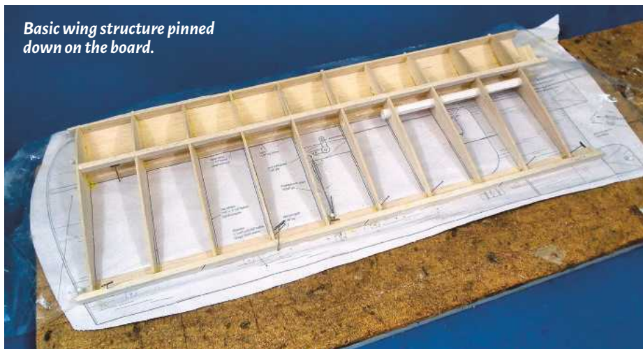
Map pins are the best way to hold the sheet down while the glue dries.
