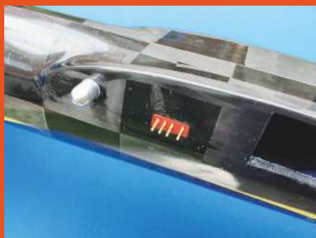
Above: The wing servo plug sits flush against the fuselage side. I'd caution against testing it for fit the 'wrong way' around!
