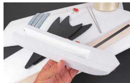
I like the way the underside fuselage protects everything and provides something to grab hold of for launching.
