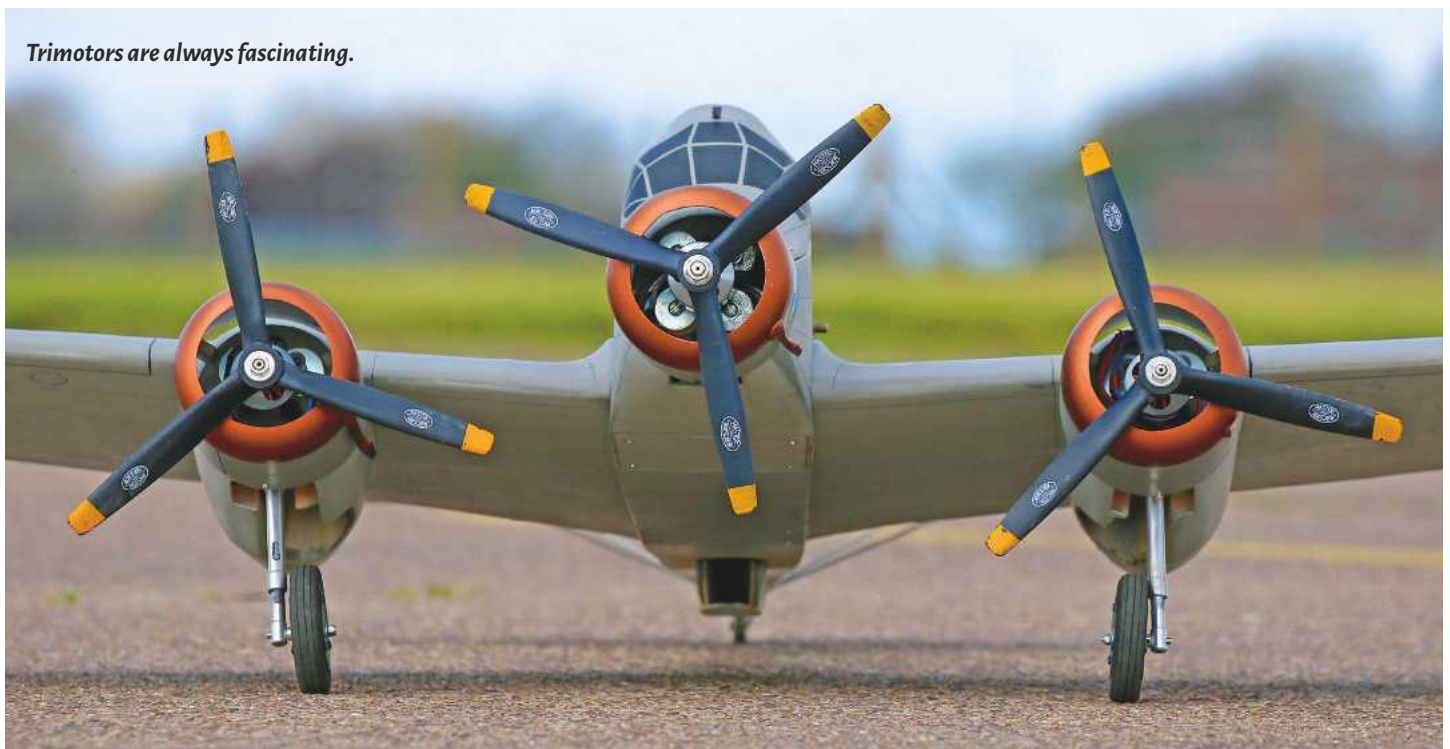
The electric powered SM.79 uses three 500kV outrunners.
