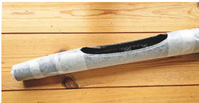
Masking around the radio bay stops any wayward drips of epoxy from attaching to the pristine carbon fuselage.
