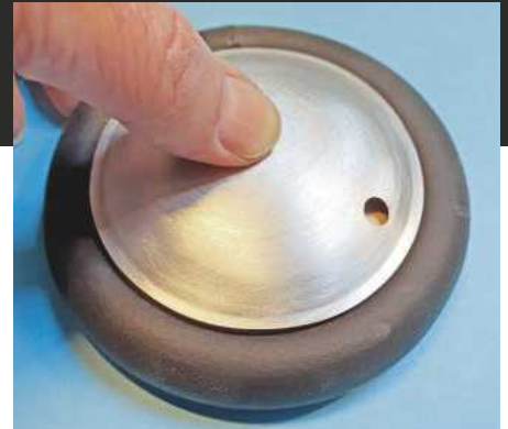
A trial fit proves that everything is well. I have made a hole for access to the tyre valve.
