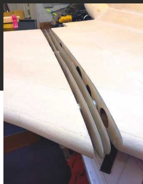
Sandwiching the wing root veneers before gluing.
