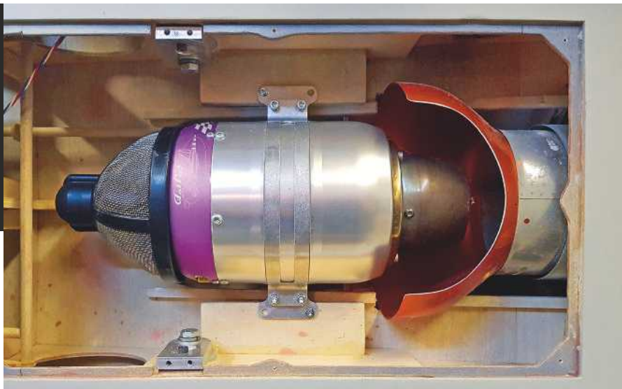
The JetCat P100 was fitted with a large thrust tube to help prevent heat build-up and recirculation of exhaust gases.
