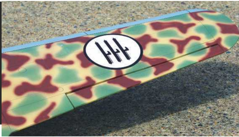
At 100" span this is not a small model. Note ailerons and the dummy flap line.
