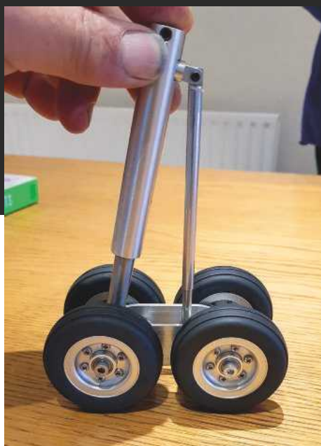
Main undercarriage leg fully assembled.
