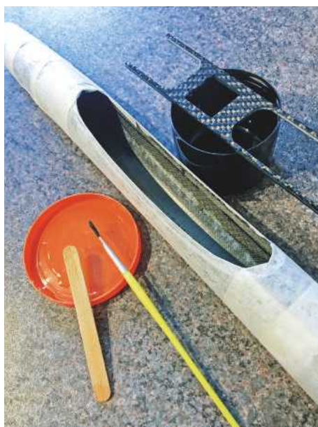
After wetting out the inside of the fuselage and the servo plate it was time to wait for the glue in the orange dish to reach that magic 'soft toffee' consistency.
