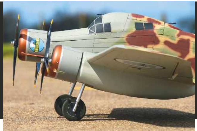
This side view shows off the varied thrust lines.
