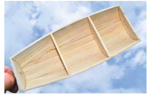
Planking isn't difficult but take time to ensure each strip accurately fits without any gaps.
