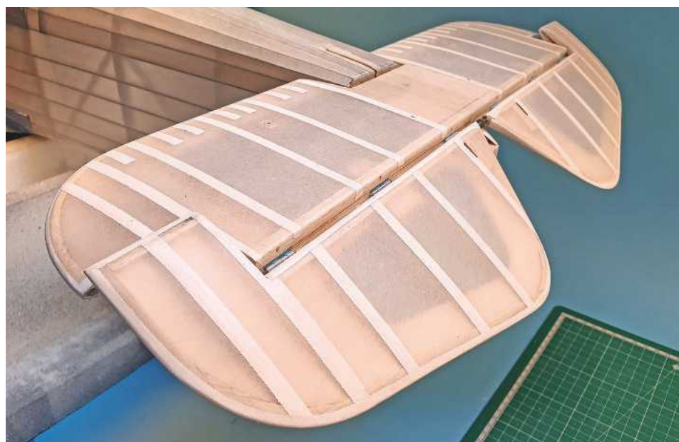
Left: Slow epoxy was used and nervously checked every 10 minutes!
