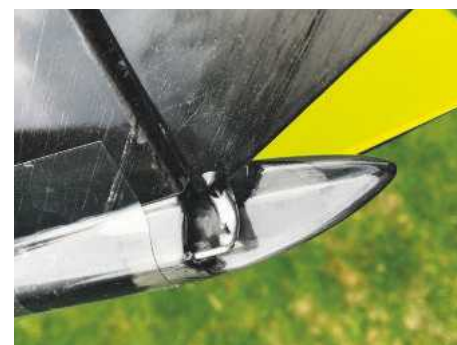
V-tail pushrods are a press fit - no keepers required.
