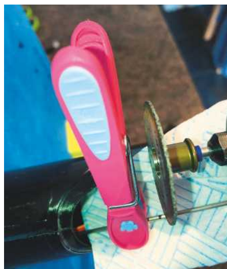
Parting off a pushrod to length. The peg lifts it just clear of the fuselage sides.
