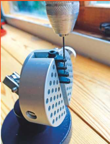
Above: Centre, tip and tail deflection guides are provided to set up the control throws. The centre one needs extending to cater for full flap - I taped on a small crescent cut from card. Left: My sole IDS horn of the correct length was used as a guide to drill out and cut down a set of longer horns. Holes were drilled undersize and then reamed out with fine pin files - no slop needed here!
