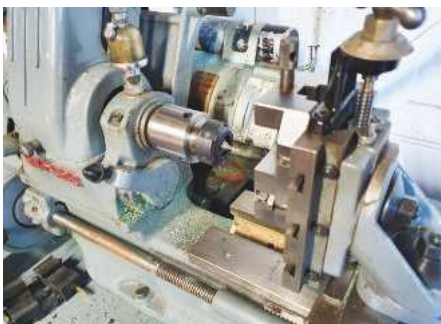
Myford ML7 with the vertical slide fitted. The collet replaces the normal chuck for rigidity.
