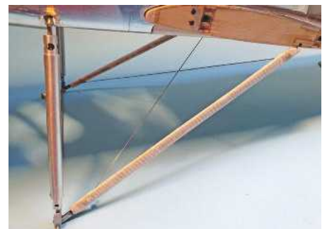
Undercarriage wire work assembled to check that it functions as expected.
