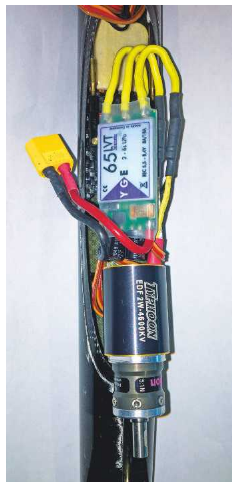
A dummy install of the motor and ESC, together with a LiPo (not connected), showed the forward position of the servo plate.
