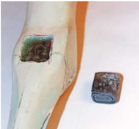
Nobody likes to add nose weight, but the short nose and head dictate its use in this case.
