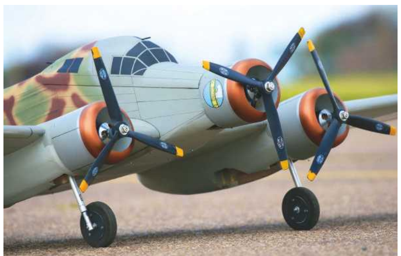
The electric powered SM.79 uses three 500kV outrunners.
