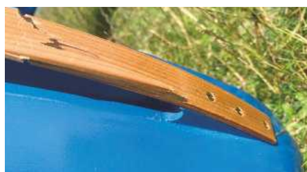
I landed out after the second flight, a broken skid being the only damage.
