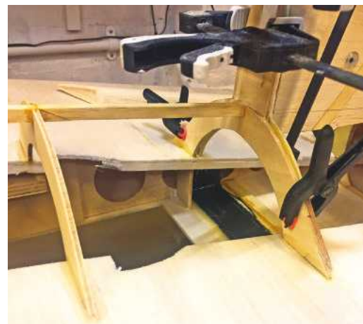
Tail reinforcements include additional glass fibre and ply formers that extend down inside the main frames.
