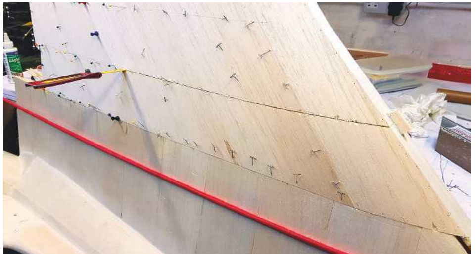
Be brave! Using a pad saw to separate the outer wing.
