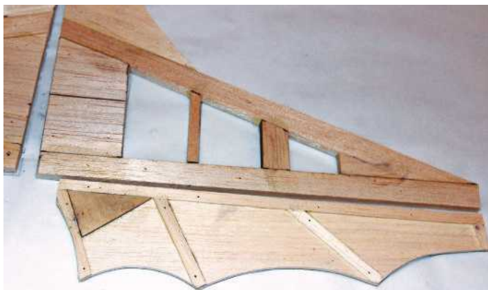
V-tail uses all balsa traditional construction.
