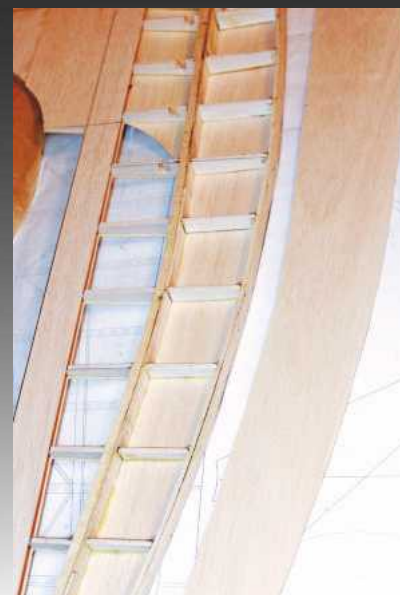
Wing sheeting cut to shape before being glued in place.
