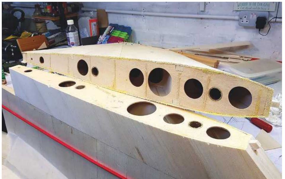
Wing parts after sawing in two.
