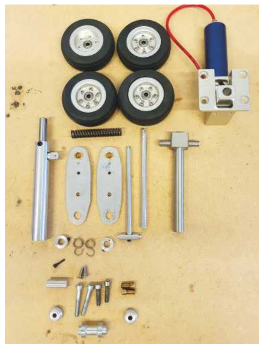
Parts for one set of main undercarriage leg, oleo and bogie.
