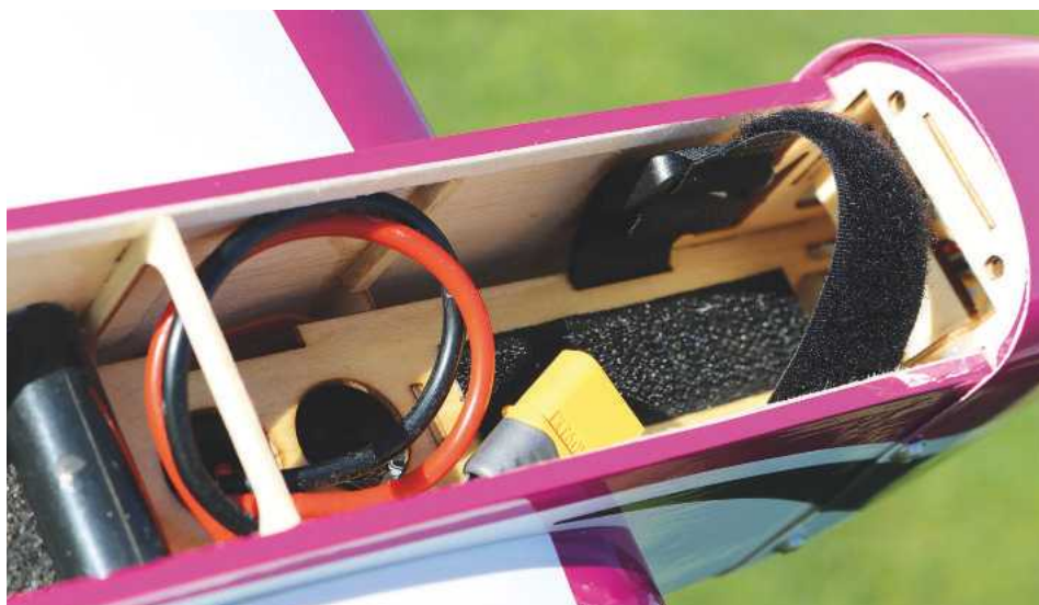
The battery bay. Anything in the 1300 - 2200mAh 3S range will fit, although I prefer the smaller, lighter packs.
