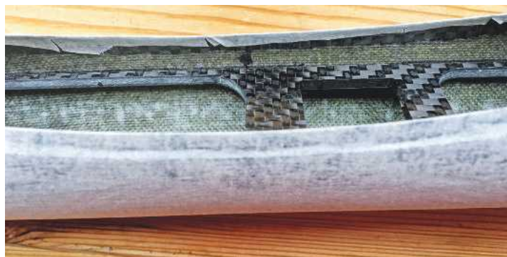
Fine marker lines, just visible, showed where I needed to place the servo plate when it was all glued up.
