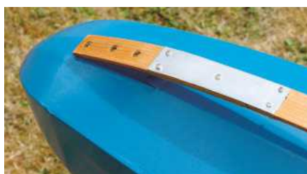
My skid repair job. Litho plate top and bottom did the trick to lend it that 'hangar workshop' aesthetic.
