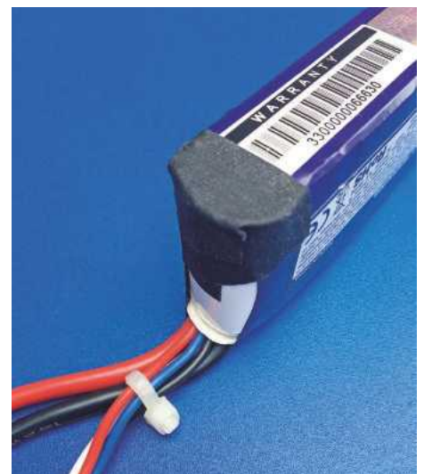
Tesa cloth 'guard' tape was used to prevent the LiPo packs from chaffing on the radio bay lip.
