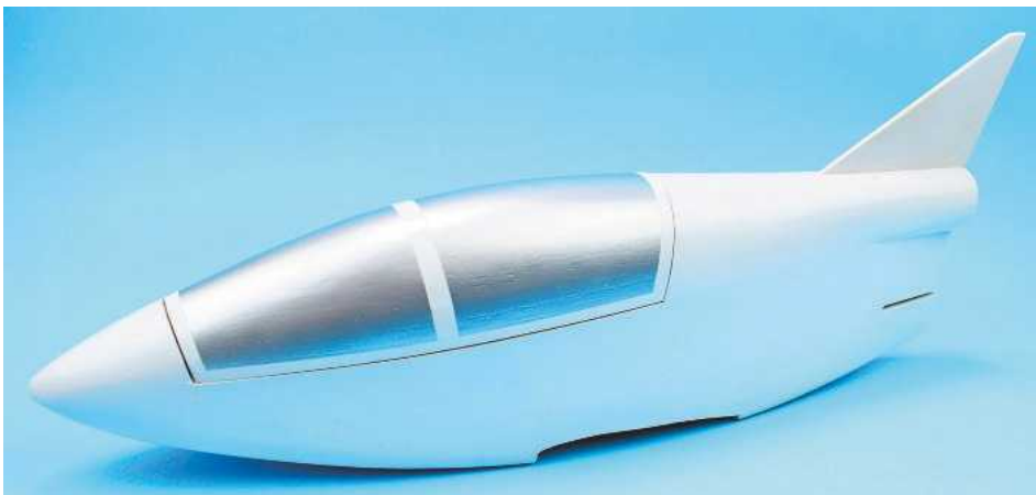
My model was simply finished in sanding sealer and rattle can paint. Don't forget to mark out the canopy lines when building the fuselage otherwise you will regret it later when trying to cut it free.
