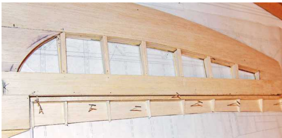
Aileron lower sheet shown fitted with riblets and curved to the rear edge.
