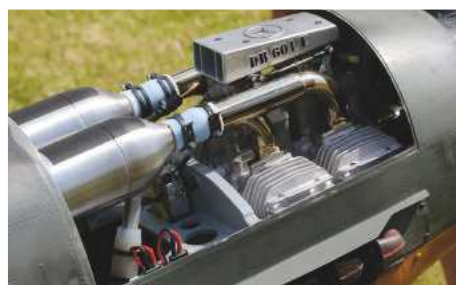
Andreas from Legendary Fighters showed me the impressive twin exhausts and his very clever close-fitting air-cooling ducting on his Me 109.
