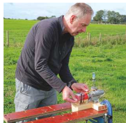
Running-in takes patience but is great fun. A simple throttle pushrod helps you change the revs.
