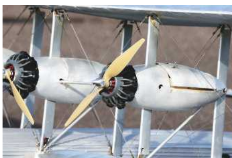
The engine nacelles are set very high. Martin home-moulded all 36 cylinders.
