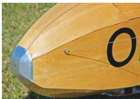
The front of the nose was built up with car body filler and covered in litho-plate.
