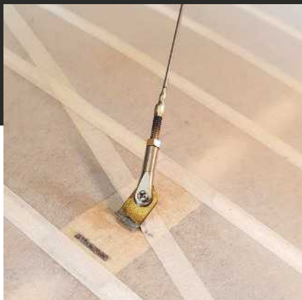
Mick Reeves rigging is a joy to use. The fittings are attached to the anchor point by a single screw. Loosen to remove.
