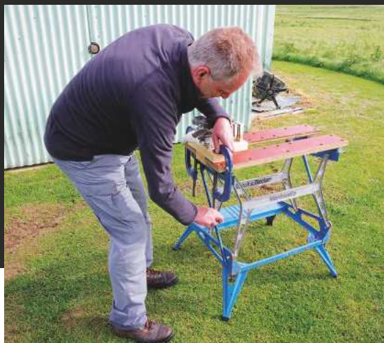
A Workmate (or clone) makes a good engine test stand.
