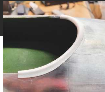
Vector Board after tucking inside and glued with 3M Super 77.
