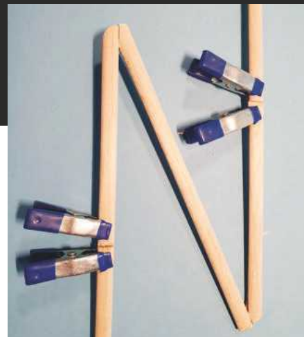
I cut the strut and added more material in an overlap.
