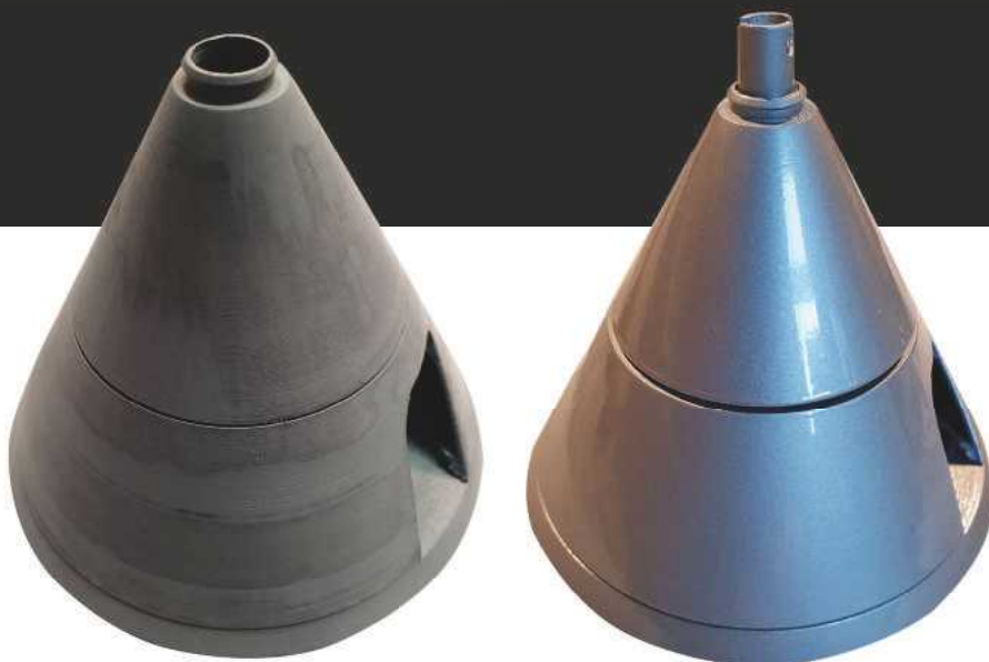
My 3D spinner after a rub down with wet and dry and a couple of coats of primer.
