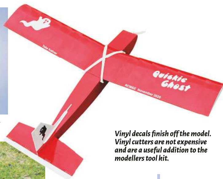
It genuinely flew off the board with no trim required. As I overpowered mine a tad it would possibly benefit from a degree or two of down thrust.
