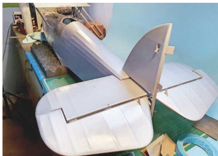
Fuselage in silver. The elevator is covered in nylon with torn Solartex tapes.
