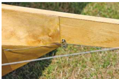
Control runs pass over neatly formed pulleys.
