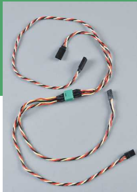
Wing wiring harness connected to its matching fuselage wires. The green connectors will need bonding to the fuselage sides and the wing roots.
