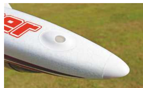
Hard plastic helps protect the sharp end.
