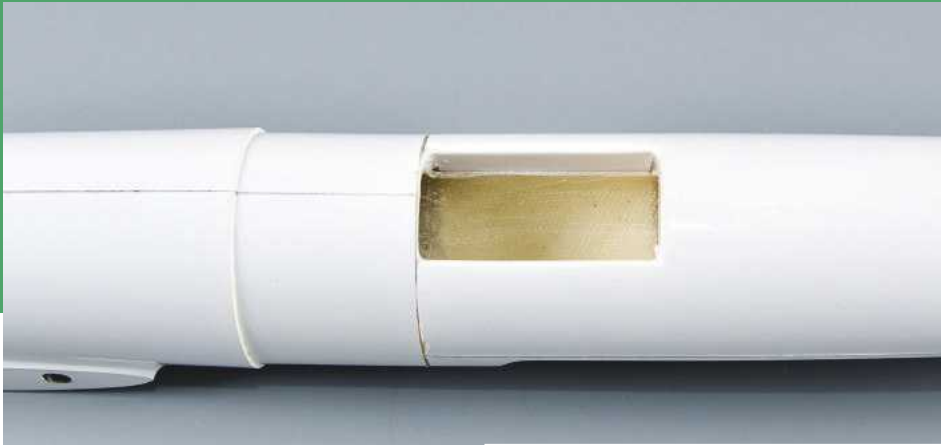
Above: Ballast tube access hole is covered by the nose sheath in flight.
