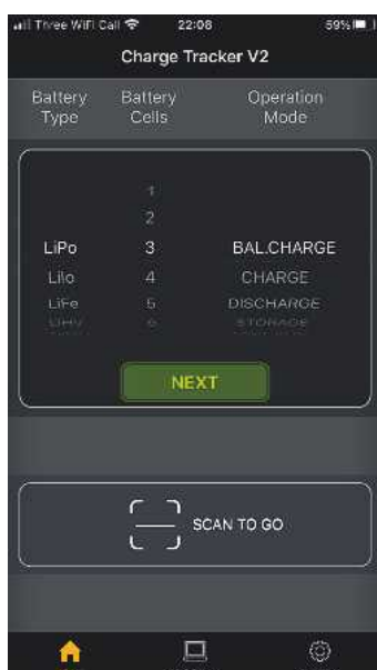
Charge Tracker app is free to download and very easy to use. Use the Home screen to select Battery Type, Number of Cells and Operation Mode.
