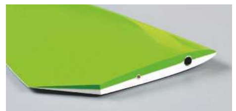
The tail jointer rod needs sanding down to be an interference fit within the larger tailplane pivot tube.
