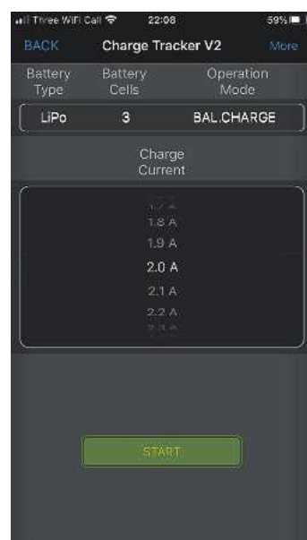
The Next screen confirms the battery set up and allows you to change the Charge Current. Press Start to begin charging.
