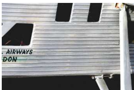
Fuselage corrugations were achieved using Martin's innovative balsa strip and Balsaloc iron-on process.
