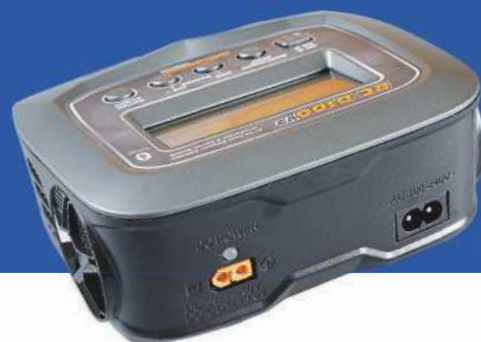
Rear view showing the AC input and DC input/output via an XT-60 connector.
