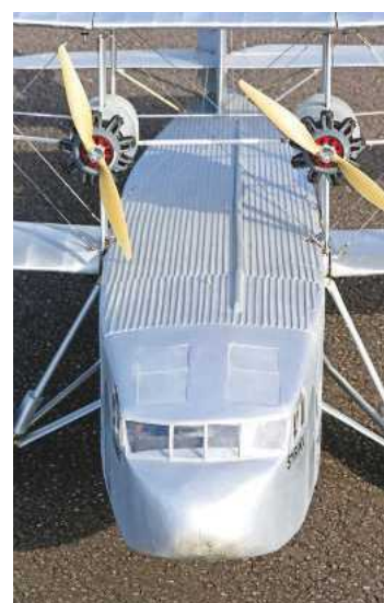
The original was an all-metal airframe employing corrugated alloy sheeting.
