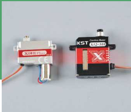
Distinctive 'open motor' KST Xo8H Plus servos are supplied for the ailerons and flaps, whilst a pair of KST X12-508s operate the tail surfaces.
