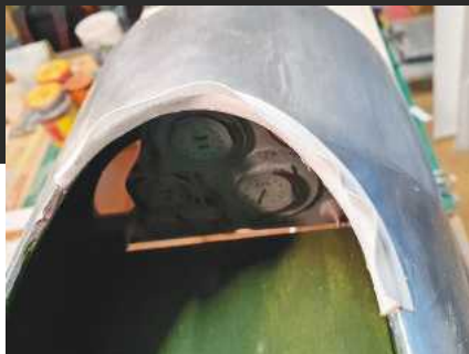
1 mm Vector Board glued to the cockpit surround, then covered with 0.5 mm board, wrapped over and inside.
