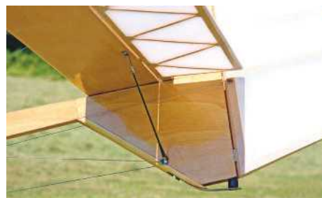
Tailplane bracing and protective tail skid in detail.
