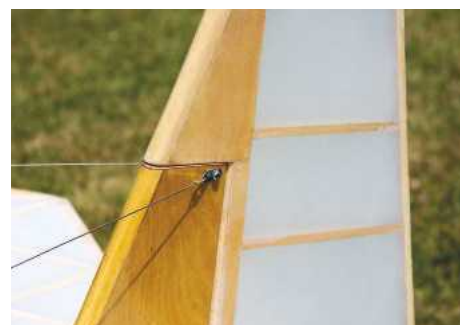
Rigging wires extend from the fin to each wing panel.
