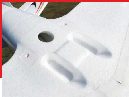
Finger holds on the underside mean solo launches should be straightforward. That's a cheater hole, just aft.
