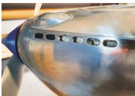
After removing the cutting template, I was left with raw holes. Not very satisfactory...
