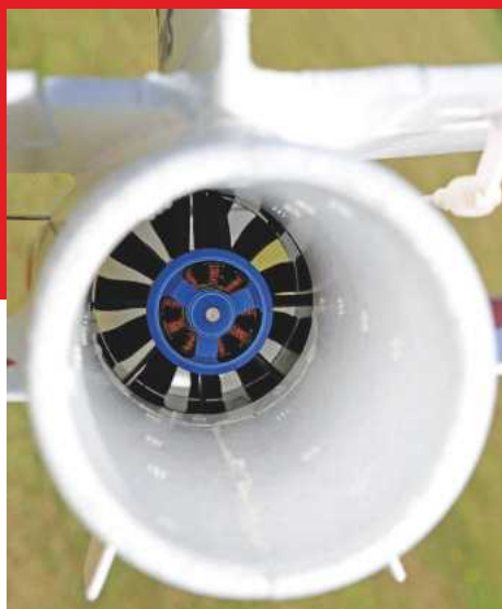
The 4500kV brushless outrunner and 11 blade fan are surprisingly quiet.
