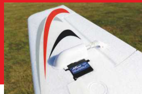
Protective covers over the servo arms are another nice touch.
