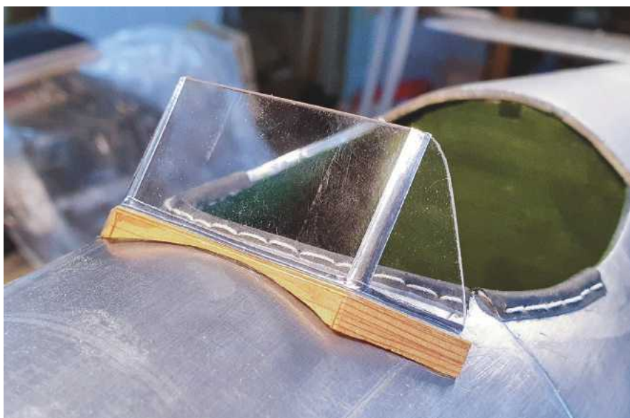
To finish the cockpit off a windscreen was made from a chunk of PETG, folded cold and with a hardwood base.
