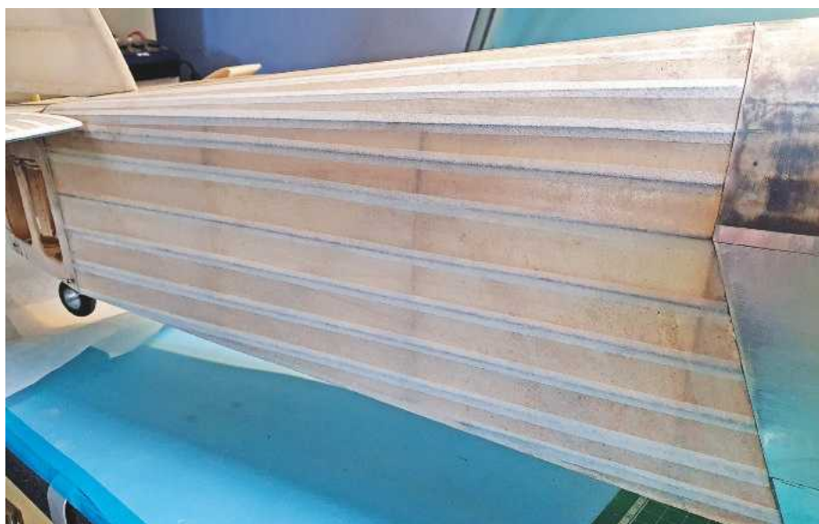
I used a lightweight tissue to simulate the rib taping on the fuselage. It does show through but is a bit feint through the silver.
