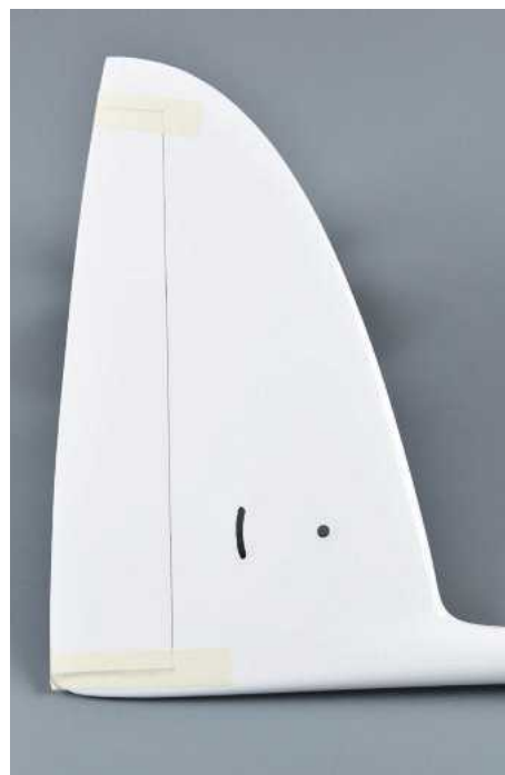
Neatly moulded tail fin showing the pivot hole and rear movement arc of the ready fitted AMT bell-crank.
