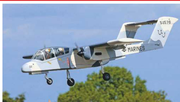
Above: David Osborne's 1/5th scale electric Bronco. Twin Axi 2328 out-runners driving 17" x 12" props.
