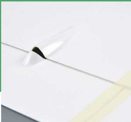
Small bulges on the top surfaces of the ailerons, flaps and trailing edges help smooth the airflow over the pushrods and control horns.
