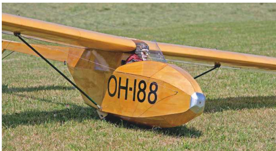
Fuselage pod showing the ply skins that were ironed onto the underlying framework.
