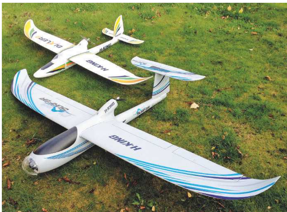
Foam pusher models make ideal FPV conversions. Some, like the one in the foreground, come camera ready.
