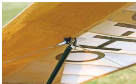
Focus on the scale wing rigging and strut attachment points.
