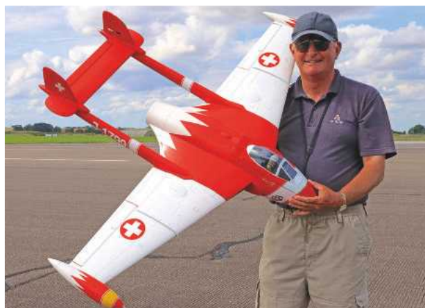
Alistair Foot and his 1.5m span EDF foamie DH Venom. Weighs 2.9 kgs.
