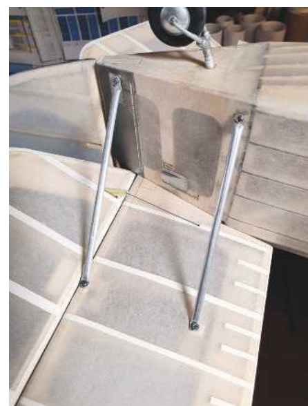
K&S Tubing, slightly flattened, serves to re-create the tailplane underside rigging.
