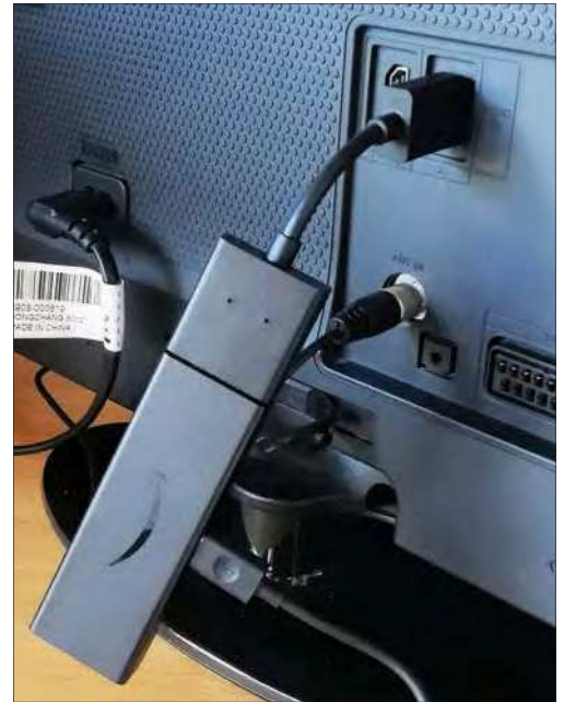
Amazon's Fire TV Stick HD dongle in situ, fitted with an HDMI extension. The 5V power cord hangs separately; you could try powering it from a spare TV USB port.
