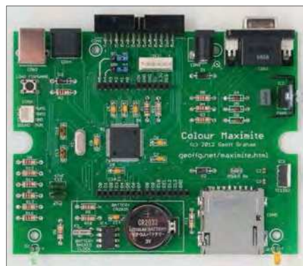
Fig.13. (left) Colour Maximite 1 (CMM): The original PIC-based Colour Maximite computer, as featured in PE (November 2019 – February 2020). £68.95
