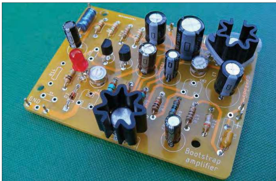
Fig.12. Completed silicon amplifier. Note how bias transistor TR3 is tied to the heatsink of output transistor TR4, providing a degree of thermal stabilisation of the quiescent current.
