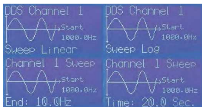
Screen 5: you can disable sweeping, or have a linear or log (exponential) sweep. If enabled, you set the end frequency and sweep time in the next couple of screens (the start frequency is the channel's set frequency). It can sweep up or down.
