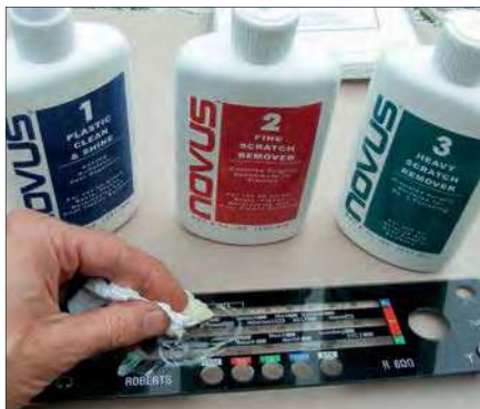
Fig.6. Scratch remover kit for plastic dials – a lot of rubbing is involved.
