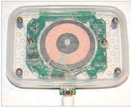
Fig.2. The charging module mounted to the underside of a lid taken from a translucent kitchen storage container.
