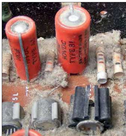
Fig.9. The dust build-up in old gear can be horrendous, and a fire hazard.
