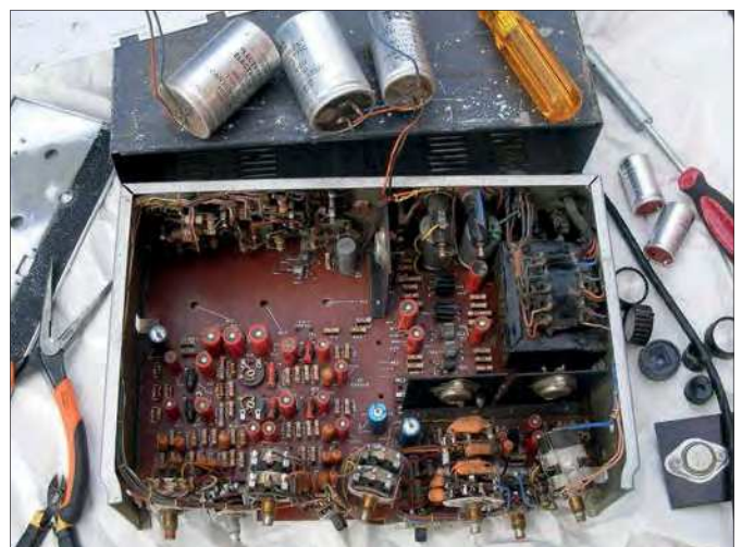
Fig.8. The eBay Stereo 30 pulled apart. Sometimes equipment is so dirty it's the only way to clean things up to get to the components.
