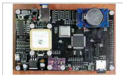
Fig.11. Extreme 100 (MMX100): MMX. Onboard GPS and gyroscope/compass headers make this a useful development platform. £80.00
