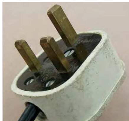
Fig.15. Unsleeved pins on a 1960s MK mains plug; it's built like a tank and good for another 50 years.
