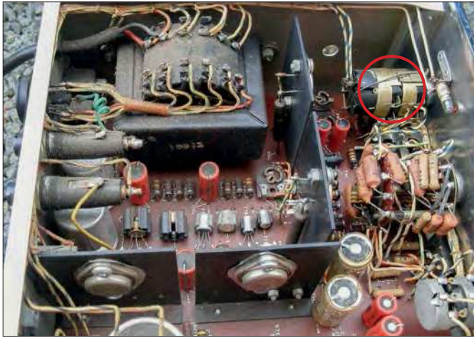
(Left) Fig.13. The mains on-off switch was often ganged with the volume control on old audio gear. I don't think it's a good idea, but it does mute the turn on/off thumps from the pre-amp. (Right) Fig.14. The fuse holder is now safe (too late in my case) with its (pink) sleeve, also on the mains switch.
