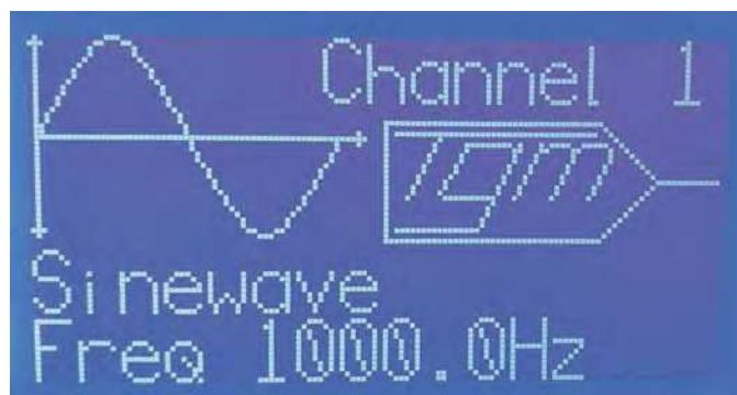
Screen 1: this screen lets you set the output frequency of the currently selected channel.
