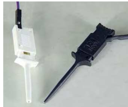
The genuine E-Z-Hook test clips, shown at right, are much easier to use and more reliable than the cheap test hooks I initially purchased, at left. I eventually found a much better-looking set of low-cost test clips at Banggood (see text).
