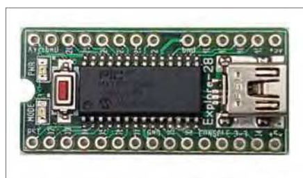
Fig.2. Explore 28 Module (E28): MM. An SMD version of the MKC and Development Module, all on one compact PCB. £17.50
