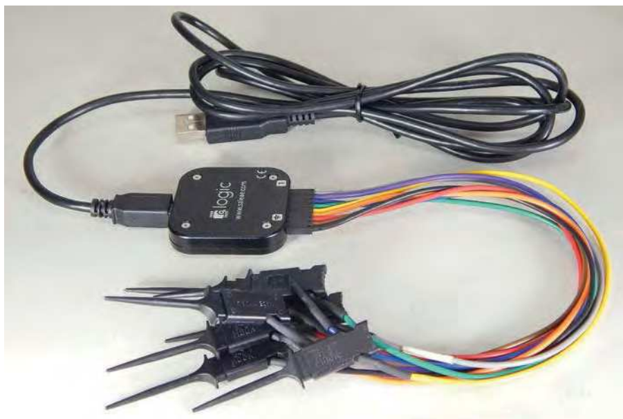
For comparison, here's the original Saleae Logic, purchased a few years ago, along with the supplied (functional!) USB cable and high-quality test clips.
