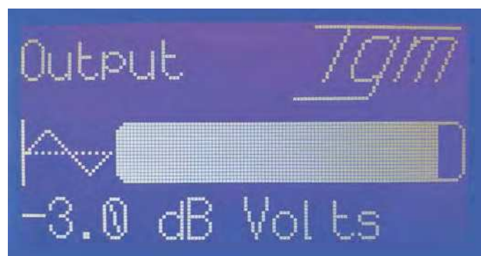
Screen 3: the next screen lets you set the output level from -123dBV (0.7mV RMS) to +5dBV (1.78V RMS) in 0.1dBV steps.
