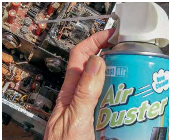
Fig.10. The difficult to reach bits can be blown with an air duster.
