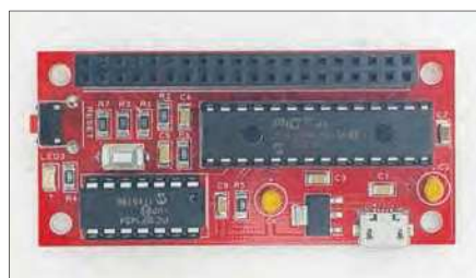
Fig.5. Pi-croMite (MM-PHAT): MM. An E28 that fits inside a RPi-Zero case. RPi PHAT modules plug into the 40-way GPIO connector. £28.95
