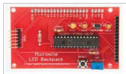
Fig.3. Backpack v1 (BPv1): MM. A 2.8-inch touchscreen plugs directly into this module – as used in several PE projects. £19.95
