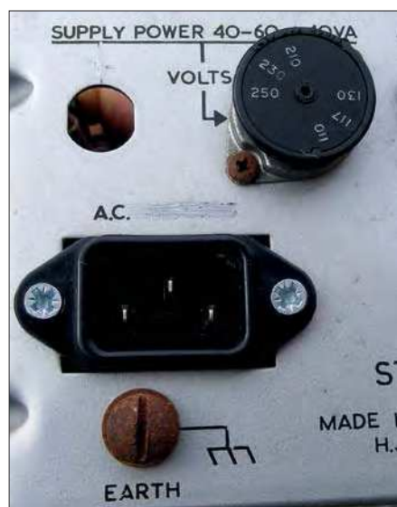
Fig.11. Old equipment often has rotary mains voltage selectors since there were wide local variations in mains voltages at the time. Use the 250V setting in the UK to minimise stress on old parts.
