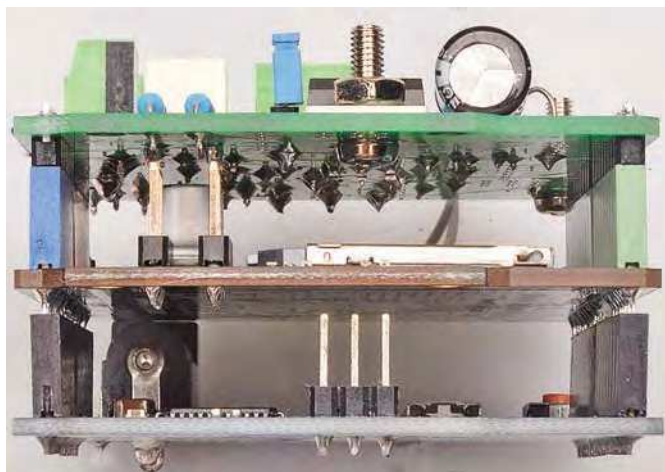
With stackable headers, the three shields (PCBs) simply connect together via their header pins and sockets, as shown here.
