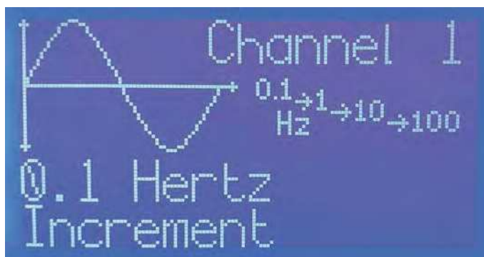
Screen 2: here, you can change the size of the frequency steps in the previous screen.
