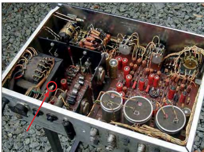
Fig.12. Old gear often has lots of exposed mains wiring. The rear terminal on the fuse holder (far rear left) bit me!
