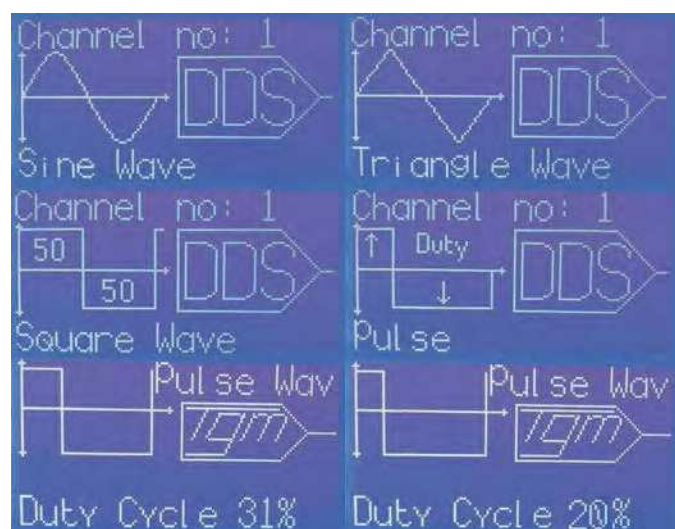
Screen 4: as you rotate the knob on the waveform selection screen, you can select Sine, Triangle, Square or Pulse. For Pulse, you can set the duty cycle from 1% to 99%.
