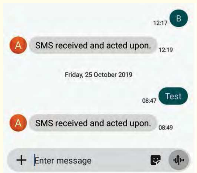
Fig.9: as the 4G Remote Monitoring Station is only powered up infrequently, it may not respond to an SMS command immediately. The two-minute delay shown here occurred during testing, when we had the Interface Shield set to power down for about one minute at a time. The canned response can be changed by editing the Arduino code.
