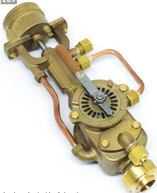
Brake valve made using Adam Cro's castings.
