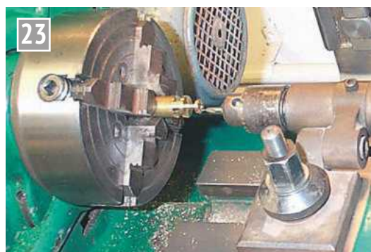
Making a lantern pinion.
