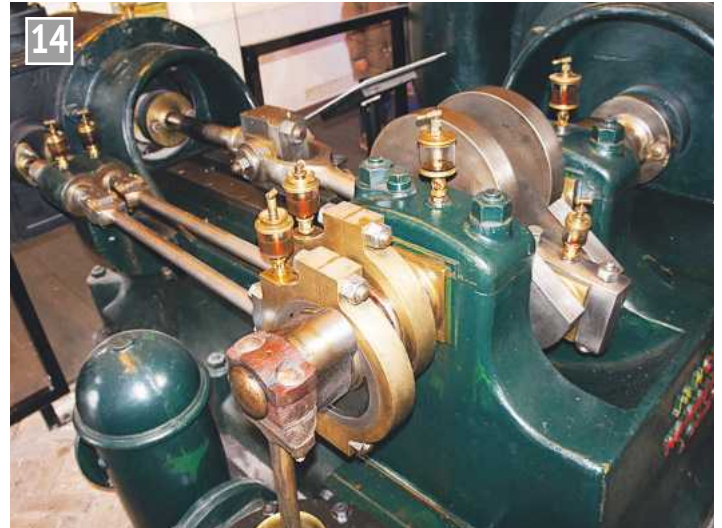
Detail of the J. & H. Gwynne engine. It had adjustable Meyer slide valves and operated until 1959.
