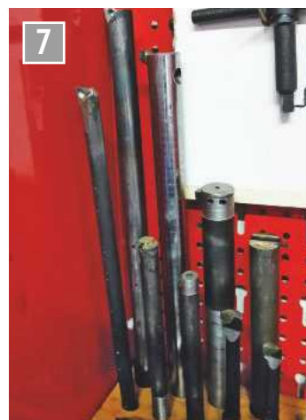
Silver soldered insert tips.
