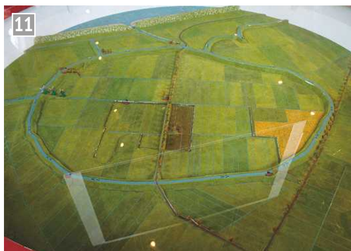
How a polder worked. The Harlemmermeer was drained like this, though on a larger scale. Pumped by a chain of windpumps (left) to a ring canal, water flows to the sea (top). Drainage ditches were then dug across the polder and farms built. (Unfortunately, it's not possible to avoid light reflection when photographing this informative model.)
