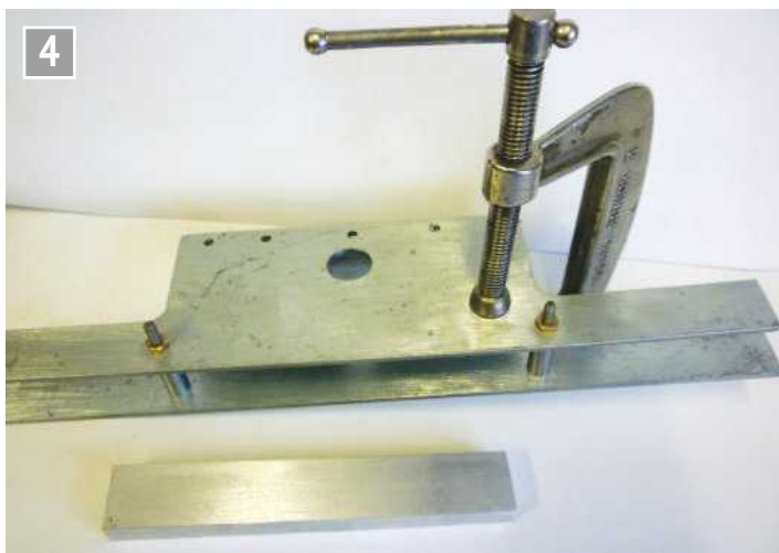
Spotting through the frame plates.
