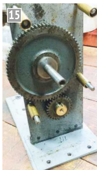
The gearbox with endplate removed to show gears.
