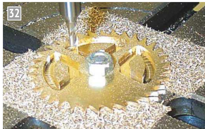
Crossing out the escape wheel on double-sided tape.
