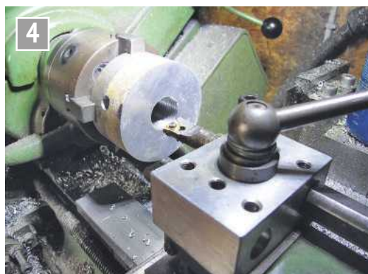
Screw cut 1 1/8 inch Whitworth thread.
