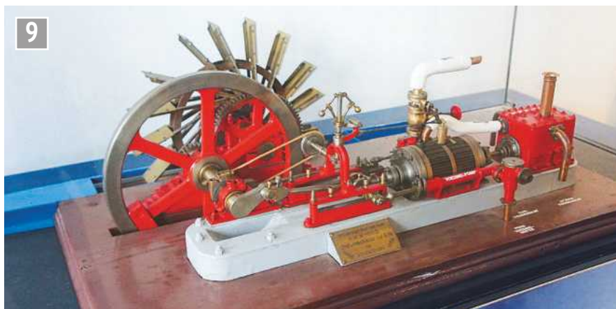
Model of a steam engine with scoop wheel, one of several fine models in the Cruquius Museum. This was built by Mr. A. M. W. Hoos in the 1880s.
