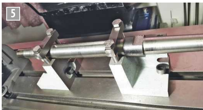
V-block set-up for mandrel slot milling.
