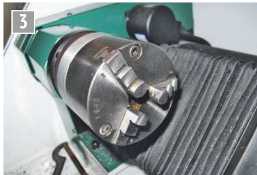
New three jaw mounted to the adaptor.
