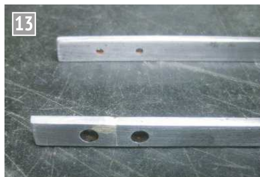
Motion bracket after repair.
