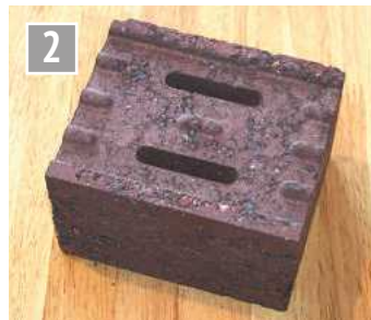
A thermal storage brick (photo courtesy of Barry Gray, Gillingham).
