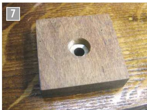
Locating spacer for the base.
