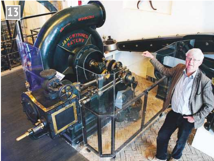
Constructed by J. & H. Gwynne of Hammersmith around 1879, this engine and centrifugal pump was considered high speed when it was built. Adrian Strik stands alongside. He is a member of the 'Steam Team' and gave a fascinating tour of Cruquius.
