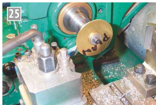
Wheel blanks were turned using a 2MT mandrel, made up for the purpose.
