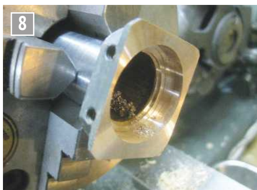
Machining a recess in the base of the column.
