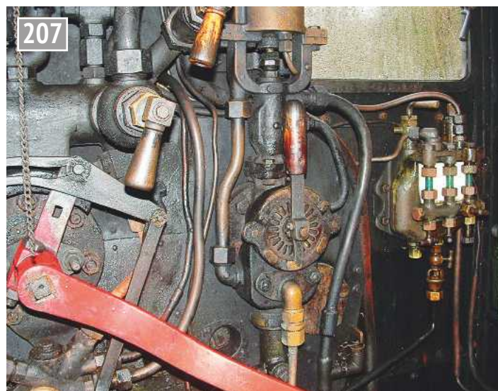
A view of the brake valve.
