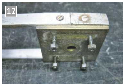
Original state of the motion bracket.
