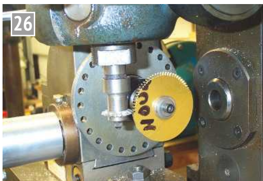
The 2MT mandrel was then transferred to the dividing head on the miller for tooth cutting.
