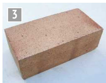
A structural firebrick.
