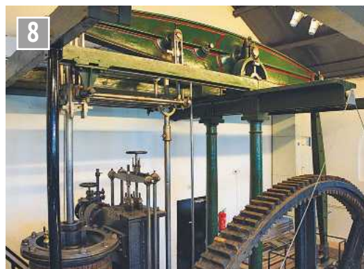
Early steam power used for drainage at Arkelse Dam. Built by John Cockerill of Belgium, it has Watt's parallel motion and Meyer slide valves. It once powered a scoop wheel of 7.5 metres diameter.
