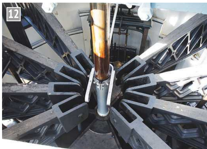
Cruquius engine - an interior view showing the beams powered by an annular compound engine beneath the great cap. The annular compound has the high pressure cylinder within the low pressure.
