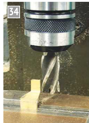
Shaping the front cock, after silver soldering.
