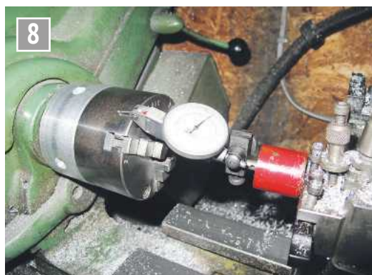
Checking for run out.
