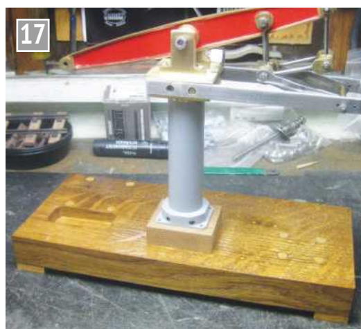
Restored beam and motion bracket assembly.
