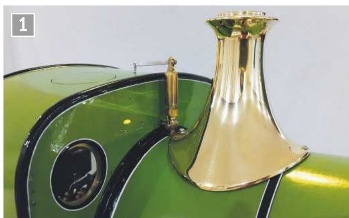
Safety valve cover made from an appliance motor and a candle stick.
