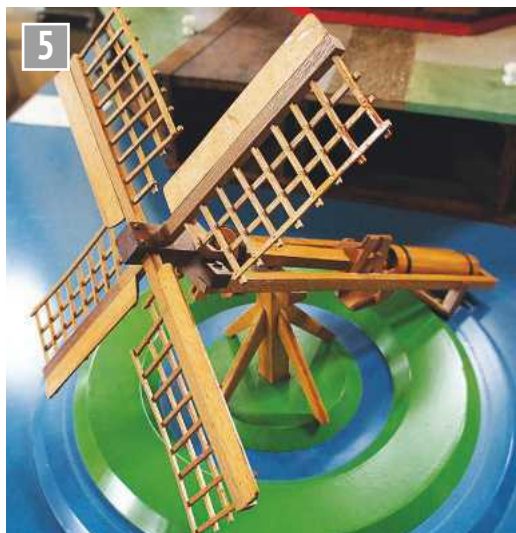
Model of a small tjakker mill. These drained fields into higher level ditches using Archimedean screws.
