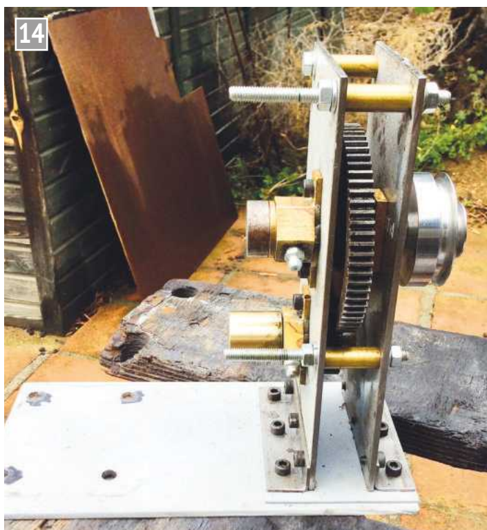
The gearbox with belt drive pulley on the right.
