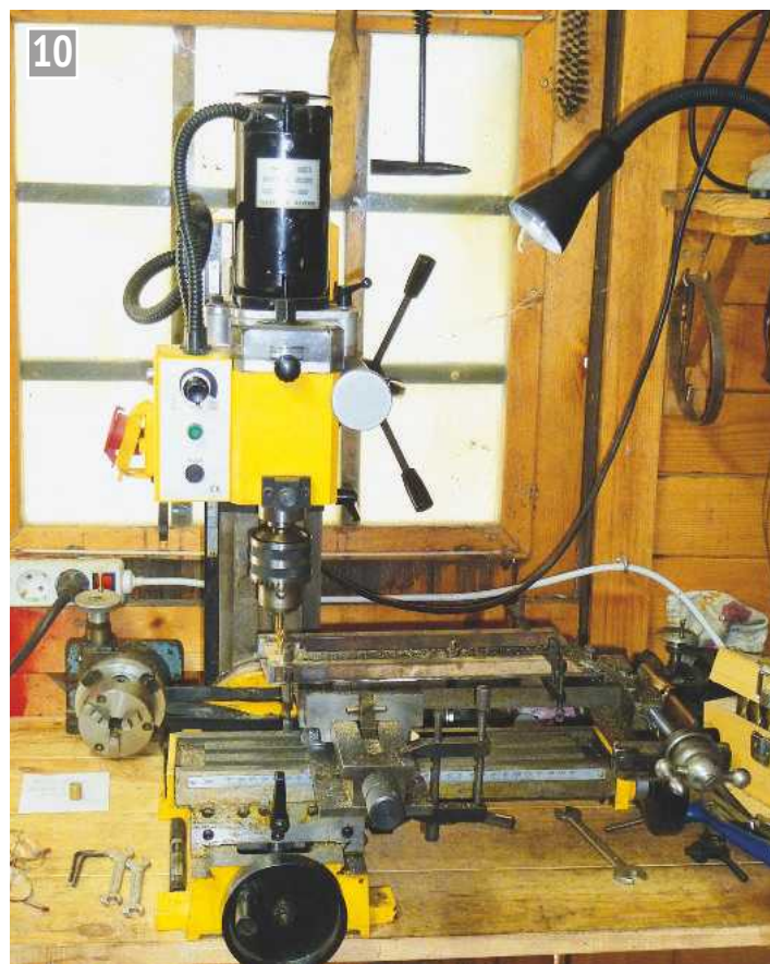
Mini-mill with belt drive conversion.
