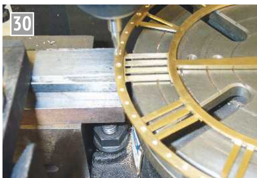
Applying the 5-minute and 1-minute markers.
