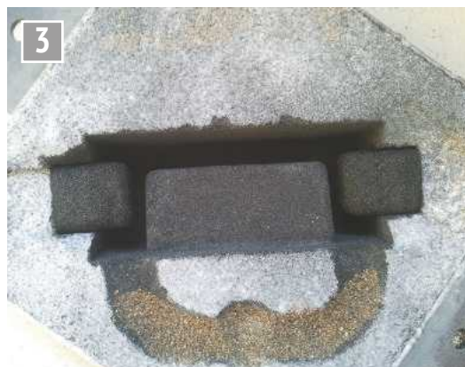
Angle 'V'-Block mould.
