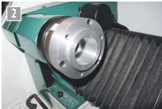
Adaptor mounted to Novaturn spindle.
