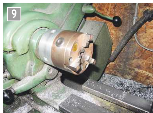
Second chuck mounted on the adaptor.
