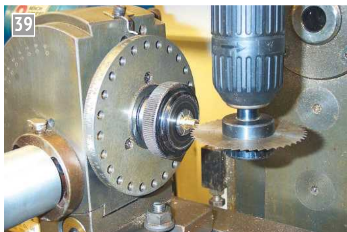
Using a fine slitting saw on a hand collet.
