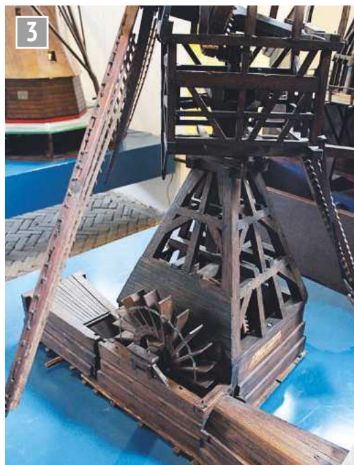
Wooden model of a post mill with scoop wheel. With their cloth sails, these dominated land drainage.
