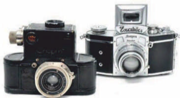
Early 35mm SLRs: the second model of the Kine Exakta (rear) and the now rare Russian Sport
