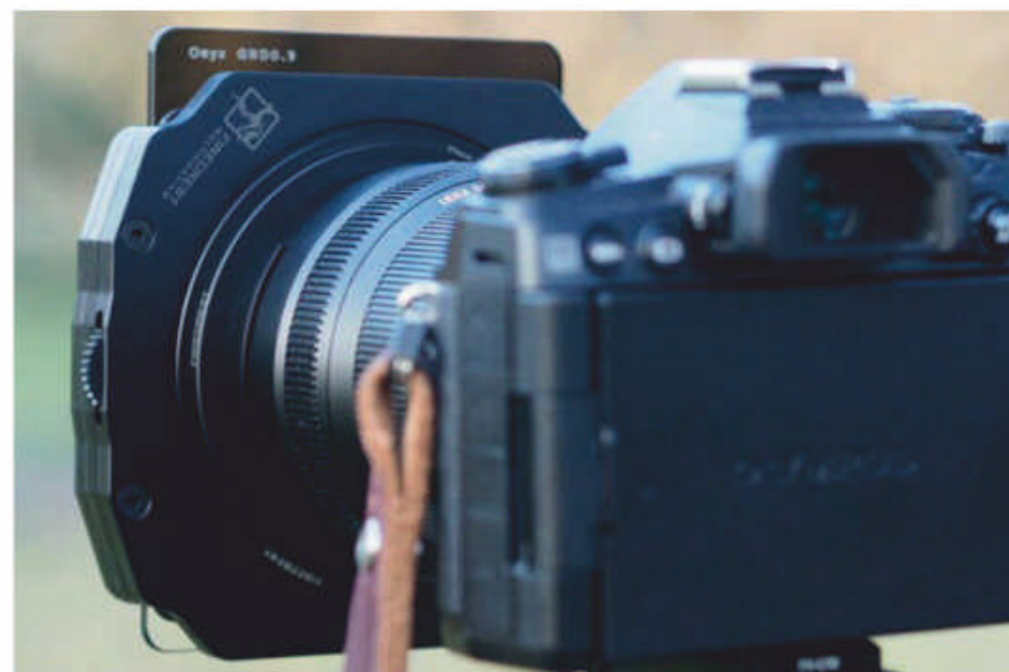
A wheel set into the holder is used to adjust the polariser's angle
