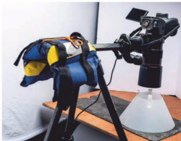
Ankle weight used to steady a lightweight tripod when shooting a look-down close-up
