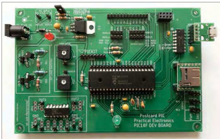
Fig.15. At last! – we have a built PIC Development Board . It's not yet fully tested, but so far it looks very promising.
