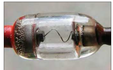
Fig.13. An old germanium point-contact diode. Note the slab of germanium and the spring-loaded point-contact wire.
