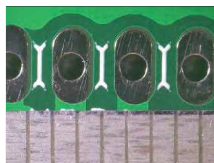
Fig.14. Solder resist layer (mis)alignment.
