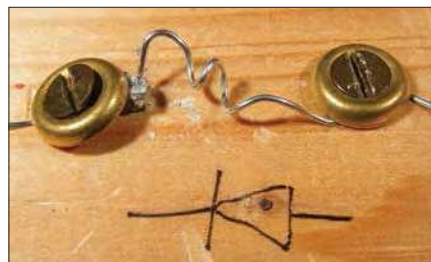
Fig.12. A detector using a galena crystal based on the Ladybird book design. Note the springy pointed wire, sometimes known as a 'cat's whisker'.
