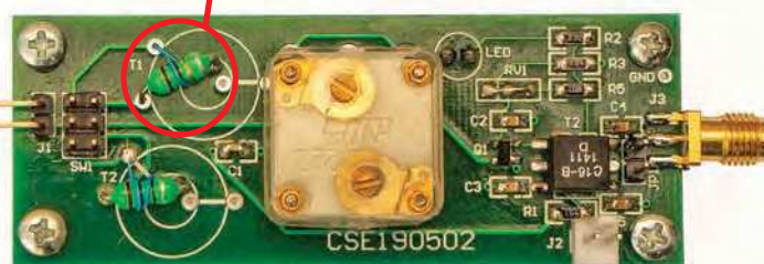
Fig.2a (top) is the component overlay for version 1, using two toroids for T1 and T2 with primaries and secondaries wound through them. Fig.2b (bottom) shows version 2, an identical overlay but using axial RF chokes instead, with primaries of one or two turns of thin wire around them.
