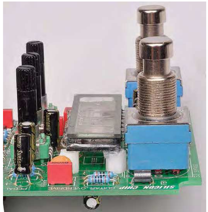
The 6P1 valve mounts on four 6.3mm nylon standoffs, as shown in these photos. This helps minimise microphonics which could otherwise be a problem.
