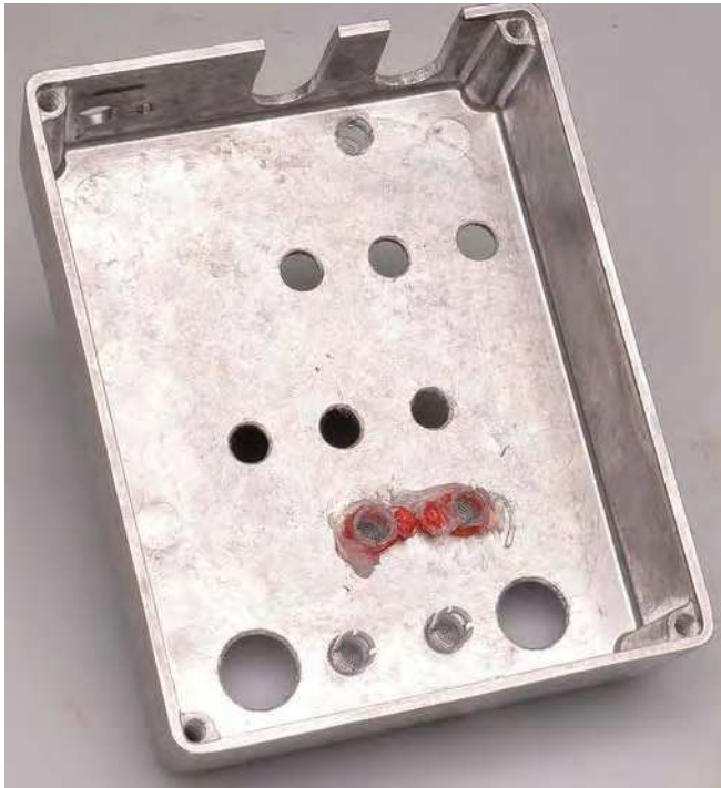
14 holes and two slots are drilled/cut in the diecast case. Note these holes are in the bottom and end of the case. (See dimensioned drilling diagram on page 36).
