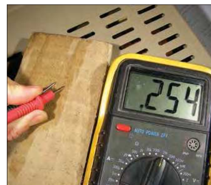
Fig.5. Tanalised wood can be conductive – do not use it in this project.
