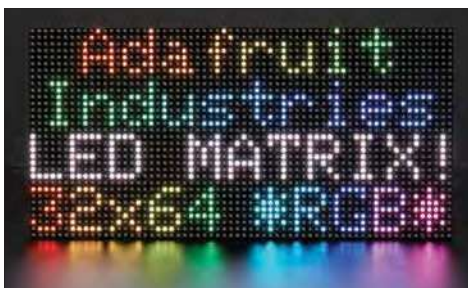
Fig.1. A typical 64x32 RGB LED matrix panel (LR): a) front, b) rear, c) connection to it is via a 2x8 connector (ribbon cable) with the pinout as shown.
