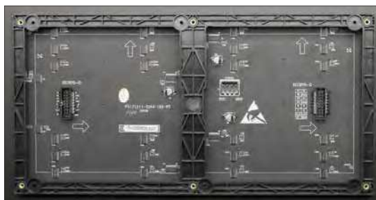
Fig.1. A typical 64x32 RGB LED matrix panel (LR): a) front, b) rear, c) connection to it is via a 2x8 connector (ribbon cable) with the pinout as shown.
