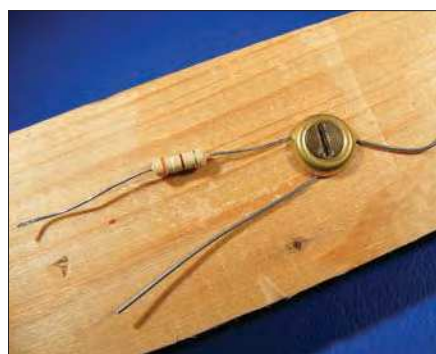
Fig.4. George Dobbs' screw-and-cup connection technique.
