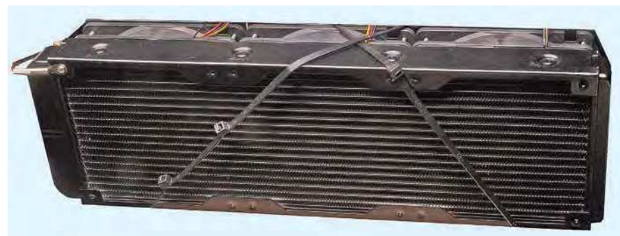
This radiator is more effective at removing heat than the heatsink and fans. This is due to its larger effective surface area.
