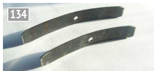
ABOVE: Two of the curved leaves ready for the two-part process of hardening and tempering. RIGHT: The revised spring assembly with its new leaves that provided the increased stiffness required.
