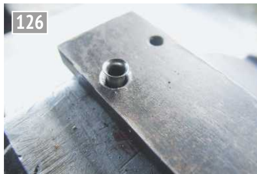
126 This view shows the forming block being used to add the flare to the top end of the vent pipe. The swaging operation has to be carried out while the pipe is straight otherwise the block cannot be removed.
