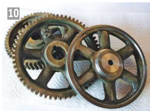
My flywheel is a repurposed gear wheel.
