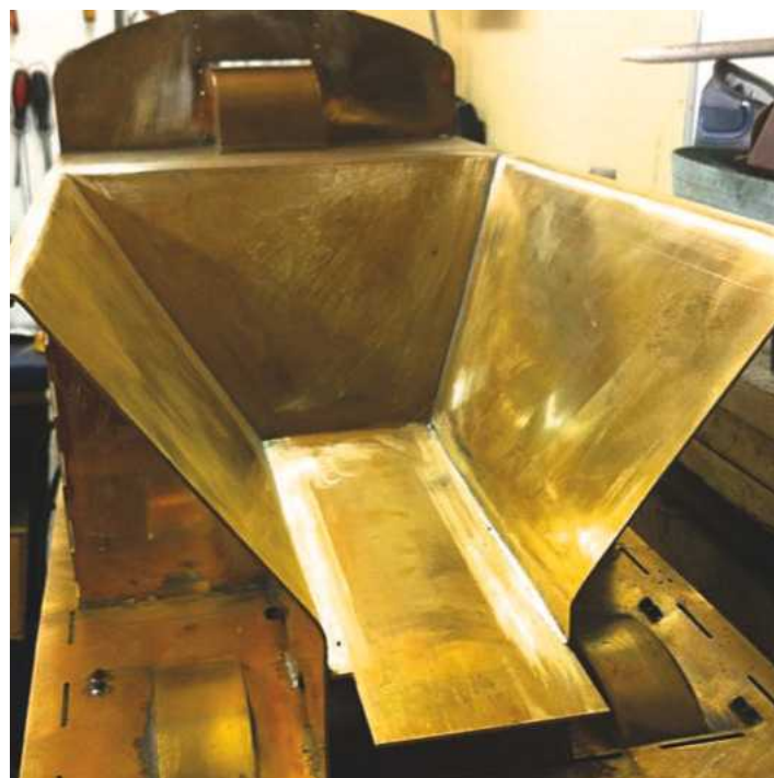
The next important step, which I include as an 'internal' part, is the fitting of the coal chute. In this picture the section has been folded to shape and soldered in place.
