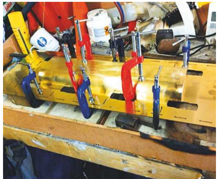
Belly tank held in place ready for brazing to soleplate. Brazing is the right word here as I was going to silver solder these parts together. Bad move - and I reverted to using soft solder in the end.
