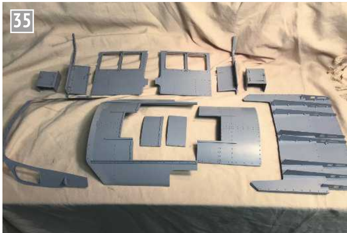
Cab sub-components assembled and primed, ready for joining.
