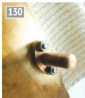
The adaptor has been fitted to the well tank ready for installation into the chassis to judge the angle of the pipe drilling.
