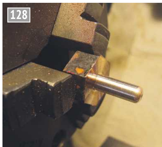
128 Odds and ends from the scrap box were used to make the pipe adaptor for the forward well tank; here the two parts were hard soldered together ready for machining.
