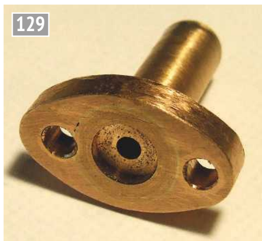
129 The pipe adaptor for the forward well tank connection. For convenience the joint onto the tank is made with a small 'O' ring rather than a conventional gasket.
