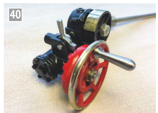
Reverser gearbox finished, with latch set back in a non-prototypical position, and oversized handle.
