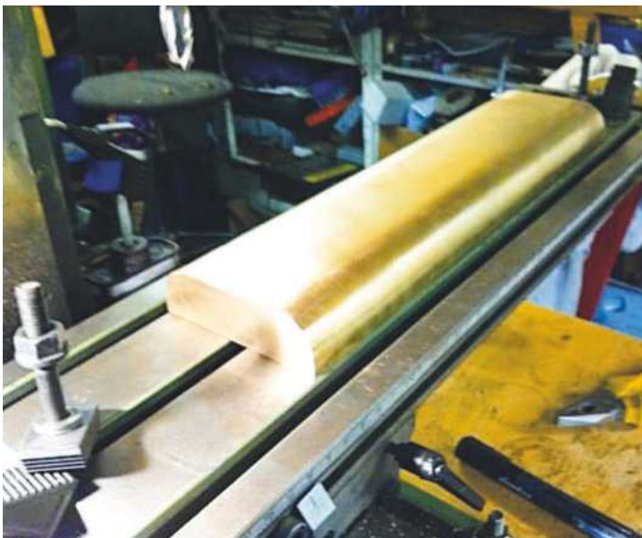
The finished belly tank being checked for the top edge being flat ready for brazing to the soleplate.
