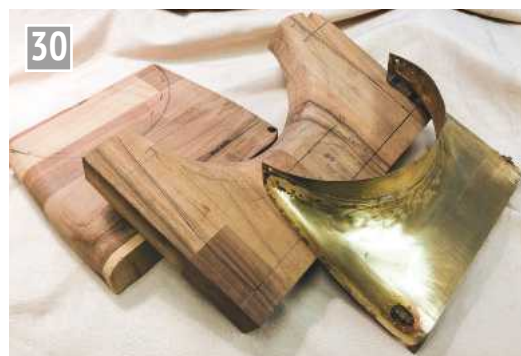
30 The lower part of the throat plate cleading formed from brass sheet using two wooden formers.
