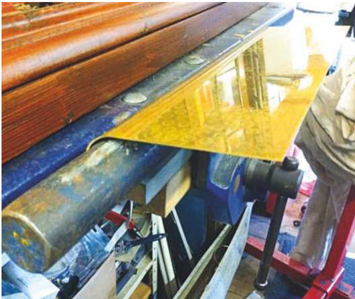
I have no rollers so had to use some steel bar to shape the tank. Some panel beating hammers helped with this.
