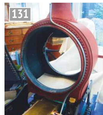
The final soldered assembly and the pipe in place on the locomotive chassis. Note that the engine has been dismantled to add the forgotten extras and undertake some painting.
