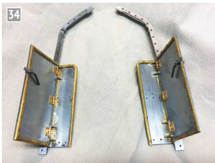
Cab doors being attached to frames and half-round brass beading affixed.
