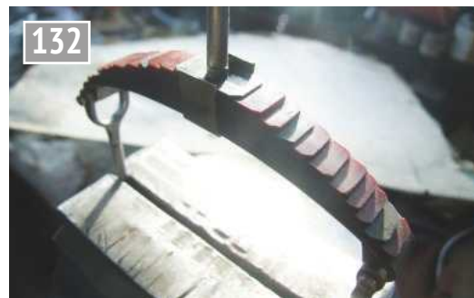
A front inside leaf spring assembly held upside down to show the method of clamping the leaves.
