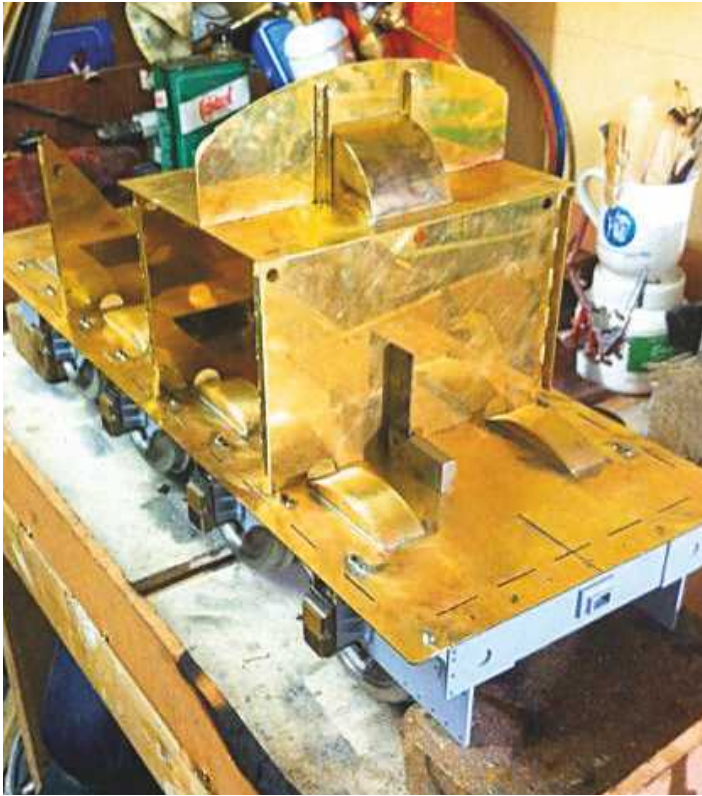
Rear coal wall with right angle supports riveted in place. The right angle sections are \frac{1}{4} \times \frac{1}{4} \times \frac{1}{16} inch.
