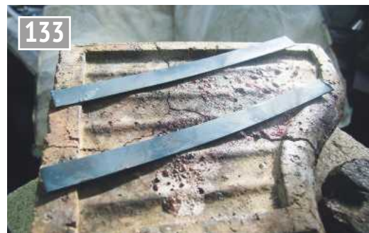
The two annealed strips of steel ready to be cut, drilled and shaped for heat treatment.
