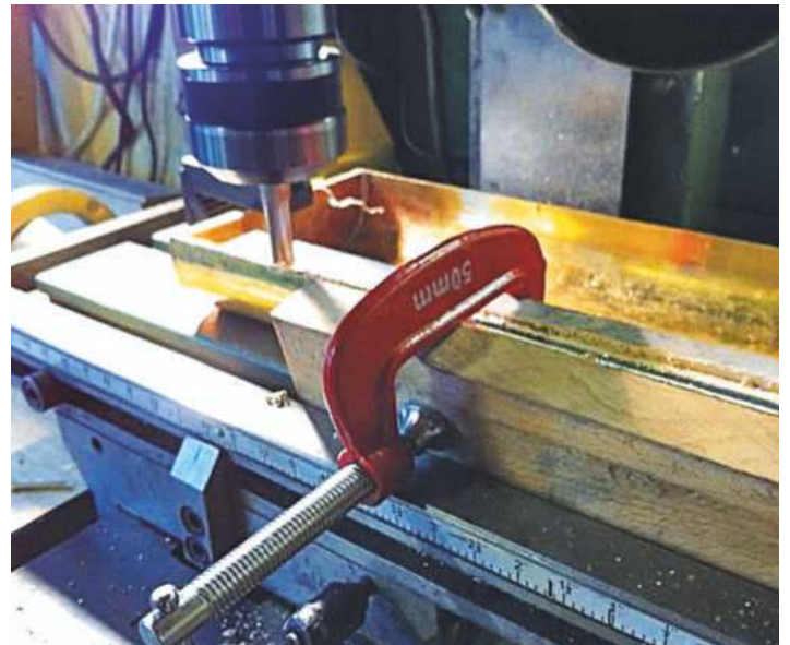
After the parts had been brazed (silver soldered) together the tank was clamped securely to the mill bed and the rolled sides were machined down to match ends.
