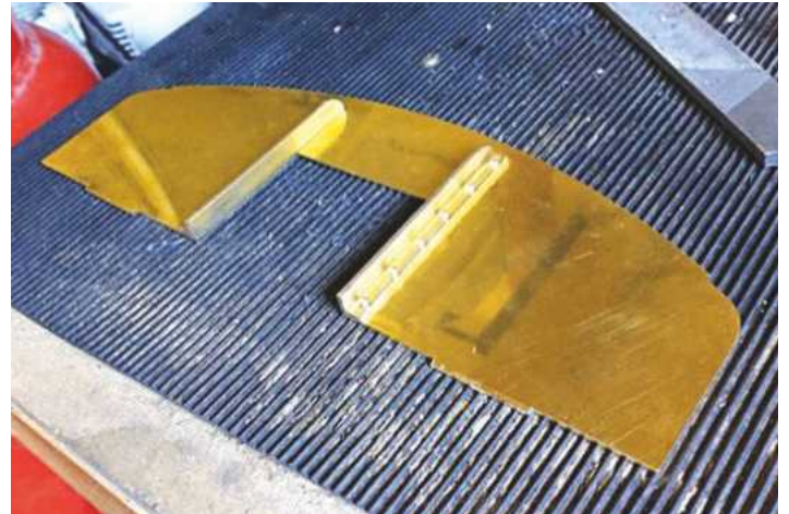
Rear coal wall with right angle supports riveted in place. The right angle sections are \frac{1}{4} \times \frac{1}{4} \times \frac{1}{16} inch.
