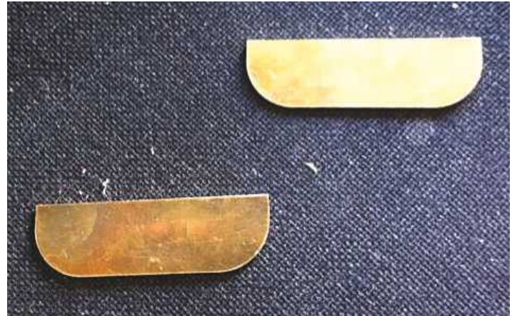
I started with the belly tank; this picture shows the two end plates for the tank, not much to see but included as part of the process, these are 3mm thick. I had to machine a small amount off the top edge to gain clearance between the bottom of the soleplate and the intermediate stays.
