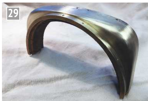
29 The Modelworks upper 'throat piece' heavily reshaped to a better profile.
