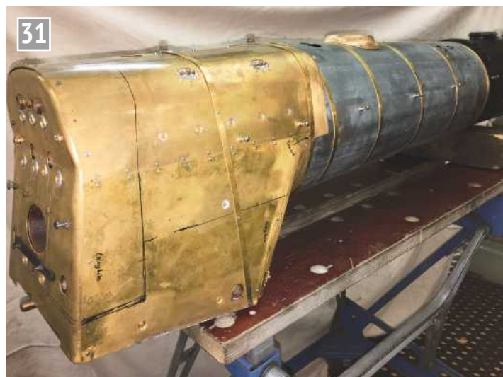
31 Boiler cleading finished with added washout doors and plugs.
