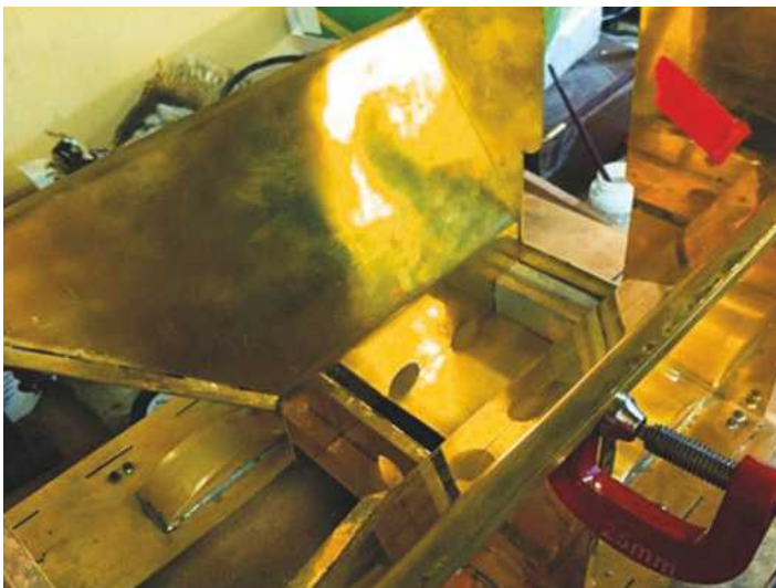
Front baffle held in place for brazing. The top right angle strips are also in place helping to keep the baffle square. Malcolm's kit is very well thought out; the right angle support sections fit neatly into slots already cut to accept them.
