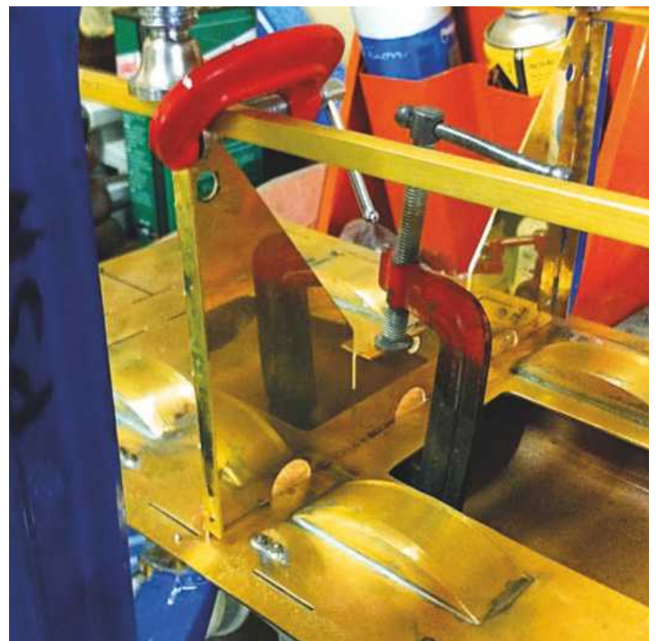
Front baffle held in place for brazing. The top right angle strips are also in place helping to keep the baffle square. Malcolm's kit is very well thought out; the right angle support sections fit neatly into slots already cut to accept them.
