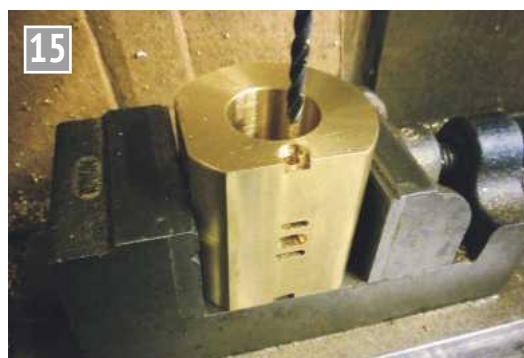
Drilling a steam passage.
