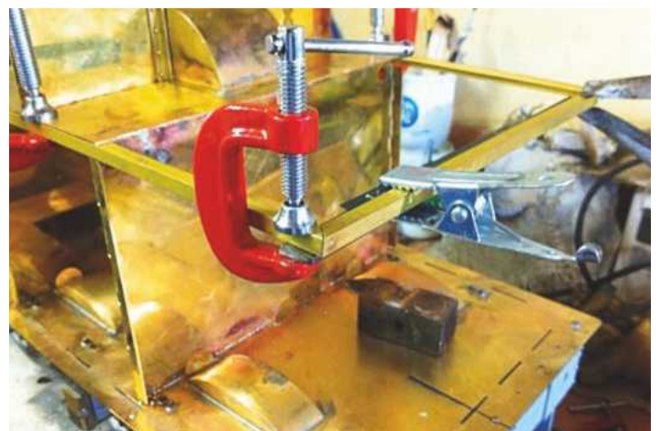
With the right angle now brazed to the baffles it was time to attach the rear section. The 45 degree angles on the right angle have been measured and cut in preparation for assembly.
