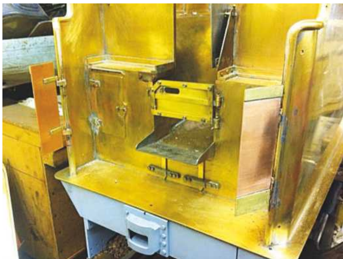
We can see here that both doors are tested in place. I later gave the affected area a good clean and ensured that the doors hung correctly.
