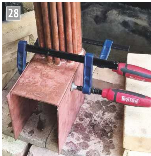
Forming the inner firebox wrapper.
