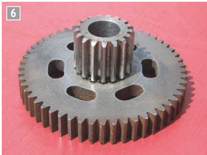
The repaired gear cluster.
