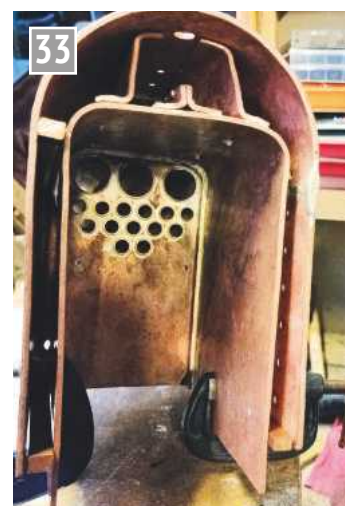
Fitting the firebox into the shell.
