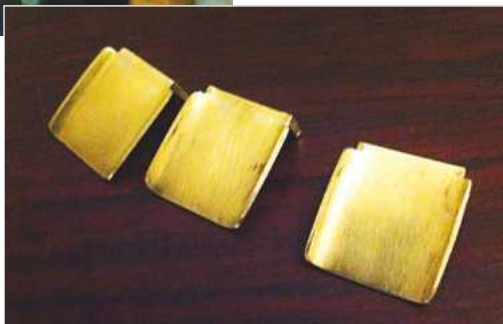
With the basic shape formed this step was then silver soldered to a rectangular piece of brass for the support bracket.
