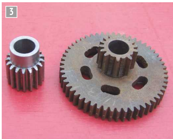
New pinion compared with the old, broken one.
