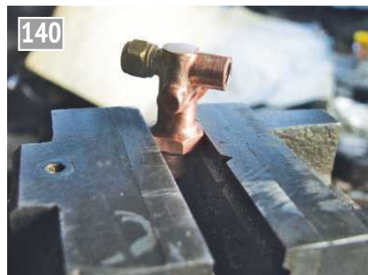
140 The gauge bottom fitting has been fully assembled, silver soldered and cleaned up, the outlet pipe connection being protected with a union nut.
