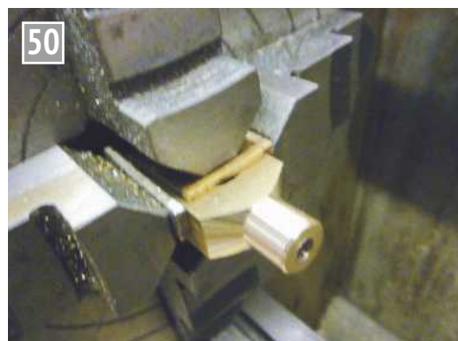
Machining the boss on a crank connection.
