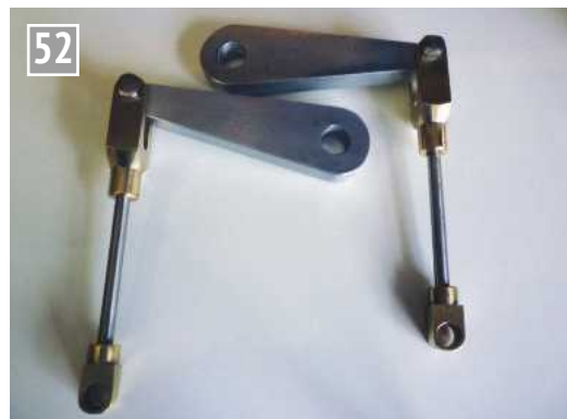
Finished connecting rods with rocker arms.
