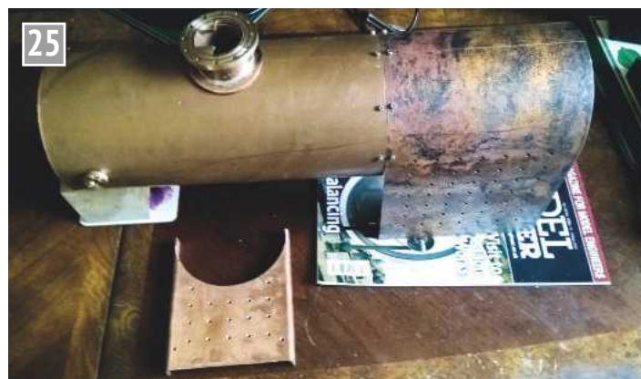
The firebox wrapper fitted to the barrel.
