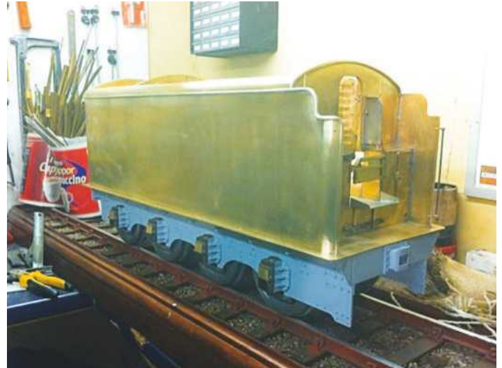
Here we have the tender with its beading permanently fitted.
