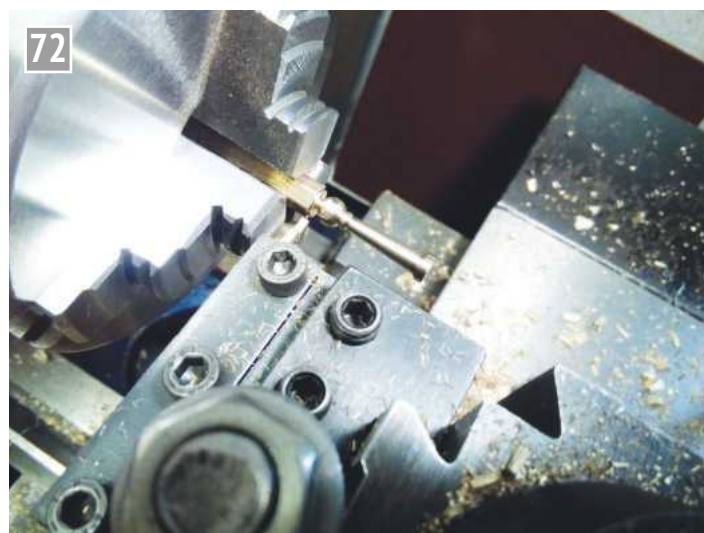
Machining the handrail stanchions.
