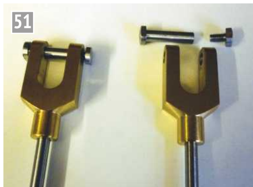
Bosses mounted on the connecting rods.
