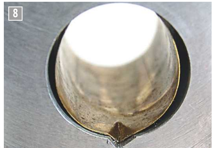
Locating the shim in the laser pointer bore.
