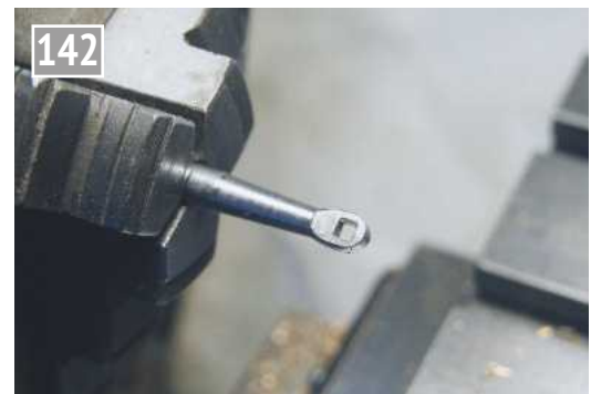
This picture shows a valve handle being made and the taper turning carried out ready to cut it off and put a small dome on the end.
