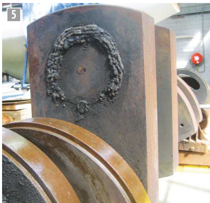
Attempted welding of crankpin 1958 style.
