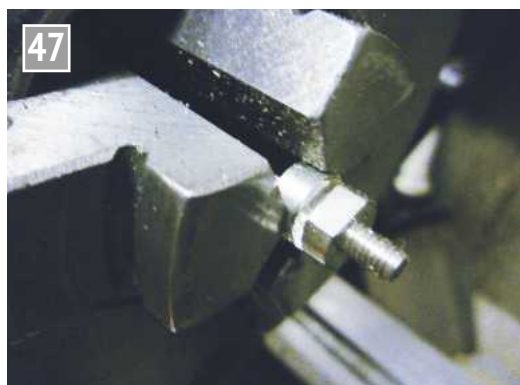
Turning a crank rod rocker end pin.
