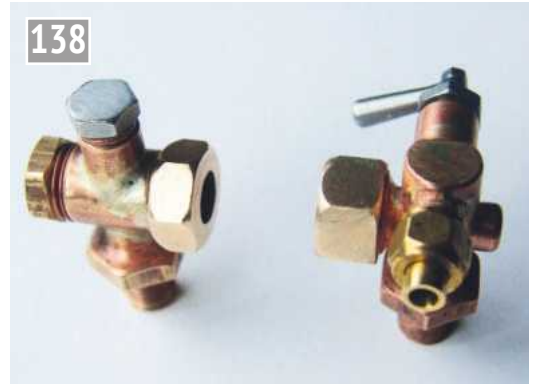
138 This view of the assemblies shows the left hand (upper) fabrication drilled and tapped with the two blanking plugs added. These have not been detailed on the drawings as they are simple turning exercises from brass or stainless steel.
