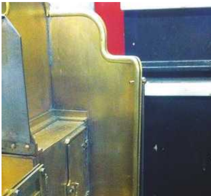
Next up was the rear of the coal bunker panel, similar to the front, and followed by the rear panel itself. Both now have the beading soldered in place.
