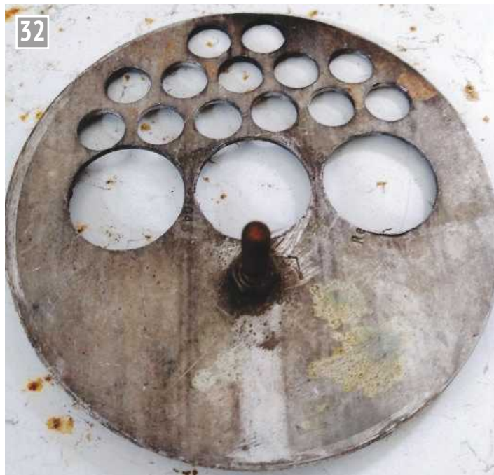
Improvised jig for locating the tubes.
