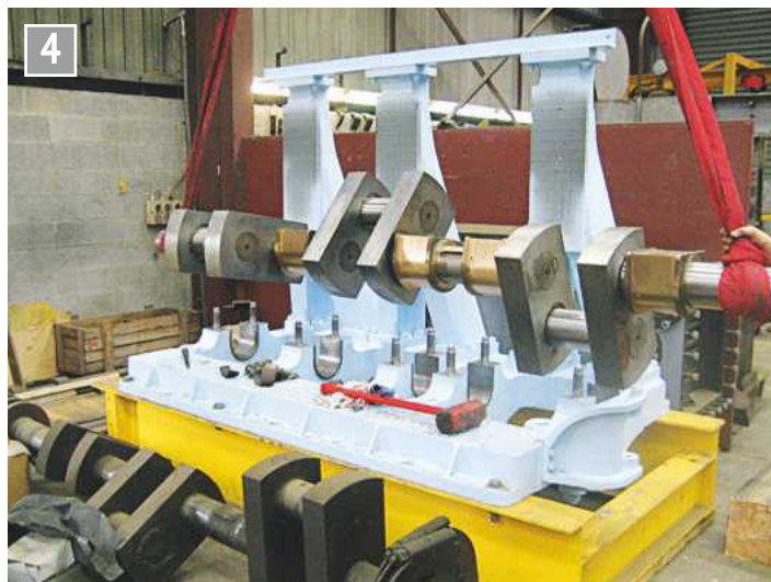
New crankshaft being lowered into engine bed.
