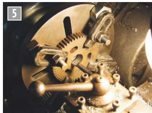
Boring out for the new pinion.
