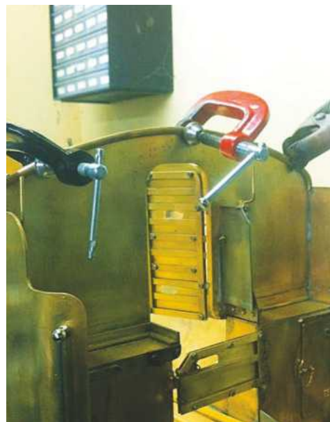
Steps fitted with 8BA hex heads, like the lamp irons.
