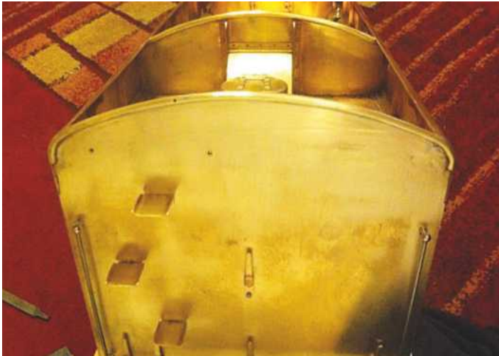
Next up was the rear of the coal bunker panel, similar to the front, and followed by the rear panel itself. Both now have the beading soldered in place.
