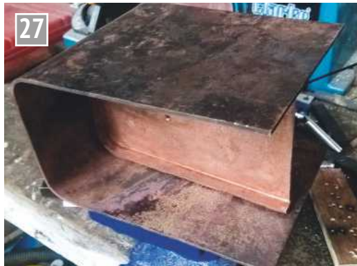
Forming the inner firebox wrapper.
