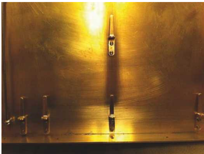
Rear lamp irons fixed in place. Currently these are held by steel hex head bolts but since these go through to the water tank I shall change these for stainless at a later date, along with any others that do the same.
