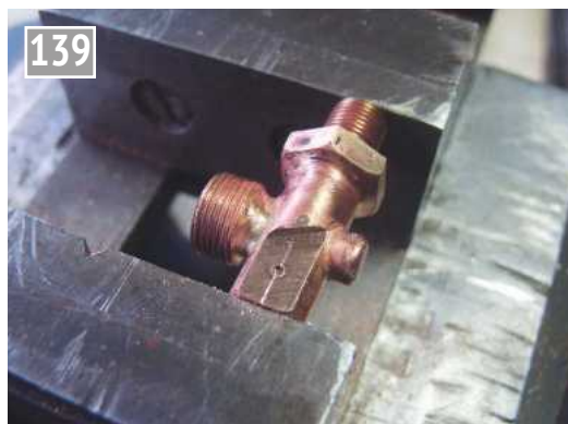
139 Here a flat has been filed onto one side of the main assembly and a centre added so a hole can be drilled through and it will be a contact face for silver soldering in the valve body. This feature dictates which hand the water gauge turns out to be.
