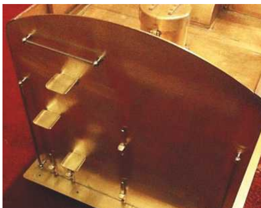
Steps fitted with 8BA hex heads, like the lamp irons.
