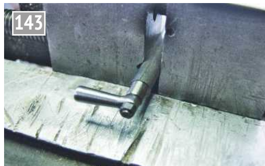
Here the square has been carefully filed on the valve rod and the handle fitted. Ideally it should be able to be assembled at any of the 90 degree positions.
