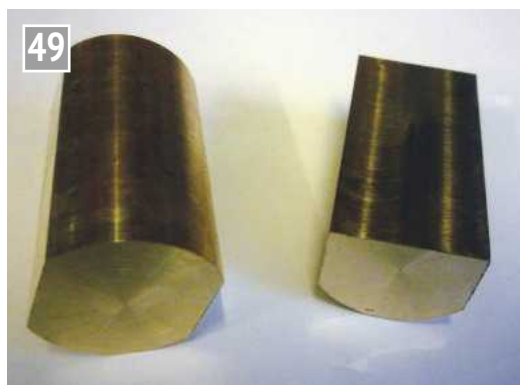
Blanks for the crank/vibrating arm connections.
