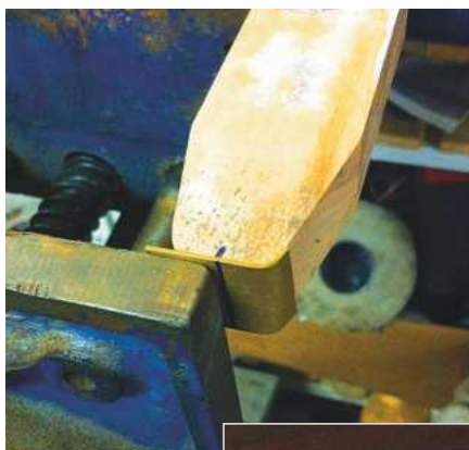
With the basic shape formed this step was then silver soldered to a rectangular piece of brass for the support bracket.
