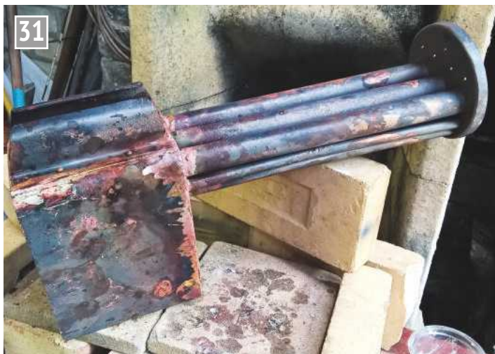
Firebox wrapper united with the tubeplate.
