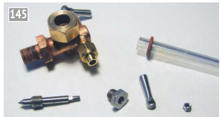
Here is the disassembled set of components for the lower gauge body with the end plug included. This has not been described but the machining is straightforward and a short length of graphited yarn should be added on final assembly to be a buffer between the valve thread and the end plug as a seal.
