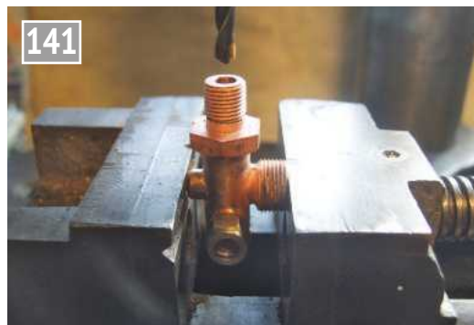
The lower fitting is being drilled initially with a \frac{1}{32} inch drill to make the water connection through the glass fitting and then a \frac{1}{16} inch drill is used to connect into the valve body.
