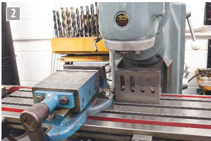
Initial set up of machine vice and angle plate in preparation for early stages of machining cylinder blocks. Photograph shows machine in vertical mode.
