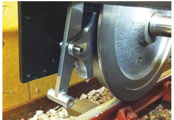
This photo is an inside view of the rear axle. I can confirm that there is indeed an error for the third brake hanger as has been mentioned by others regarding 'drawing errors' before me. It's nothing big - just needs some metal removing from the back edge of that particular brake hanger to allow enough clearance for the shoe to fit between the hanger and wheel without fouling the rear stay.
