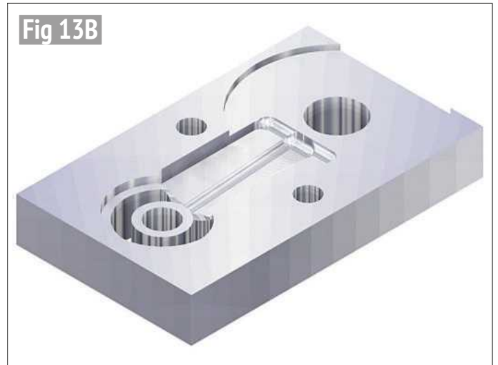
Stage 10 - A circular slot was milled right through to dimensions and angle with an \frac{1}{8} inch square end slot drill. There was obviously no need to reverse the part in the fixture on this stage. This produced the outside diameter of the small end.
