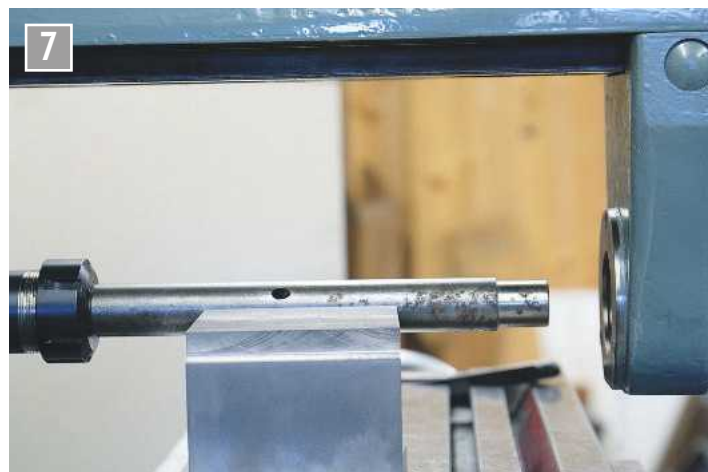
Showing just how little space there was between the end of the boring bar and the overarm bearing bracket.
