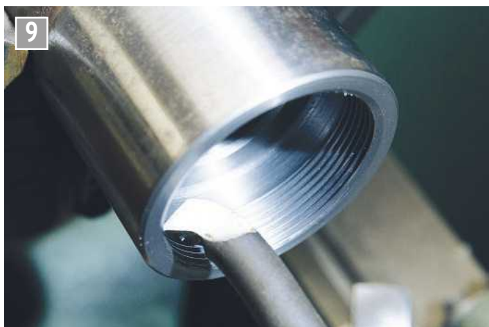
Close up view of the internal screwcutting operation of the retaining cap.
