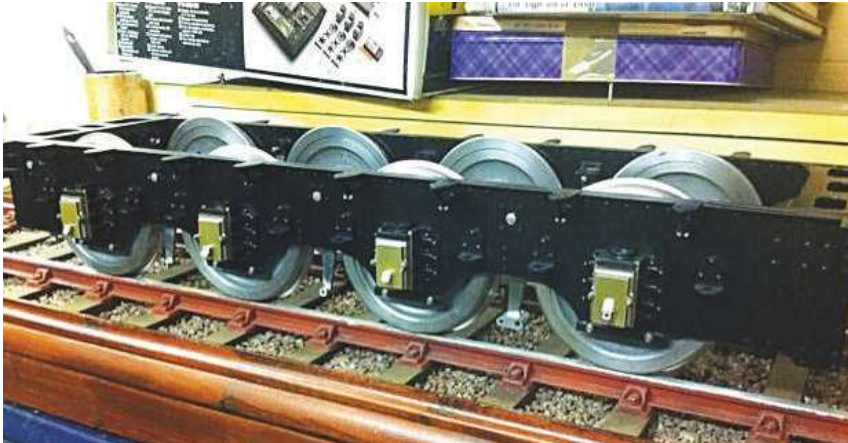
Brake hangers fitted. The front hanger has two bottom holes - one (large) is for the front brake beam, the second being for the first control rods.
