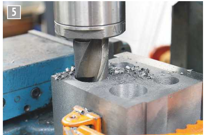
Removing bulk waste with 1\frac{1}{4} inch slot drill.
