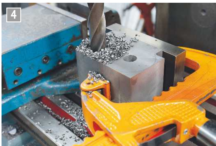
Opening out hole with large drill in milling machine.
