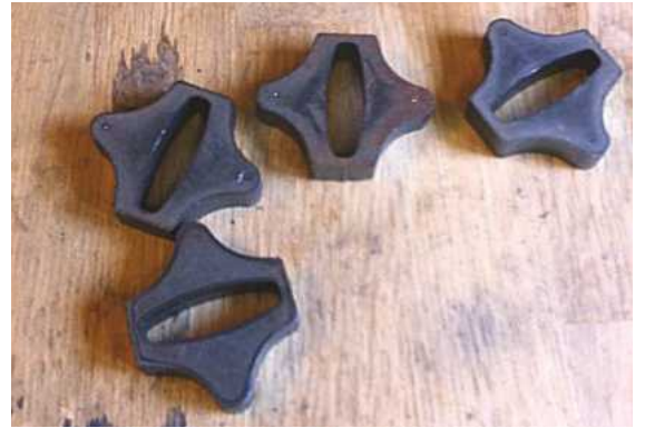
It was then time to tackle the brake shoes. In the photo are the laser cut shoes from Model Engineers Laser. Having now machined these I think it may have been quicker to machine from solid. Being such thick material, the laser had hardened the edges deeply and cut at a slight angle in places plus the material was thicker than the drawing so had to be machined to size. They also needed making symmetrical too. Still I persevered and battled on...
