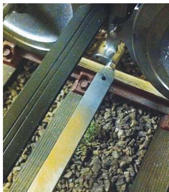
This photo is an inside view of the rear axle. I can confirm that there is indeed an error for the third brake hanger as has been mentioned by others regarding 'drawing errors' before me. It's nothing big - just needs some metal removing from the back edge of that particular brake hanger to allow enough clearance for the shoe to fit between the hanger and wheel without fouling the rear stay.
