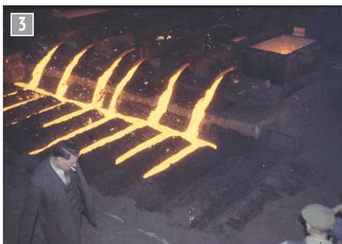
The excess forms 'pigs' of iron.
