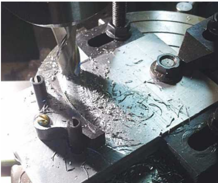
Here is the jig I made/used for holding each shoe while its inner face was machined to 2\frac{1}{2} inch radius. The pin hole has already been drilled to No.30 and used to help hold the shoe rigid between the two 5mm roller pins. Next stage was to mill the slot that slides over the brake hanger and is then held by the pin. The pins were made the same way as the larger hanger pins.
