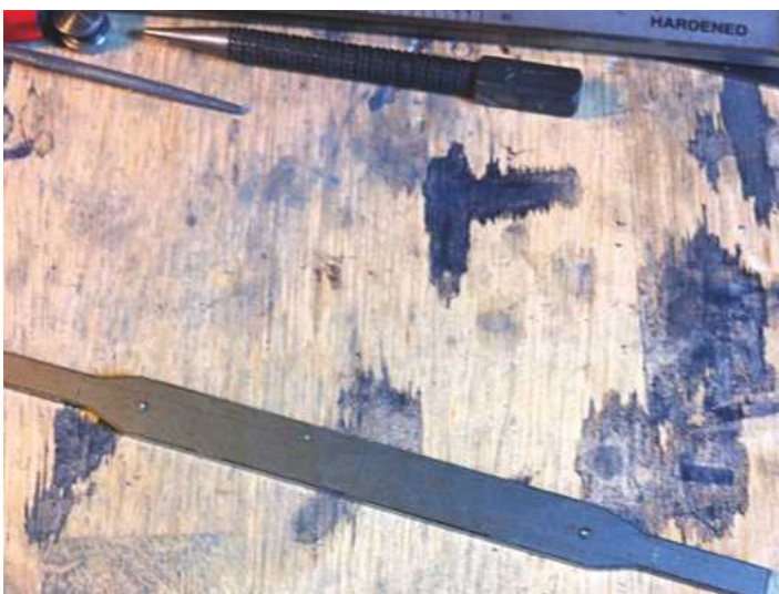
Continuing with the brakes here we have the last laser cut part from Malcolm's brake hanger kit. This is the front brake beam. If you look closely you'll spot the ascribed lines across the end tabs. I decided to remove these and turn up the required \frac{5}{32} inch diameter spigots separately and silver solder them on.
