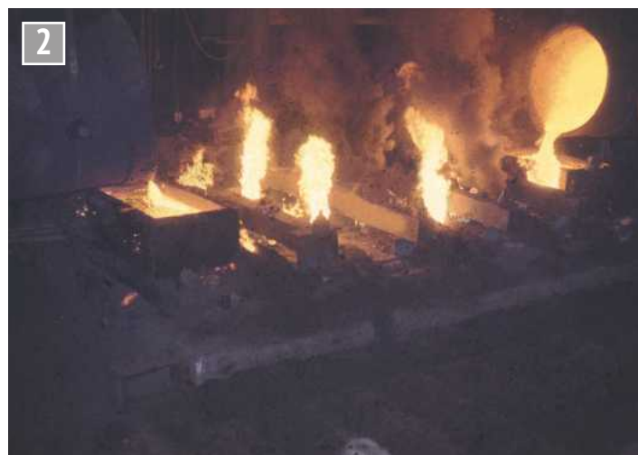
Flames emitted from the risers during the pour.
