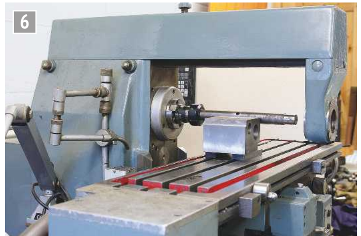
Initial set-up on milling machine to assess how much space was available.
