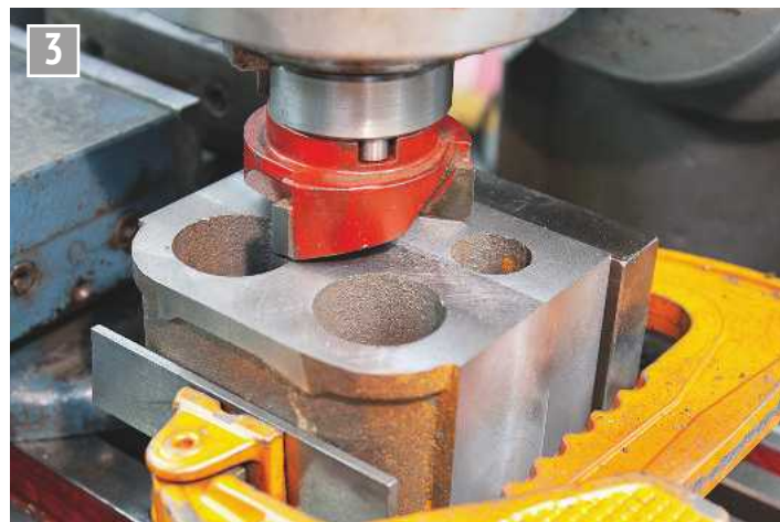
Carbide tipped face mill used for machining the flat surfaces. This photograph is posed and shows machining of one of the actual castings.
