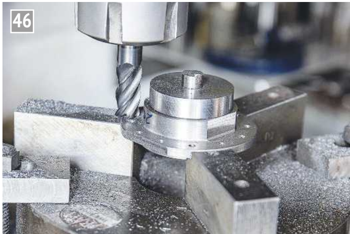
Machining the two flats for the slide bars to be bolted on to. The side teeth of the cutter are being used and there is a very slight radius on the tooth corner.
