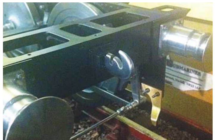
11. The finished hook in place. The end profile is basically a taper from ⅜ inch at the bottom to just over 1 mm at the top and then everything is rounded off to finish.
