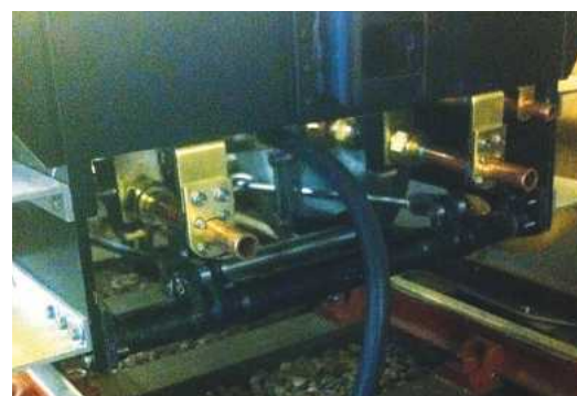
4. A general wider view of the pipework showing the two water pipes for the injectors. I have tried to replicate the general appearance of these brackets as seen in some of the photos of full size shown by Don in his words and music. On researching this it seems that things varied a lot on different tenders so I've used a little modeller's licence in doing this but I think overall it looks good.
