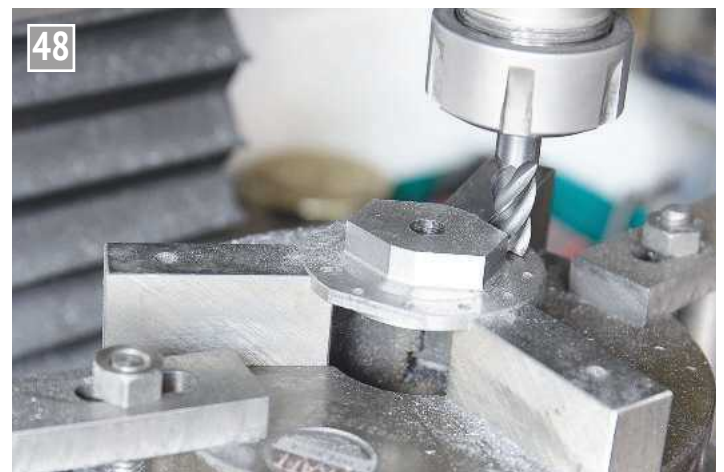
Rotary table slewed 25 degrees either side to cut the lozenge shape of the boss.
