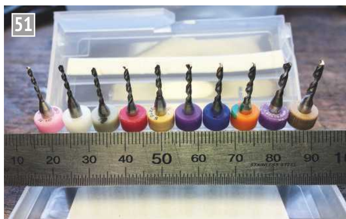
Carbide PCB drills self centre on the work and are very sharp.
