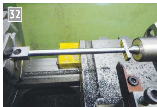
Taper turning the conrod with a round insert tool.
