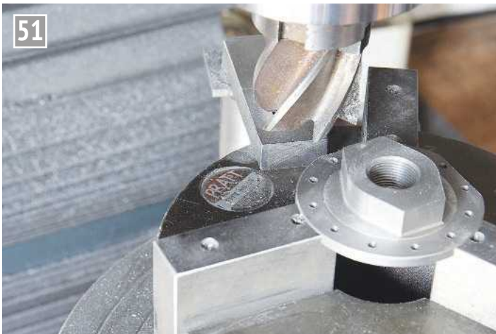
Cutting the small scallop to give clearance to the underside of the piston valve liners.
