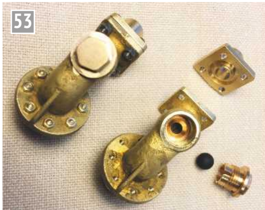
53 The two top feeds, one showing an inset bronze cone seat and O-ring groove for attached pipe flange. Note the cage cut into the top nut to retain the rubber ball.
