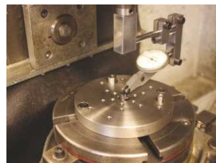
Concentrica – Pete Worden's aid to setting up a rotary table.
