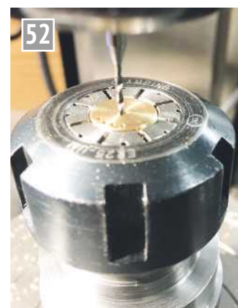
Threaded safety valve screw adjuster gripped easily in an ER25 collet, with the work moved on a rotary table between each drilling operation.
