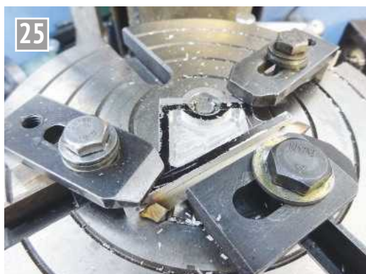
Milling out recessed detail to sides of the pedestals.
