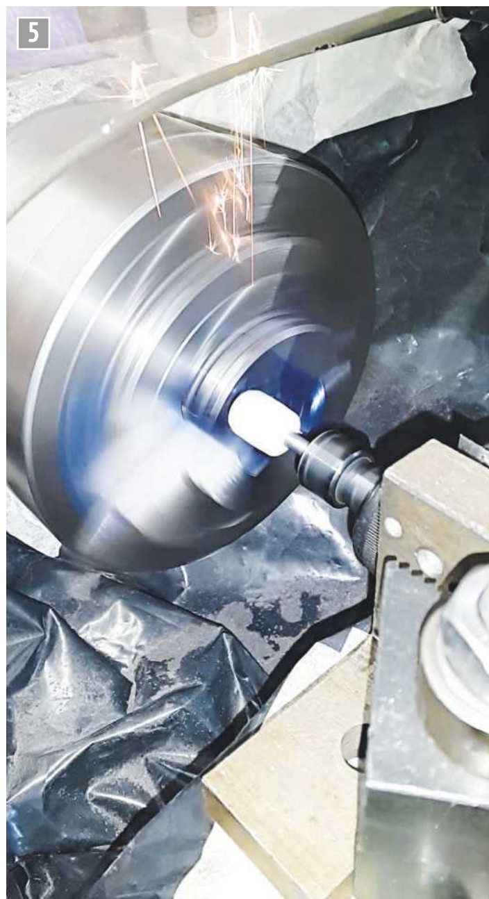
Toolpost grinding to true chuck jaws.
