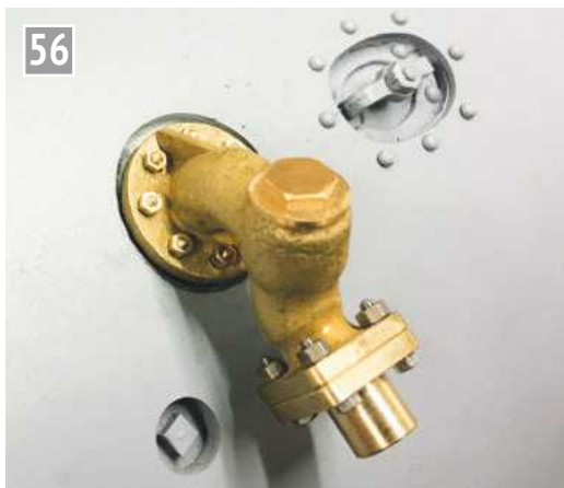
56 The screwed in top feeds unfortunately sit too high on the boiler. They should be recessed into a cut-out in the cleading.
