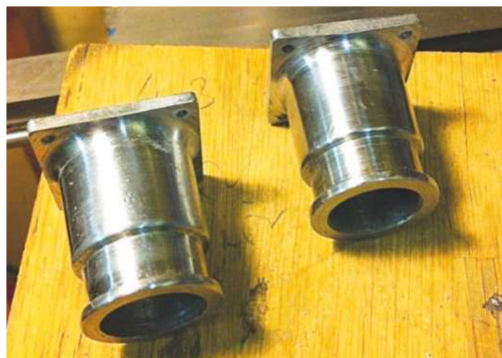
5. The completed buffer stocks - polishing to remove machining marks was done after taking this picture.
