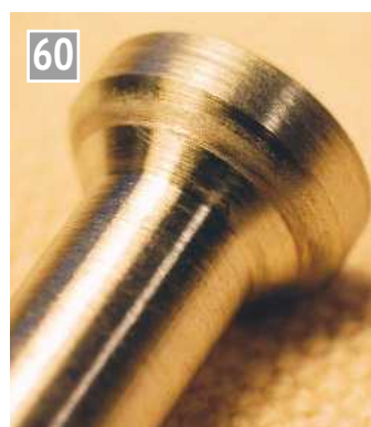
60 Grey seating line seen on the spindle conical face.
