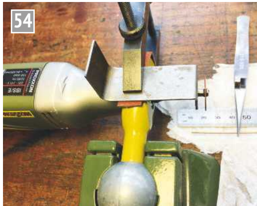
54 Proxxon drill and thin cut-off disc with guide for cutting consistent lengths of 12BA studding.
