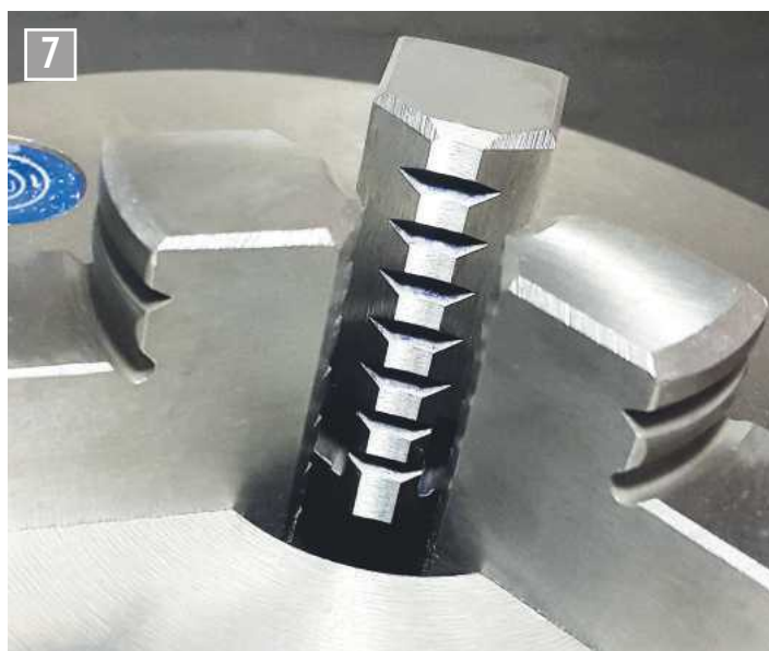
Toolpost grinding to true chuck jaws.
