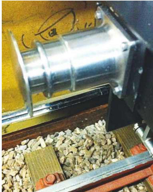
7. The finished article now temporarily fitted to the buffer beam. The frame is directly behind it, so the stock needs to contain all of the spring mechanism to work.
