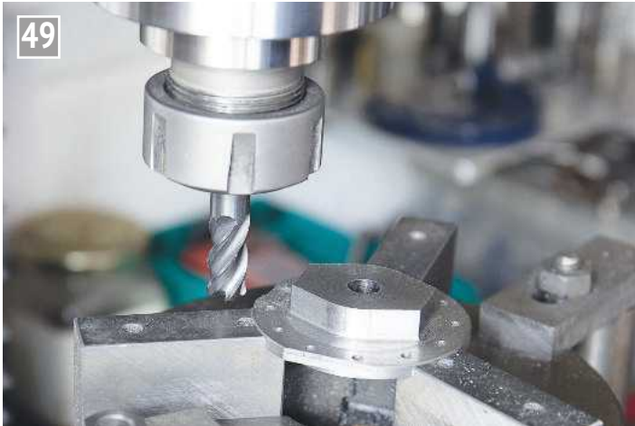
The two sloping surfaces blended with a small rotating movement of the rotary table.
