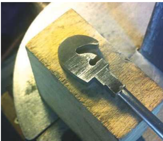
8. The parts brazed together. Some may say a single piece would be stronger – perhaps so if the joint is weak but with good penetration it should be as strong if not stronger. However, Don states that Doncaster being a very powerful locomotive, and able to haul large loads, a more suitable arrangement should be used rather than the hook and coupling shackles, which is normal practice anyway. So this will only be for display purposes and I'll use a clevis type for actual running.
