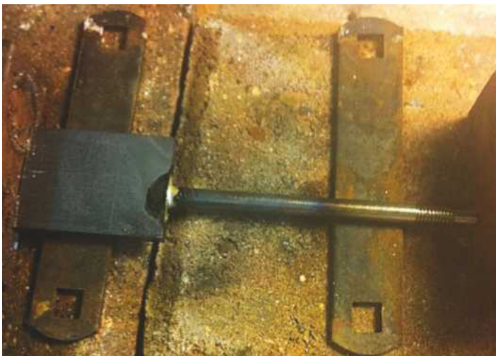
8. The parts brazed together. Some may say a single piece would be stronger – perhaps so if the joint is weak but with good penetration it should be as strong if not stronger. However, Don states that Doncaster being a very powerful locomotive, and able to haul large loads, a more suitable arrangement should be used rather than the hook and coupling shackles, which is normal practice anyway. So this will only be for display purposes and I'll use a clevis type for actual running.
