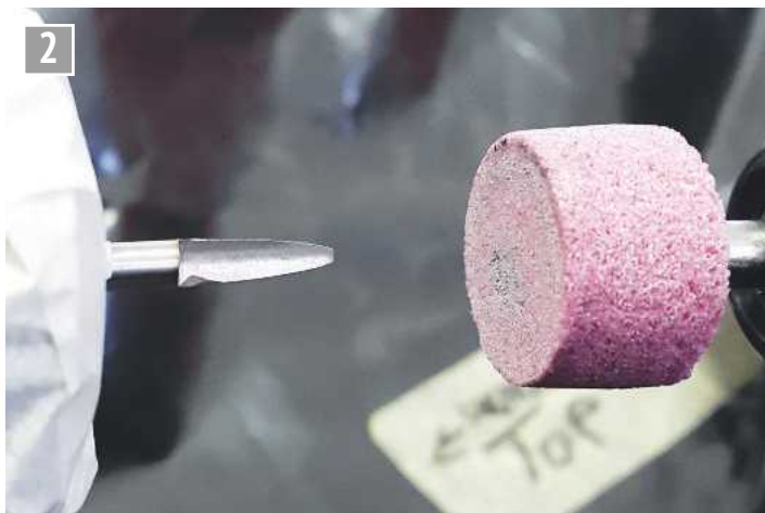
Reamer - first surface ground.
