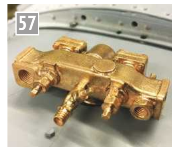
57 Commercial manifold casting, drilled and threaded ready for pipework to be attached.
