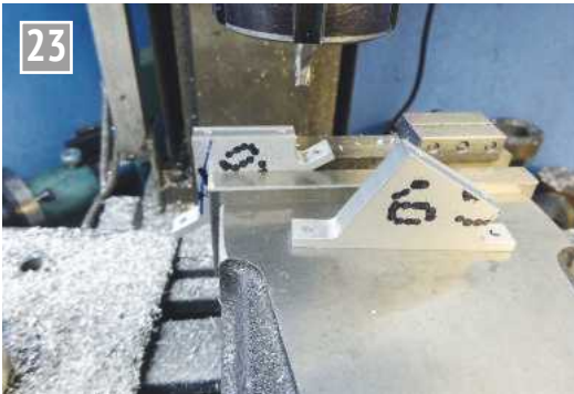
Pedestal profile being milled.
