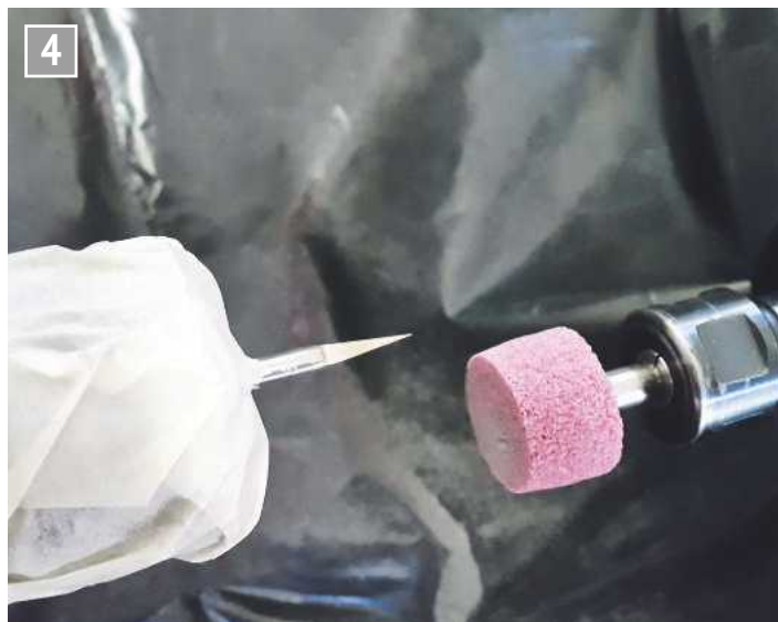
Reamer - Final surface ground ('D'-cutter at the end).
