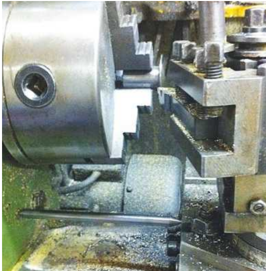
6. Here the buffer head is seen being machined using the method that I picked up from reading John Baguley's post on one of the engineering forums (2½ Inch Gauge Association). As you can see there's a steel bar with points machined each end to act as a pivot (seen below the chuck). The length of the bar is calculated to give the correct radius of the buffer head by the arc that it forms. The saddle needs to be loose for this to work.
