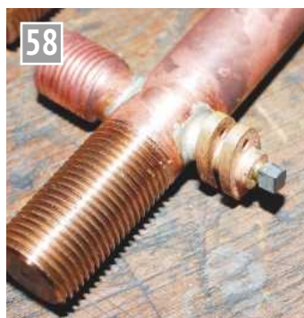
58 Outlet stub and dummy top detail silver soldered to a cross drilled body. Long stub remaining to allow gripping in the chuck for drilling through.
