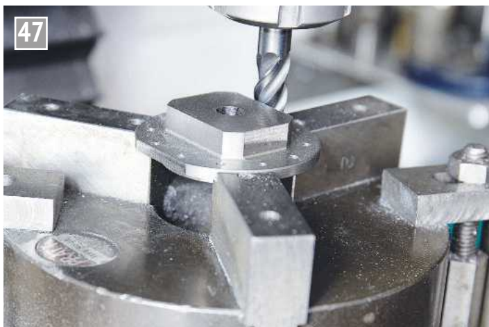
Machining the two vertical flats on the rear cylinder cover prior to profiling the boss.
