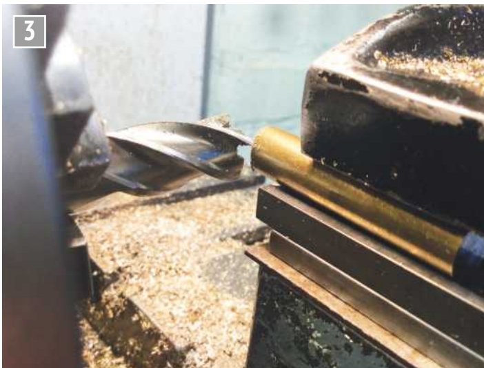
Milling the saddle shape for brazing. The workpiece is held in the toolpost.
