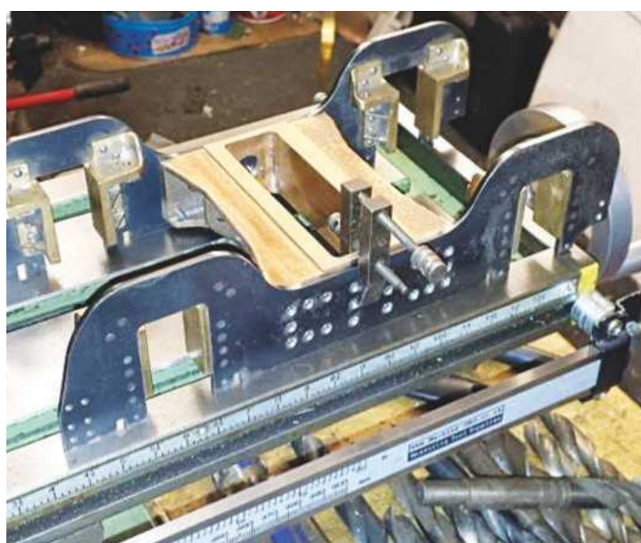
10. With the first side completed I then placed the bogie on to the mill bed and clamped the other side into position checking that the centre lines lined up, that the height was correct and also checking with a square that the two frames were aligned correctly in relation to each other - it's easy to be a fraction out just relying on the centre lines. Once happy and with everything clamped tightly together I repeated the process exactly the same as for the first side - a long job but worth the extra care taken.
