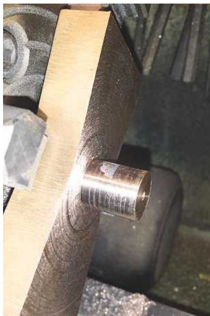
17. With the bolster set up in the four-jaw chuck the spigot is machined to size and a pilot hole drilled for the pivot bolt.
