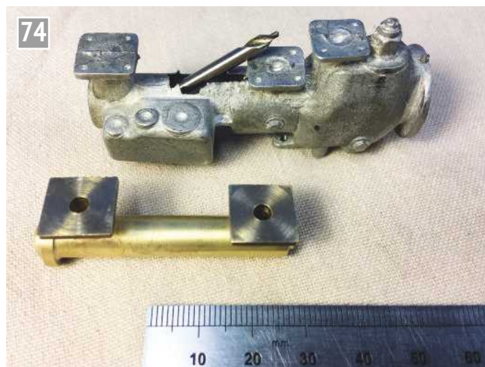
74 White metal 'Davies and Metcalfe Exhaust Injector' had an unfortunate hole. The repair pipe and flanges sit in front before installation.
