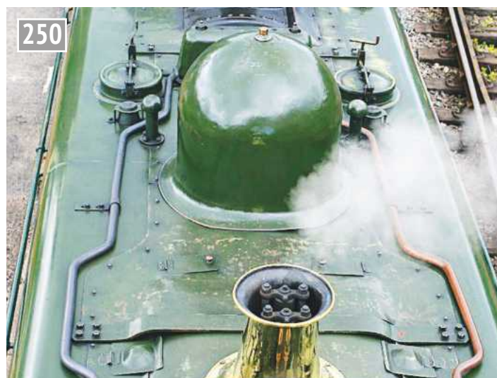
Top cover plate on pannier tank 5786.
