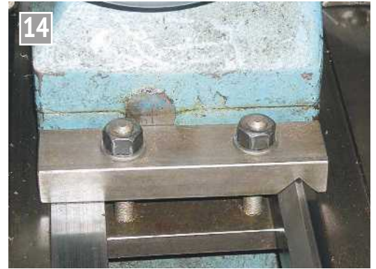
Tailstock clamp resists the broaching thrust.
