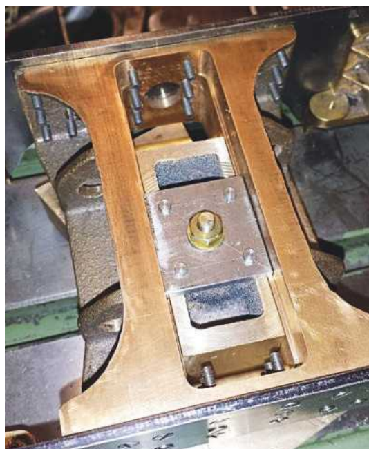
21. FAR LEFT: Here is the finished bolster sitting on its yoke. Of course, I still needed to drill and tap the mounting holes but will transfer these from the main frames as usual when ready.
