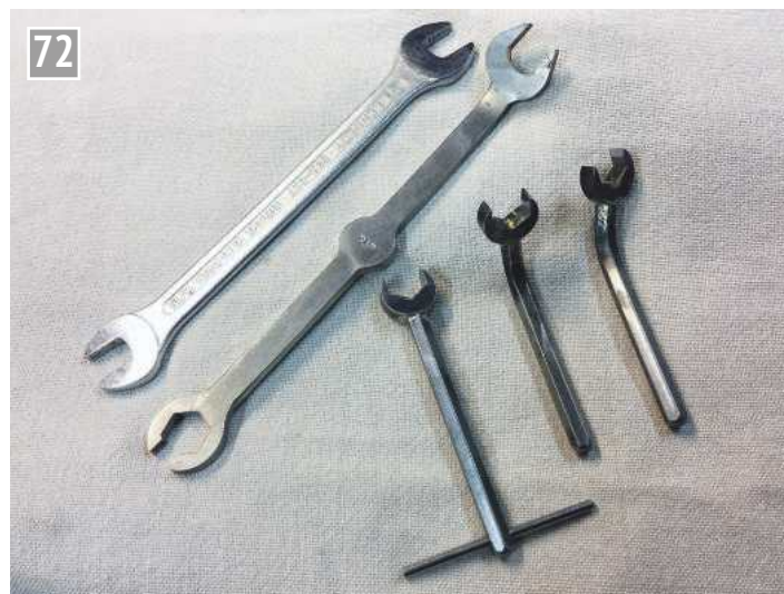
Two (long) commercial \frac{3}{8} inch A/F spanners with three home made angled, small spanners to fit tight spaces.
