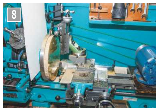
Cutting teeth on the sidereal wheel.
