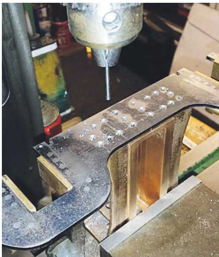
9. With the two parts reassembled and placed back in the machine vice it was a straight forward job to spot and drill the other 18 holes to complete the first side. The last job was to tap the remaining holes the same as the first two.
