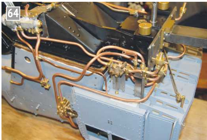
'Even more pipework' - an inverted view of the model showing some of the extra pipework running between the cab floor and frames, to service the 'real' model injectors.
