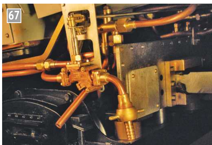
Left mounted water valve and crank to cross rod above. Behind is the left mounted model injector. An extended injector overflow comes out under the valve.
