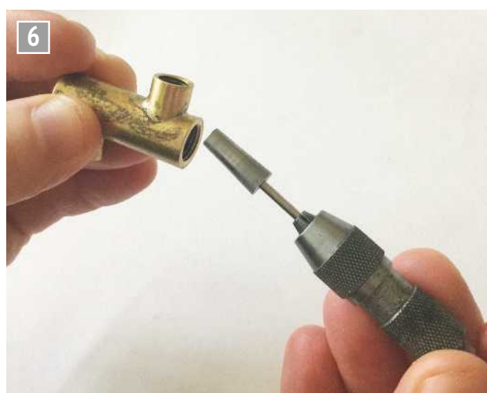
Grinding-in the valve, using a pin chuck and rod to hold it.
