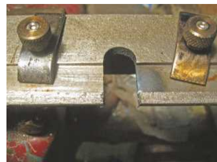
Will Doggett makes a bandsaw blade repair station.
