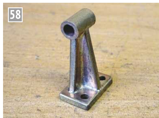
Valve guide after soldering and drilling.
