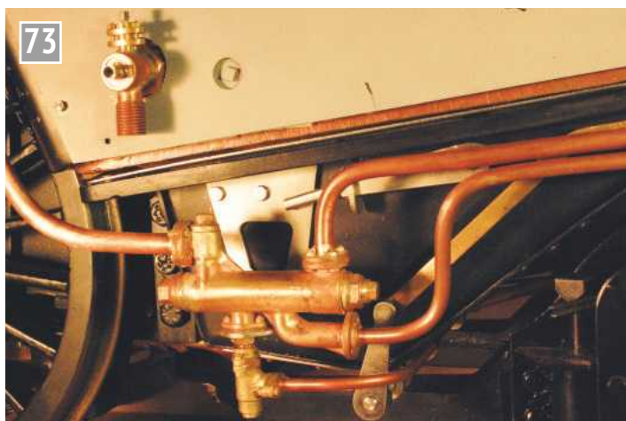
73 10X steam injector is a dummy, but piped through to carry feed from the left model injector to the left side boiler top feed clack. The lower two pipes are for show.
