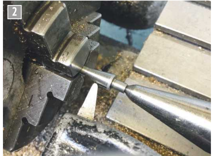
Turning the valve, using a live centre for support.
