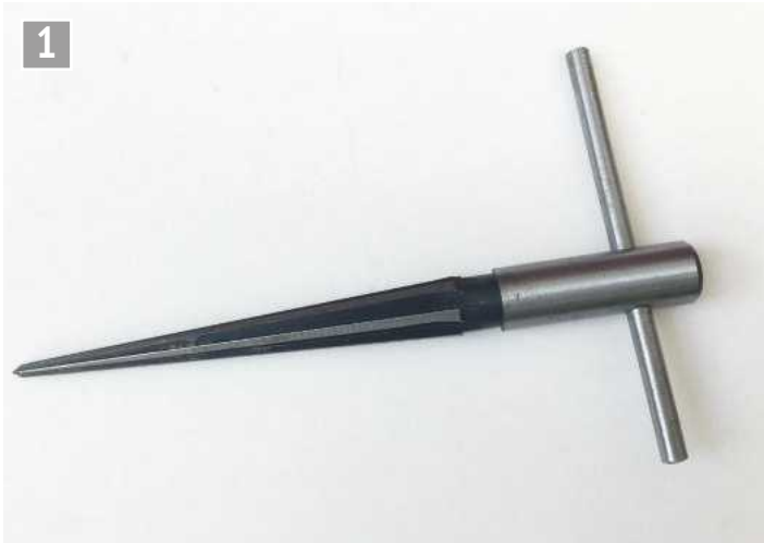
Hand reamer normally used to enlarge holes in sheet material.
