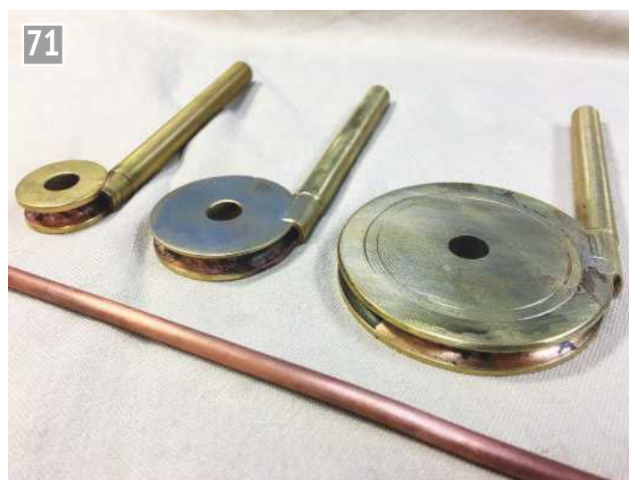
Three \frac{5}{32} inch pipe bending rollers for radii of \frac{1}{2} inch, \frac{5}{8} inch and 1\frac{1}{8} inch.
