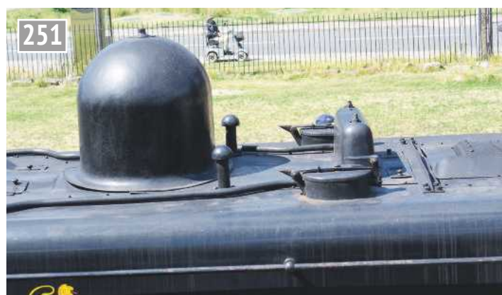
Top cover plate on pannier tank 9681.
