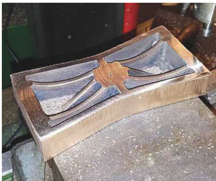
19. A fly cutter is used to finish the bolster casting to \frac{3}{4} inch depth.
