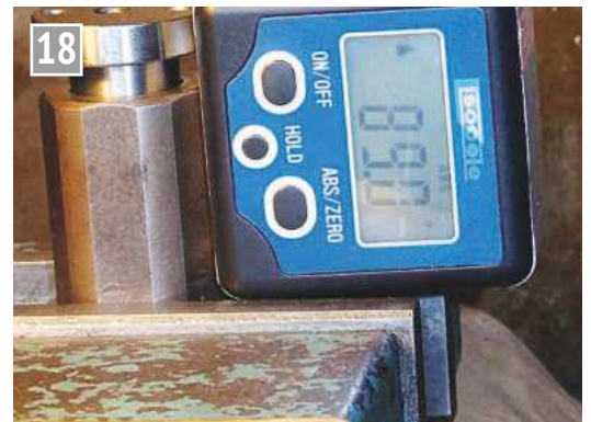
Setting the angle of the work in the machine vice.
