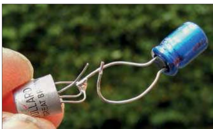
Fig.43. The TO7 tin-whisker problem can often be fixed with a capacitor discharge. This trick has saved many classic radios using AF114/5/6 or 7 and OC170 transistors. It has to be done every five years since the whiskers continue to grow.
