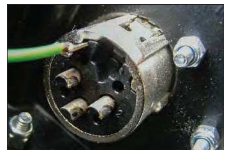
Fig.27. Metal cases can be earthed off XLR sockets via an earthing tag on the rear of the socket connected to the PSU 0V.
