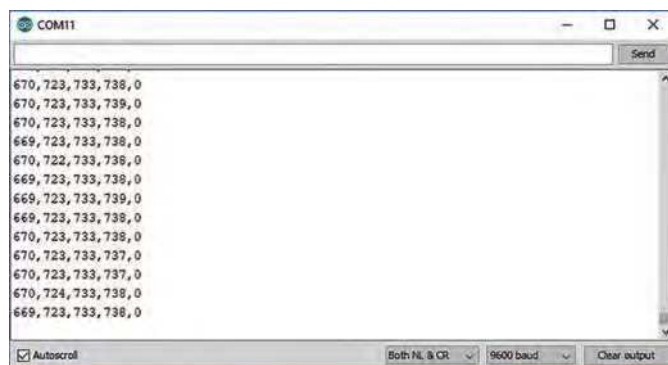
Fig.3: example output of the ADC sample values corresponding to the sensed relative capacitance for each of the four pushbuttons and the slider. You can see that the four first values are fairly steady over time, while the last value is zero. If you bring your finger near or touch a button, one of the values will increase, indicating the added capacitance from your finger.
