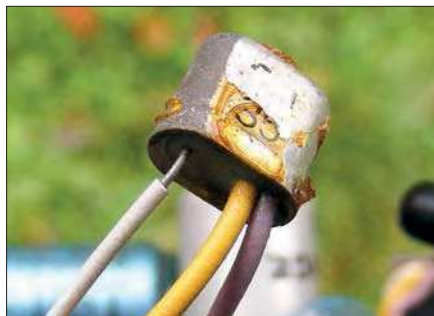
Fig.47. One of the first NPN transistors by Sylvania, who specialised in NPN devices. The 2N35 in its distinctive SO-4 can from an ancient Lin/Dinsdale amplifier in an old organ. Introduced in 1953, this transistor cost $4.45 in 1955! Jack Dinsdale used a similar device, the Syl 1750 which cost the considerable amount of 25 shillings (£1.25) from Home Radio , March 1962.
