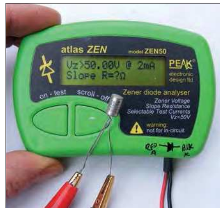
Fig.51. Testing transistors for collector-emitter voltage breakdown ( V_{ce} ) with a Peak ZEN50 Zener diode tester. This AC188's V_{ce} is much higher than its stated minimum -32V rating, and could replace the GET538.
