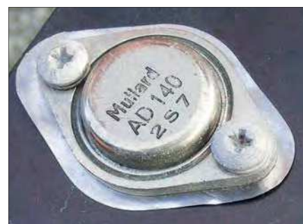
Fig.38. Mullard AD140 power transistor and heatsink. Note the soft metal washer is electrically conductive, so the heatsinks are 'live'. Is the date indicated by the three-character code?
