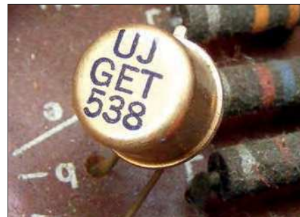
Fig.48. GET538 (TR6), a hard-to-get PNP driver transistor, replace with an ACY17.
