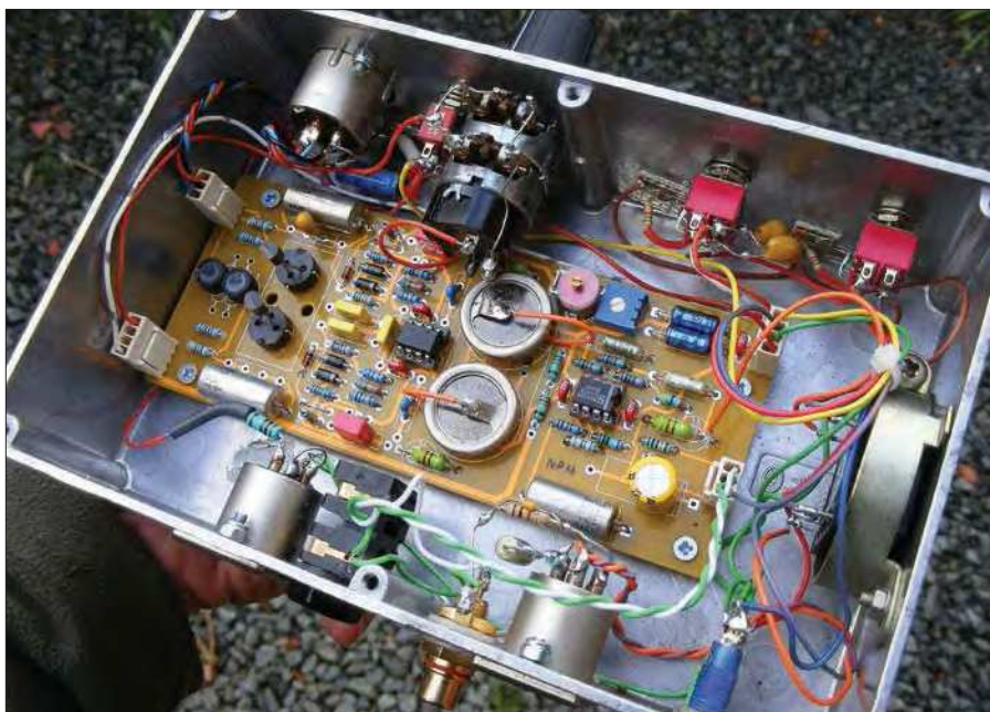
Fig.26. A single-channel microphone preamplifier fits in this die-cast box, size 187 x 120 x 55mm. (Note the PCB shown above is a slightly different prototype).
