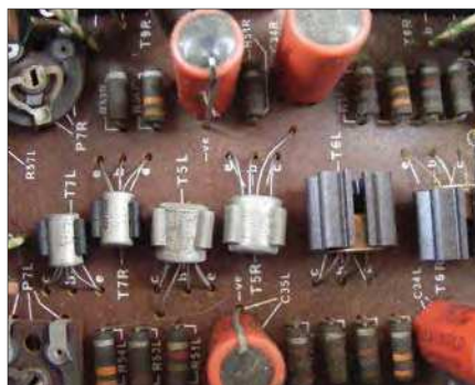
Fig.44. The two germanium driver transistors used in the Stereo 30, TR6 and TR7.
