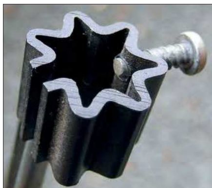
Fig.49. Tapped TO5 heatsink used for the GET538. People took great care with transistor mounting in the 1960s when they cost as much as a beer and sandwich.
