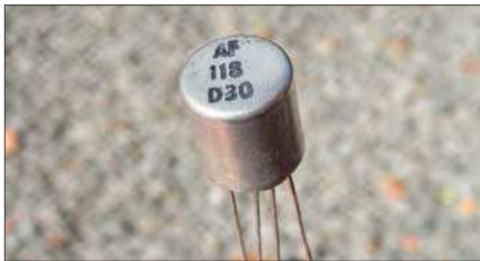
Fig.39. (above) GET113 small-signal transistor; Fig.40. (below) The enigmatic AF118 (TR5) – a rare germanium high-voltage RF transistor. Its data sheet was in the Siemens 1970-71 Semiconductor Manual , p.228.
