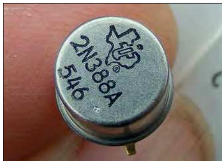
Fig.46. The mil-spec 2N388A NPN germanium transistor used by Toby Dinsdale. The late Bernard Patterson, a long-term PE subscriber, generously sent me a few.
