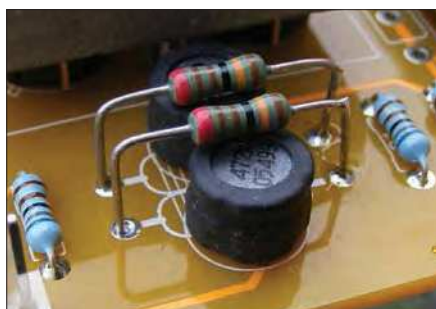
Fig.31. To reduce a minor amount of ringing on square waves, the input filter chokes L1 and L2 can be damped by wiring 1.3kΩ resistors across them (R28 and R29).
