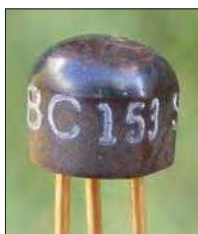
Fig.56. Later models of the Stereo 30 dispensed with the small-signal germanium transistors and used these early PNP silicon BC153 and BC154 transistors.
