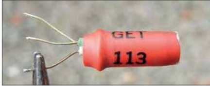
Fig.39. (above) GET113 small-signal transistor; Fig.40. (below) The enigmatic AF118 (TR5) – a rare germanium high-voltage RF transistor. Its data sheet was in the Siemens 1970-71 Semiconductor Manual , p.228.
