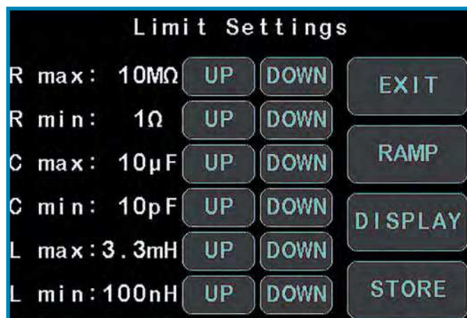
Screen2: pressing the SETUP button opens the Limit Settings page. There, Soft limits can be set to avoid non-useful or dangerous test values. Further settings can be found by tapping on the RAMP or DISPLAY buttons, while STORE saves the current setting to non-volatile Flash memory.
