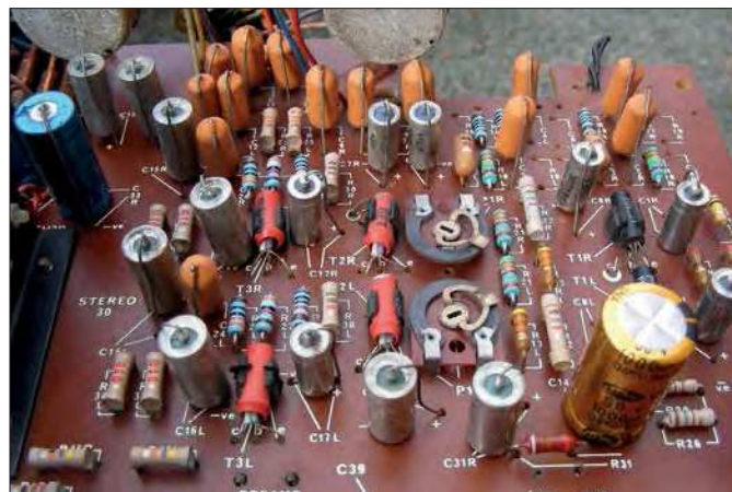
Fig.55. Old axial solid-tantalum capacitors make a good replacement for old axial electrolytic types; they seem to last forever. These ones were in an RAF store for 50 years, all perfect. Note the much larger, gold-coloured C14 decoupling capacitor.
