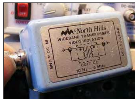
Fig.30. When testing balanced-input circuits it is necessary to use an isolating/balancing transformer between the signal generator output and preamplifier input.
