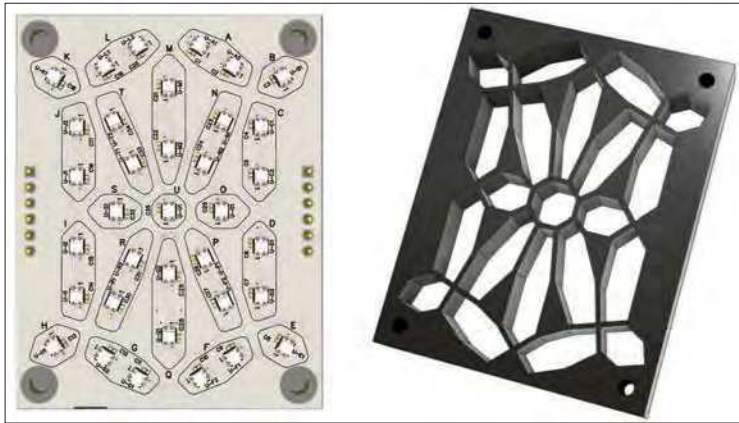
Fig.5. LED board and 3D printed shell for 21-segment display: a) LED board (left); b) 3D printed shell (right).
