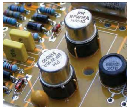
Fig.33. Transistors should be mounted in sockets so noisy ones can be easily removed. (It's also good for finding unknown gems in one's parts box) Transistors from Hitachi, Toshiba, Sanyo and Rohm seem to be the best. Only home constructors have time for this, so it is possible to improve on ready-made units.
