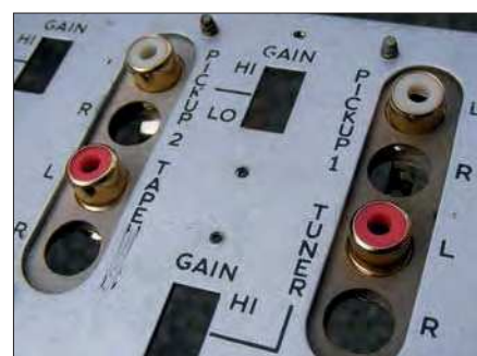
Fig.58. New phono connectors were required on the eBay amp, but were a pig to fit. I had to use the insulating plates from the old phonos.
