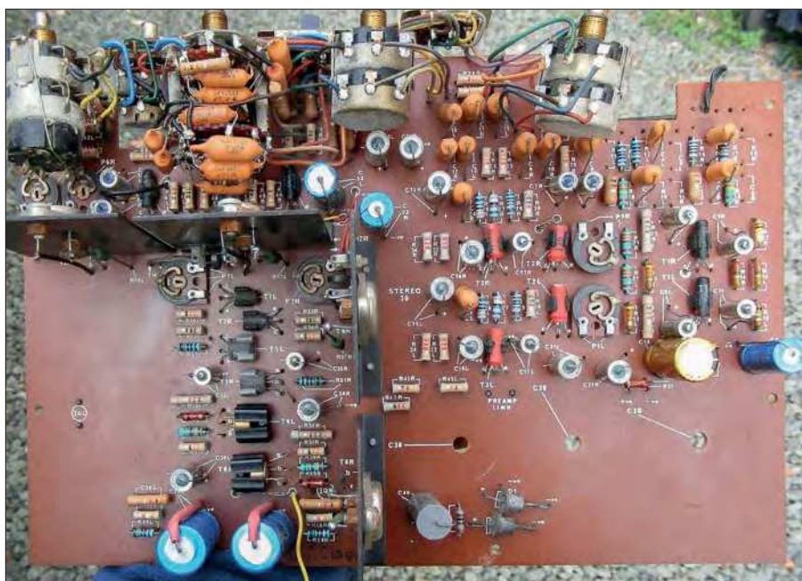
Fig.52. The DC bias point presets (P6) for the power amplifiers are hidden in the top left-hand corner.
