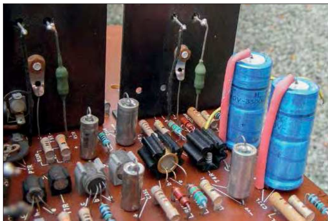
Fig.54. The original output capacitors were insufficient in capacitance and voltage. I installed these big axial Philips/BC electronics/Vishay electrolytics. The top of these caps is a good place to do the output half-rail voltage check.
