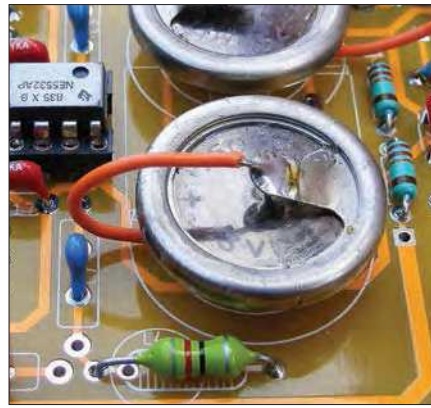
Fig.24. Note the green 82µH inductor, which looks like a strange resistor. The odd things that look like back-up batteries are Plessey Castanet tantalum capacitors.
