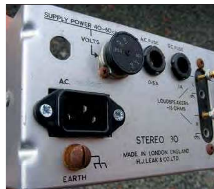
Fig.57. A lot of dumped equipment will have had their power cords cut off by overzealous technicians, especially in the public and educational sectors. It's a good excuse to then add a proper IEC mains connector.
