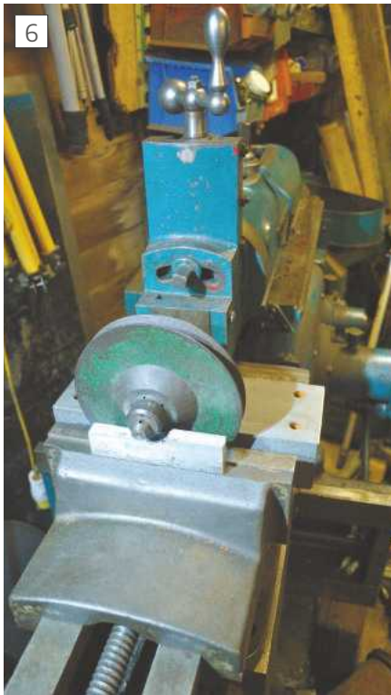
Setting up the pulley and tool for alignment in the shaper vice.
