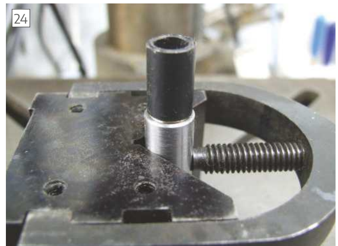
The acrylic tube has now been fitted onto the brass end cap.
