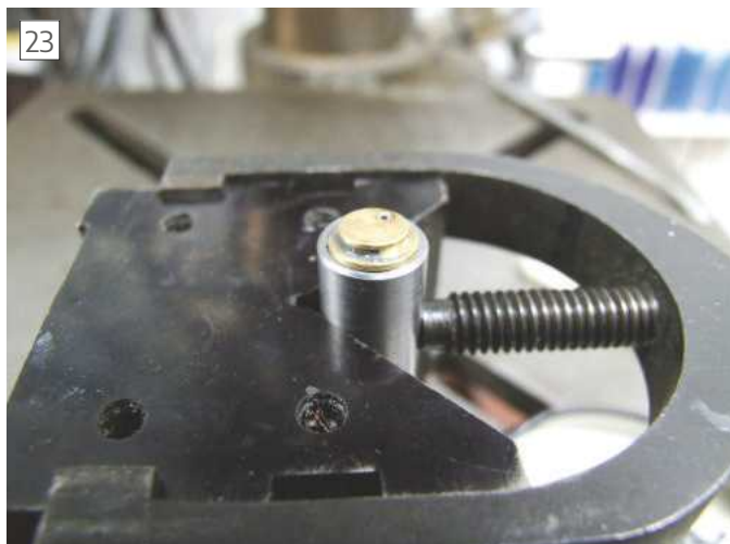
The brass end cap is located in its holder prior to applying the JB Weld epoxy adhesive.
