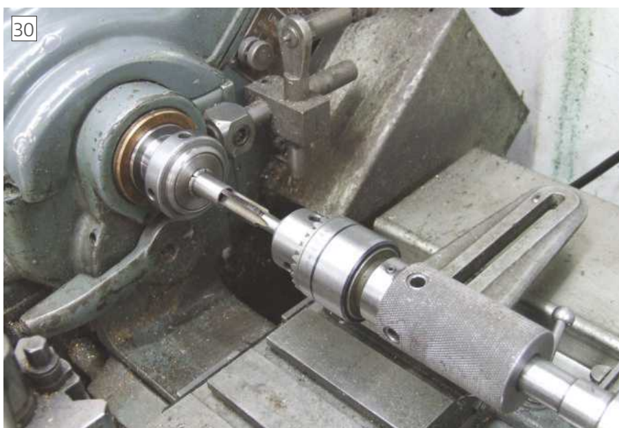
Using a plug tap to finish the 7/16" x 32 thread.
