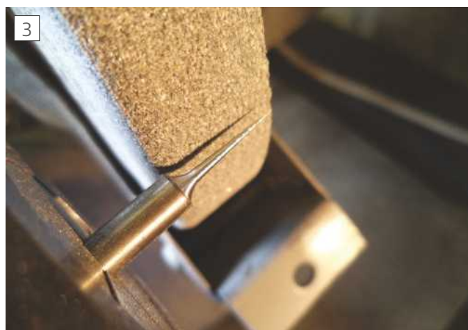
Grinding the taper by rotating by hand
