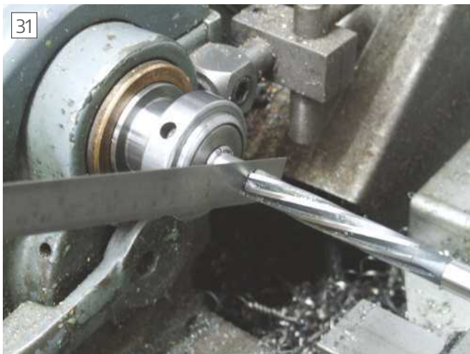
31 Setting the reamer to achieve 0.50" depth for the probe insulation sleeve.
