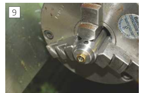
The depthing rod and collar being used to pull the nut against the face of the sleeve
