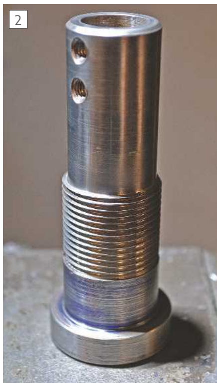
The adapter after machining and thread cutting
