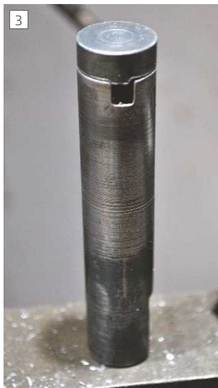
The tool bit holder after cutting the slot.
