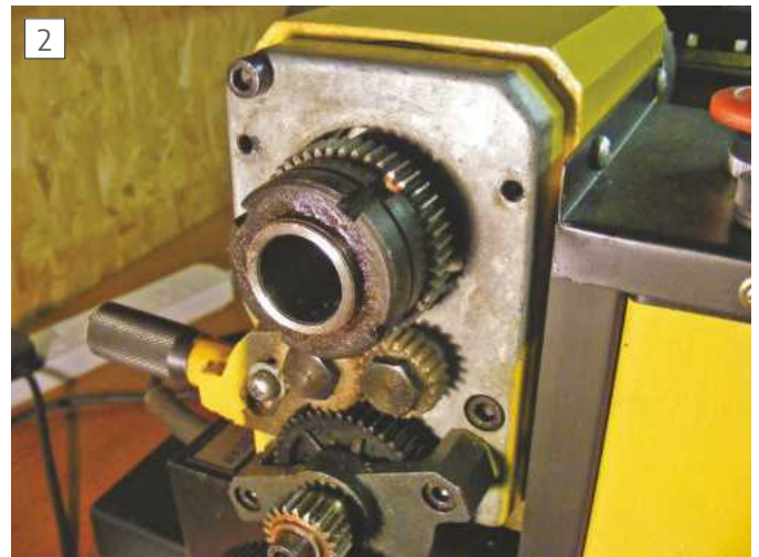
The rear of the spindle is directly over the change gears.
