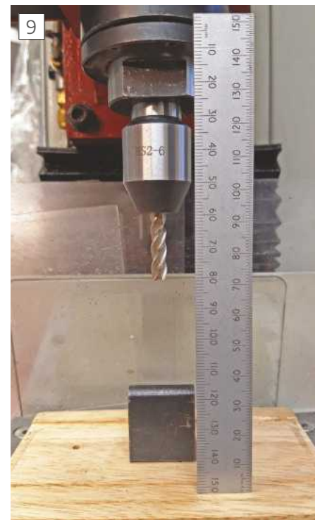
Tool height comparison. 2MT end mill holder. ➤
