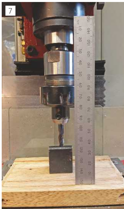
Tool height comparison. New holder.
