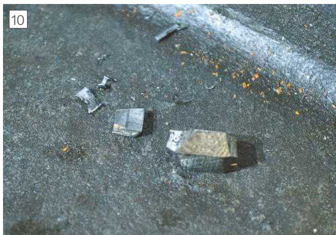
After a few strokes there was a bang and the tool bit shattered as it dug in!
