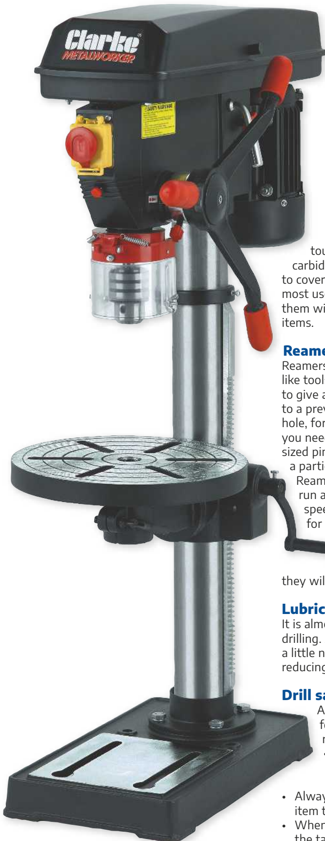
This large Clarke bench drill has sixteen speeds and an MT2 spindle.
