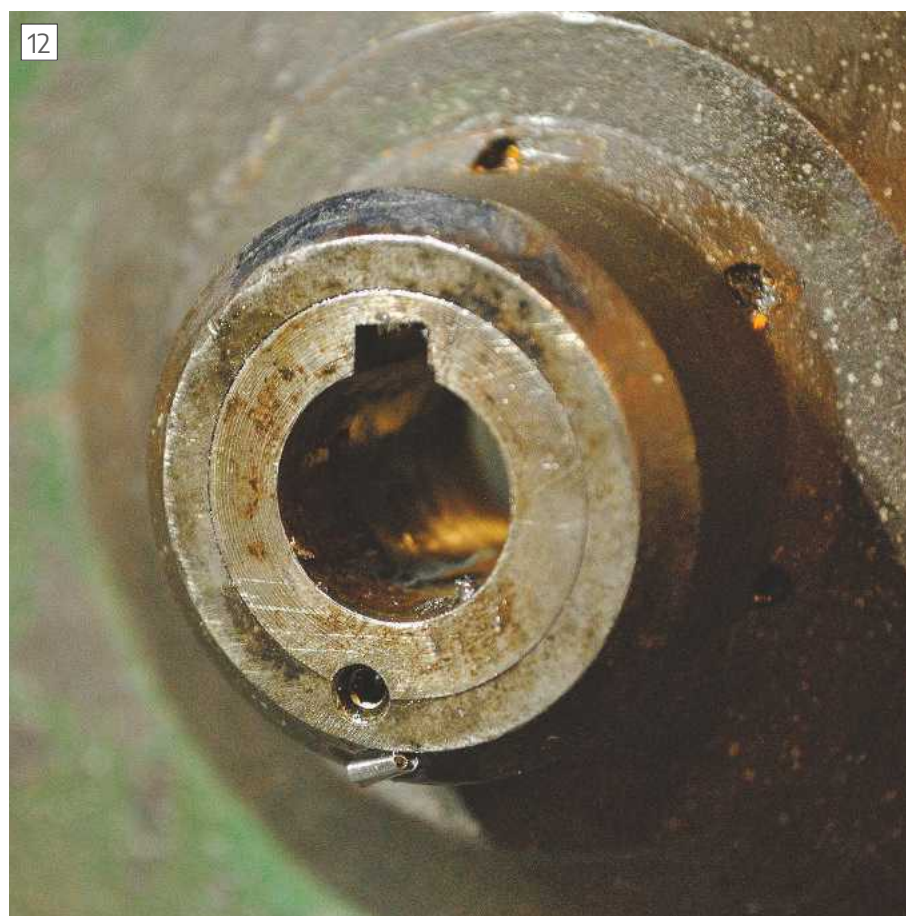
The finished keyway, not bad for first attempt.
