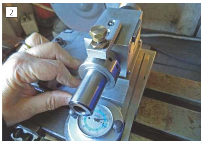
Setting the fixture to required angle
