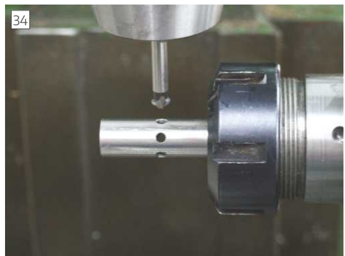
34 Countersinking the light apertures.
