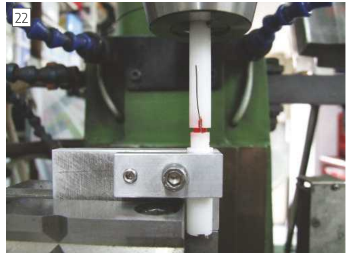
Fitting the LED into the cartridge body - note the cathode wire alongside LED lens.
