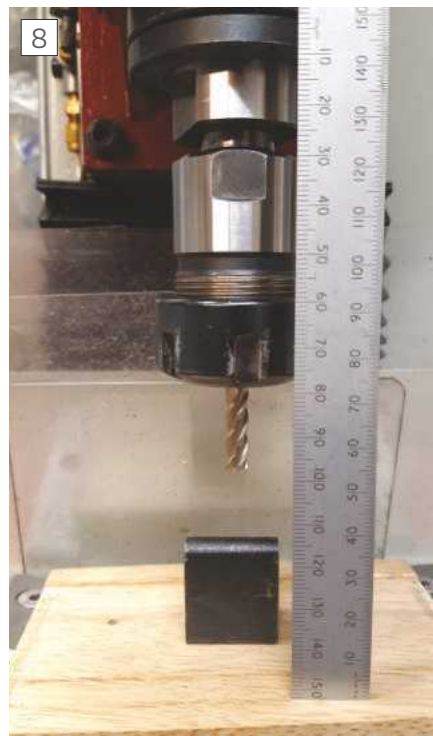
Tool height comparison. ER25 collet.
