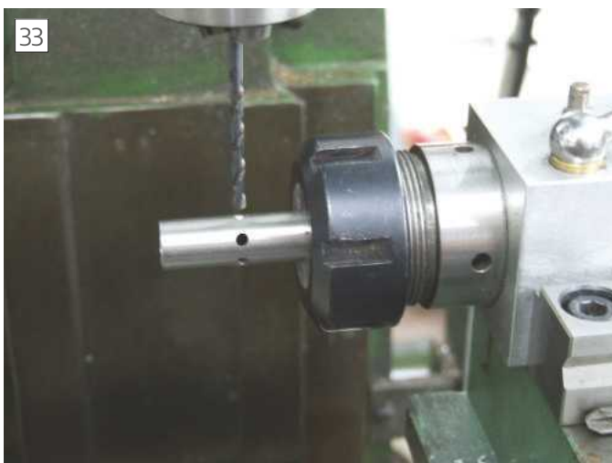
33 Drilling the last of six light apertures in the body.
