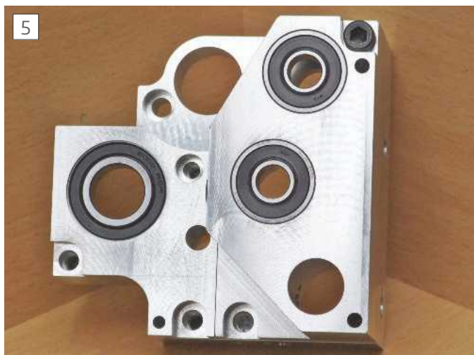
5 Main body with clutch gearbox cover fitted.
