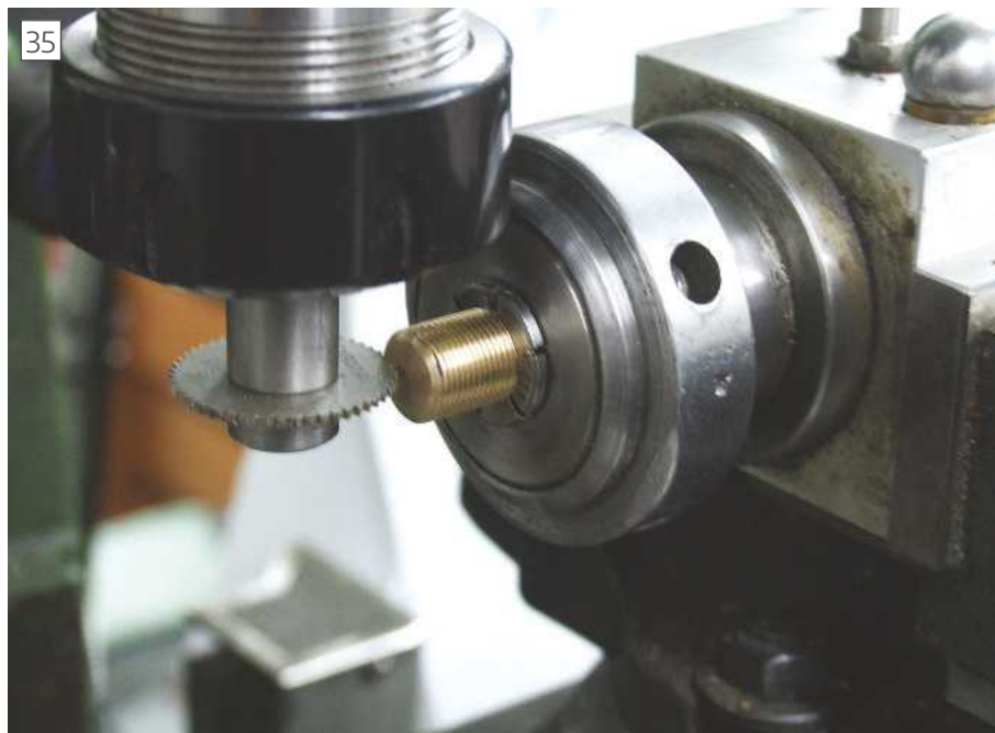
Cutting the screwdriver slot in the end cap.
