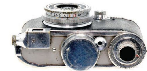
View from the top, showing the viewfinder swivelled 90° and the unusually complex frame counter
