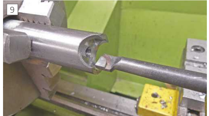
Boring the internal recess.
