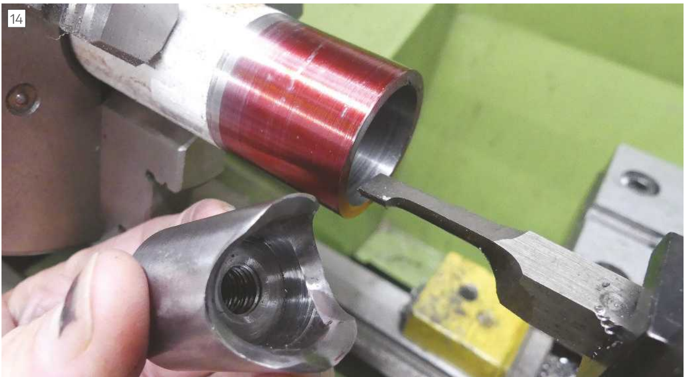
Turning the die on the lathe.
