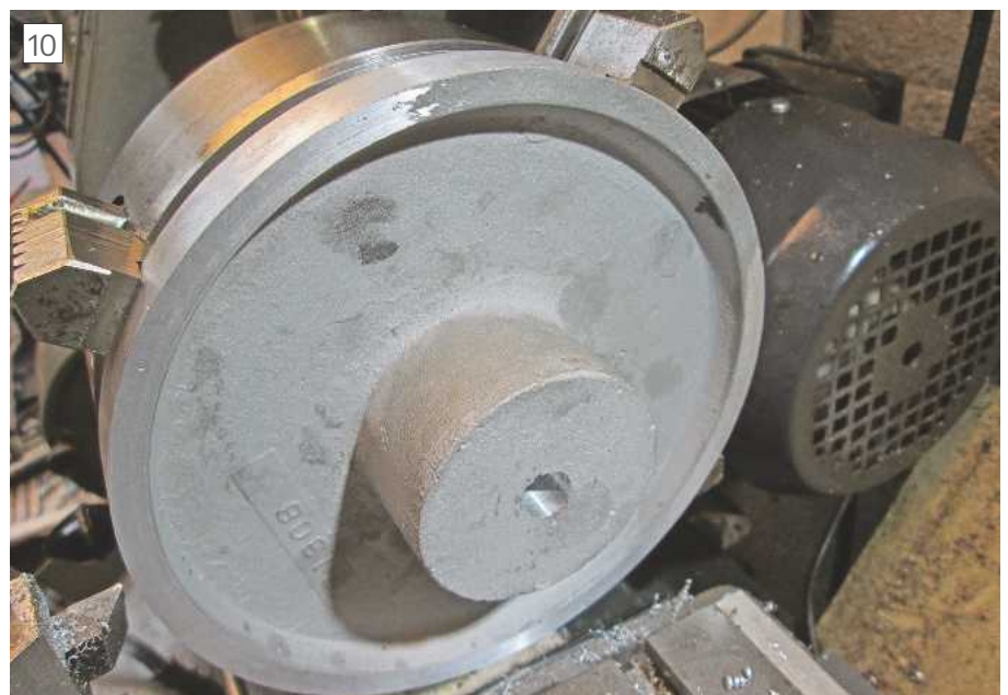
Casting reversed and held in the 4 jaw chuck ready for final machining
