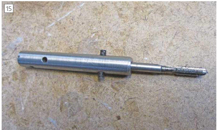
The tapping drill extension modified to take the tap at its other end
