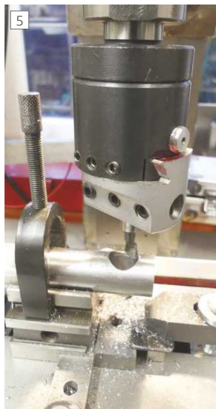
Boring head to enlarge the transverse hole.
