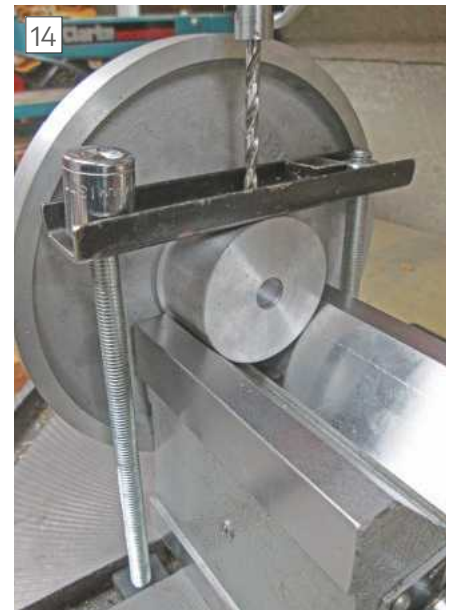
Cross drilling the boss utilising the extension
