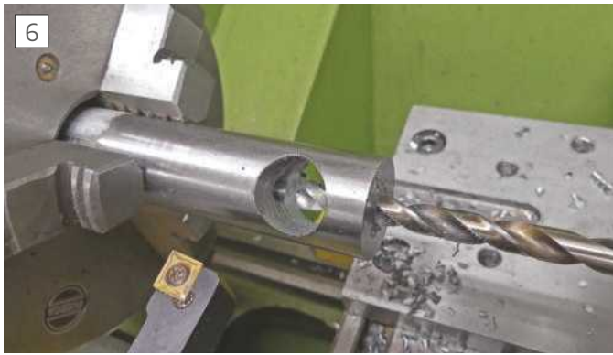
Drilling M8 tapping hole on the lathe.
