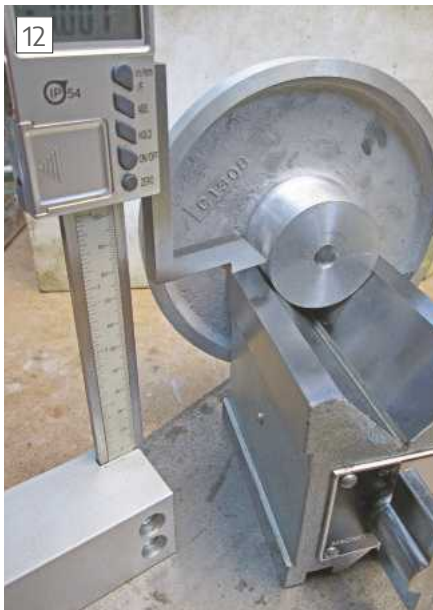
Marking out in readiness for cross drilling the boss
