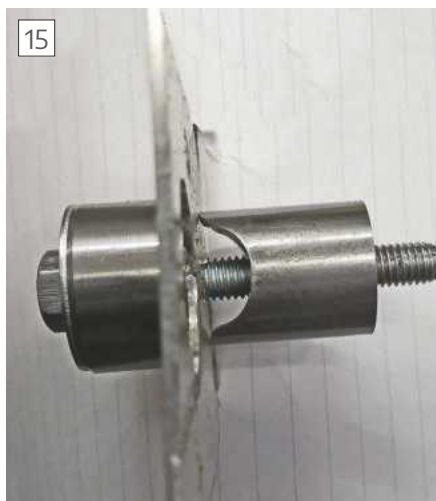
Punching 1.5mm aluminium.
