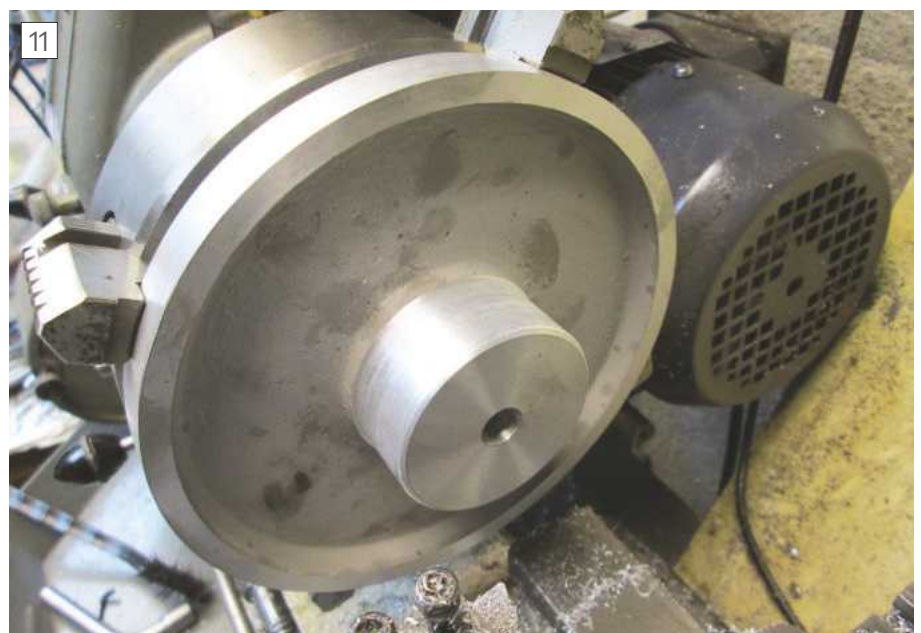
Lathe work completed on the disc casting
