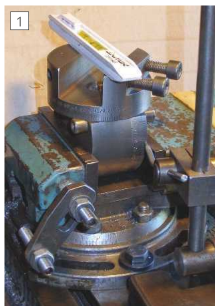
Setting the vice level in a machine vice.
