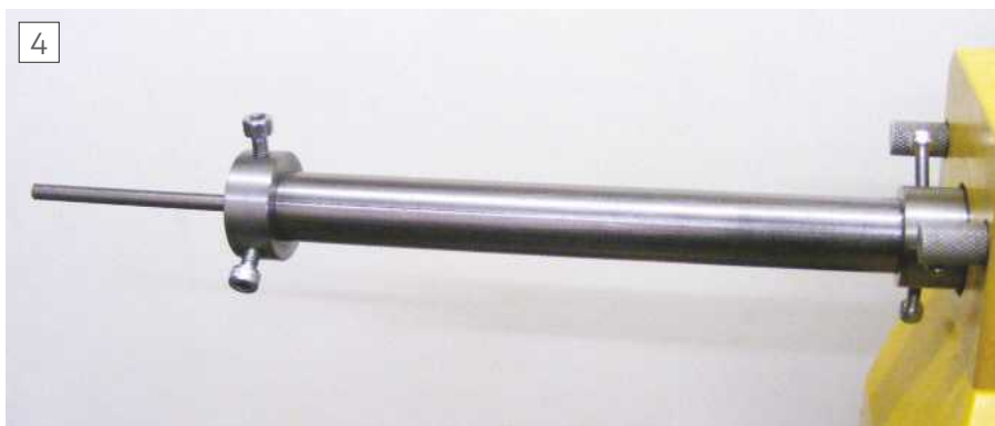
The tube installed in the lathe spindle.
