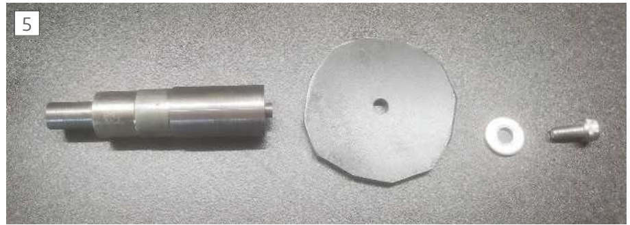
Retaining plate mandrel set up
