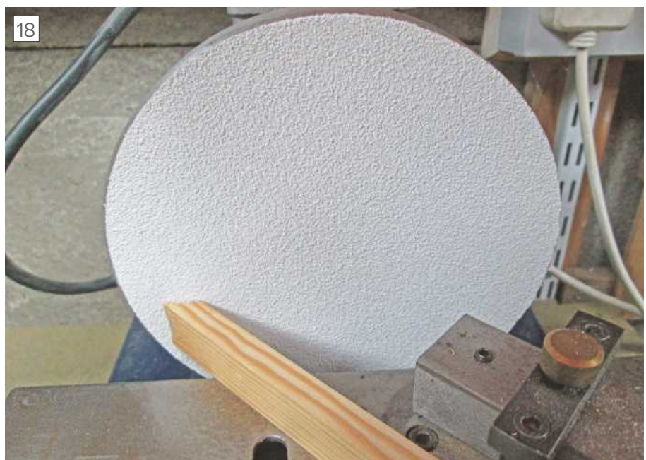
Abrasive paper fitted to disc and ready to go
