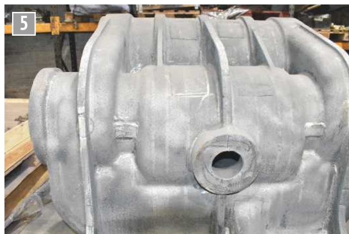
Detail of the outside surface of the casting which has picked up the sealing tape marks of the pattern.
