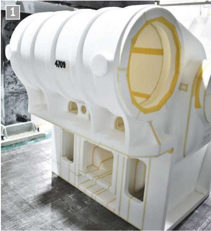
1 A view of the polystyrene pattern before being used in the mould.
