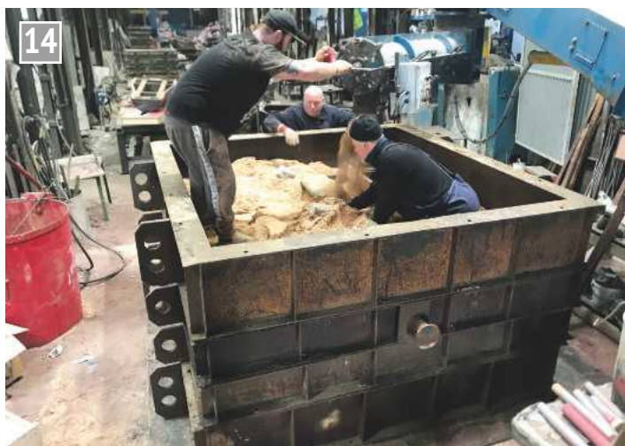
Packing the sand round the pattern (photo supplied by the Boro Foundry).
