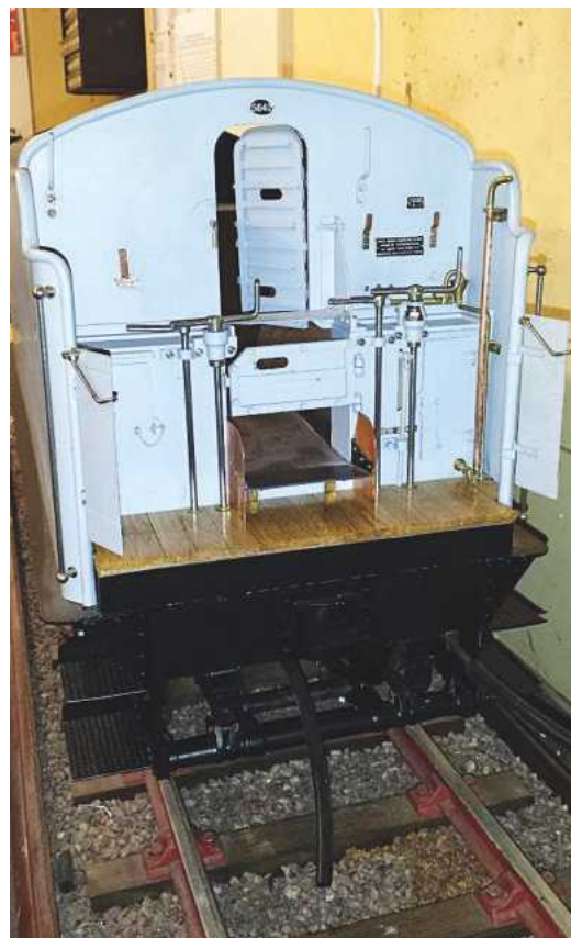
12. A close up of the front. There's been a few changes here. I have finally redone the wooden planking. New items include a lamp bracket, seen on the left side as viewed, handle for locking the coal door closed, safety hoops that sit over the cab/tender doors, the two side shields fitted to the coal scuttle, the water gauge has had some of its holes filled to follow the prototype closer and there is now the water tap that is below the right hand (as seen) locker.
