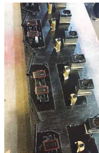
5. Next were the axlebox covers - these were done again using the pen but this time using a template as the guide.
