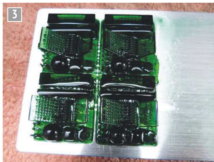
Only four of the test pieces came out, the others were stuck to the vat floor.
