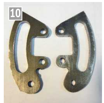
The right-hand link finished and the left-hand after machining. As can be seen the ends of the slots have not been finished yet - a job for a rainy day.
