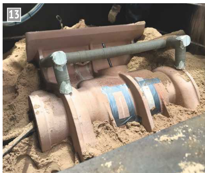
The pattern installed in the mould box awaiting additional sand (photo supplied by the Boro Foundry).
