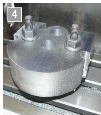
Radii machined and the two 0.75mm holes bored and two small holes for corner fillets.
