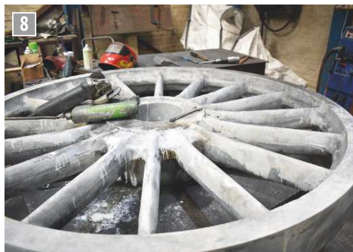
One of the bogie wheels for the new LNER P2 locomotive being prepared for ultrasonic testing.
