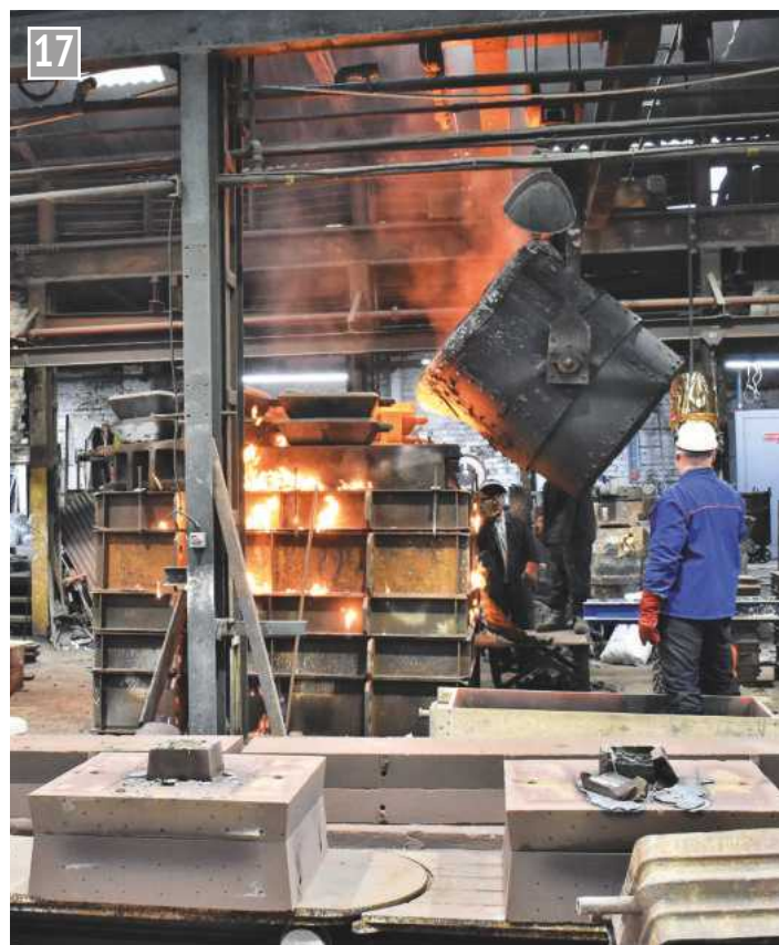
The escaping gases ignite around the mould box.
