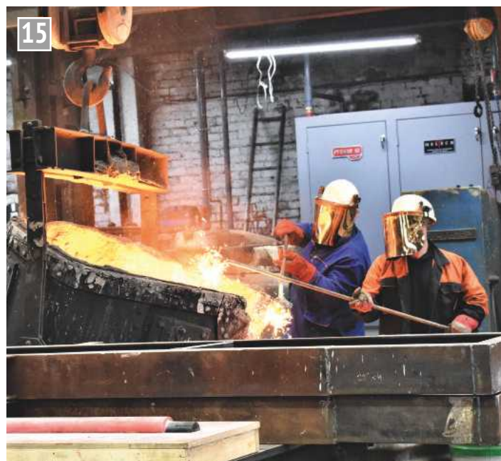
Removing slag from the ladle before pouring into the mould.
