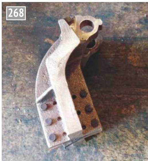
4. This picture shows the trunnion so far. Note that I have worked the outside profile a little using files and a belt sander to bring it closer to the drawing. I could have done more here to centralise the bearing hole but decided to do the two bearings first and use them as a final guide to the outside profile.
