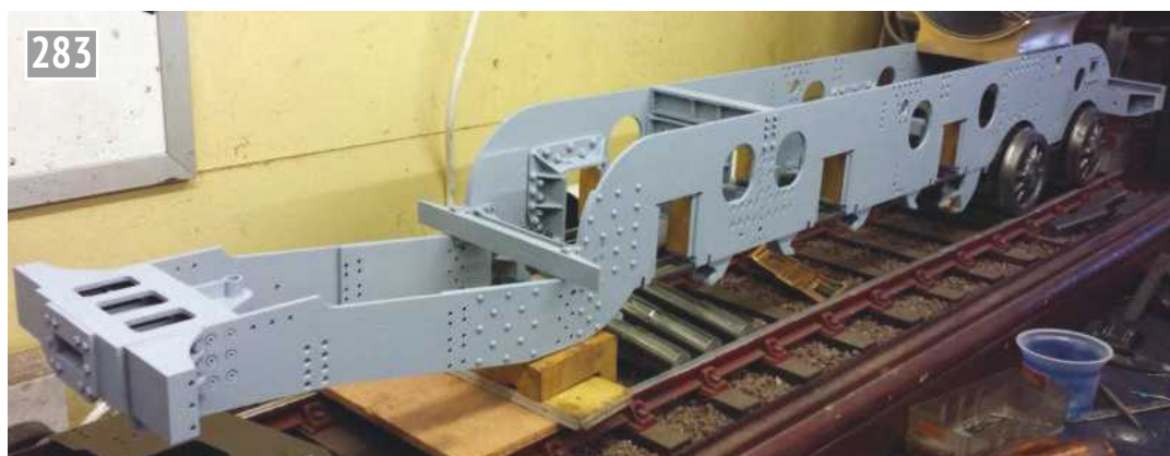
19. There was then a marathon session (I seem to have a lot of those), stripping everything down, painting with Acid 8 and reassembling with small head bolts for scale. This took many hours but I think the end result speaks for itself.
