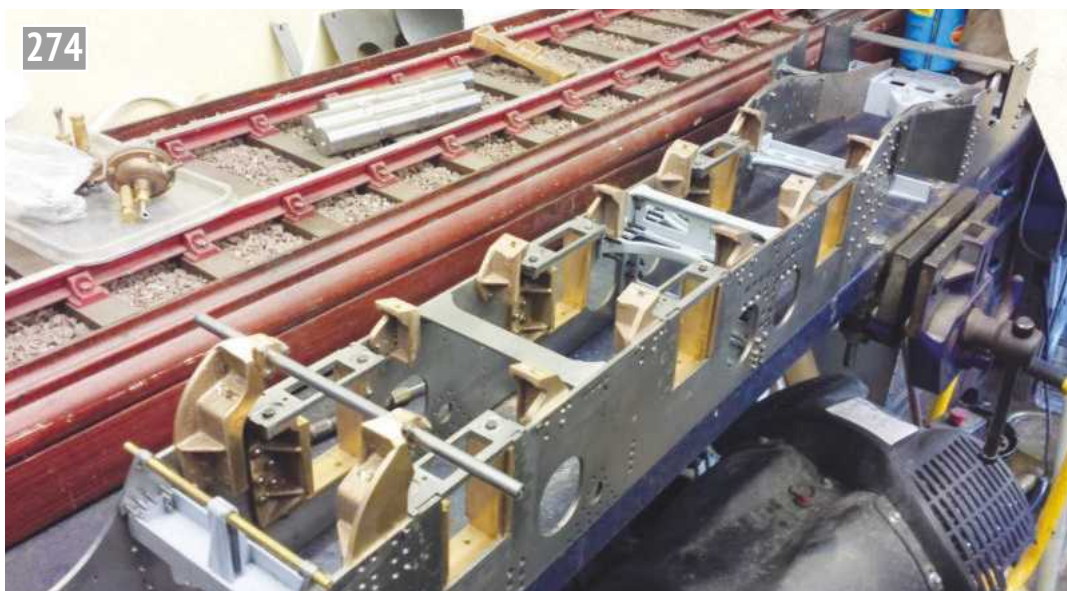
10. And here we have the chassis with brake trunnions and spring hangers in place. Note the brake shaft steel bar is only a temporary item for alignment which I'm happy to report is good, as is the brake cylinder alignment. There's still a lot of riveting to be done here but it was getting there slowly.
