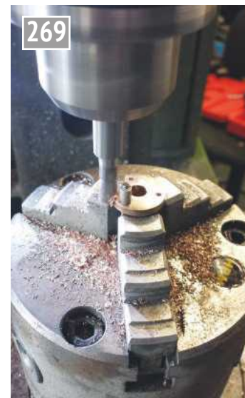
5. After turning the bearings they were transferred to the rotary table for drilling the three securing holes at 120 degree spacing. The unwanted material between the spigots was then machined away. I cheated here. I didn't see a reason for setting up an index but also didn't want to rely on the dial markings alone so went for using a spacer positioned in each hole and just machined up to the spacer - not the engineer's way but good enough for the eye in a non-critical situation.
