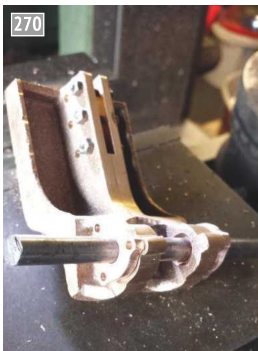
6. Here I am checking on how things are fitting together - as can be seen I still had a lot more work to do on the trunnion bearing housings before they matched the bearing profile. The mounting holes were then transferred onto the bearing housings.
