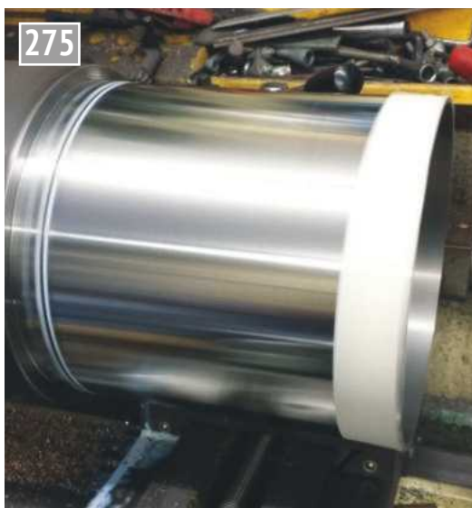
11. Here is the smokebox tube being parted off. The white tape seen was to reduce chatter.
