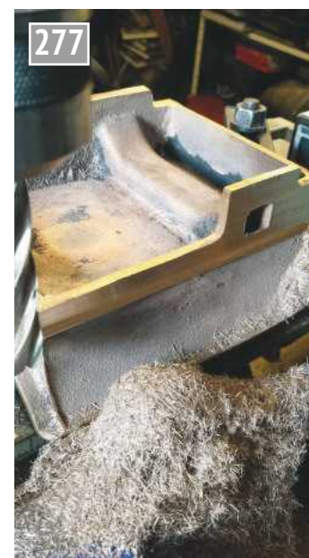
13. Once lined up, the saddle casting was machined roughly to size. The casting has a \frac{1}{8} inch overhang to sit along the top of the frames, which is cut 1\frac{1}{4} inches from the bottom edge of the exhaust port tabs (top as seen in the picture) and as a check it also needed to be \frac{5}{16} inch from the rest of the saddle base. Here the casting proved to be very good - both measurements were spot on. It was also very reassuring to find that when machined both sides were identical. proving that the saddle was sitting level.
