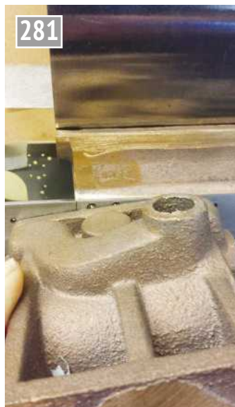
17. Here, I am holding the cylinder roughly in position to check that the steam/exhaust openings don't foul the saddle's rear face. As can be seen it's close, but then it is on the drawing and if I moved the saddle forward to match the exhaust positions this would be even closer, perhaps fouling the rear of the saddle with its \frac{1}{8} inch thickness. It all looks good though so I left the saddle as it was. I tried to check all possibilities and think way ahead but I had to decide and that I now did. Later, much later I realised where the \frac{1}{8} inch error may have come from - there's a \frac{1}{8} inch difference in mounting position between the two bogie types. Perhaps Don didn't allow for this on his drawing?
