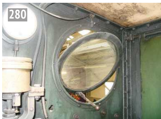
Showing how the cab window is hinged for opening.
