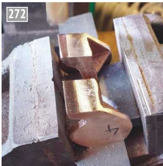
8. Once the ten spring hangers had been drilled they were again placed back in the tilting vice in pairs to have the holes drilled.
