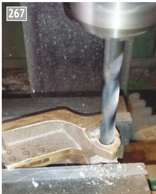
3. The bearing journal faces were then machined flat and the holes drilled ready to accept the brake shaft bearings.
