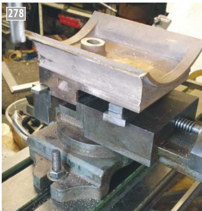
14. Next the casting was up-righted and the side and front edges machined square, removing all of the flash in the process. This, as can be seen, only just fitted in the machine vice. With both sides done I had just enough movement on the table to do the front edge, the rear was cast without any flashing so easy to finish with a file.
