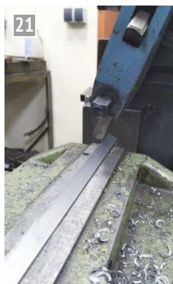
Using the shaper to form the dovetail guide rails.
