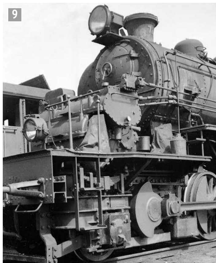
Turbine housing on front of TGOJ locomotive designed by Alf Lysholm. (Image from https://digitaltmuseum.se )
