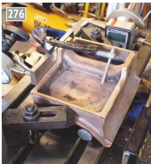
12. The saddle casting lined up on the milling machine table, ready for machining.
