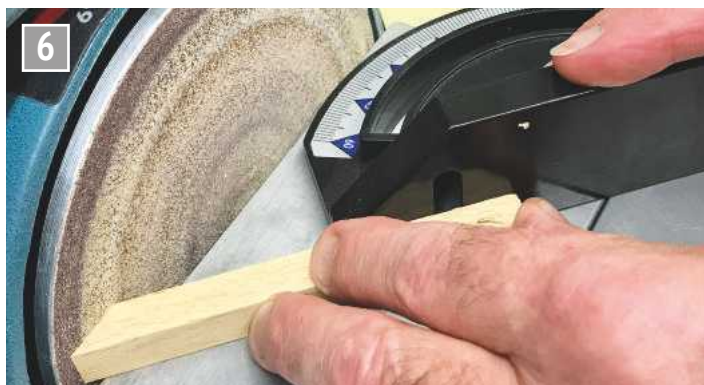
Wood strip shaped to 45-degree end.
