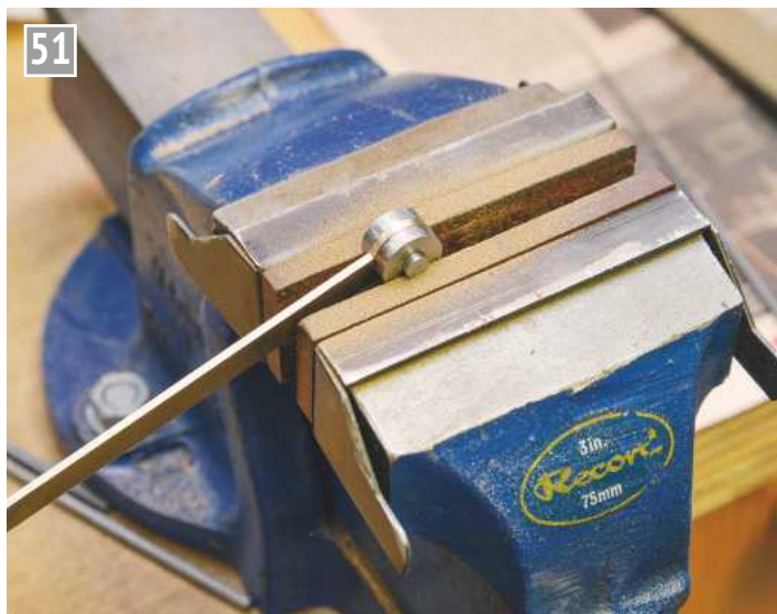
Using a filing button to form the rounded end.
