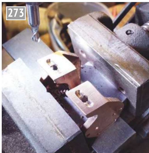
9. The recessed grooves for the shock absorbers to locate were also cut at this stage.
