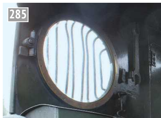
The rear windows are hinged differently from the front windows.
