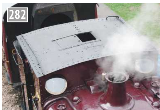
The hatch on the early cabs opens sideways.
