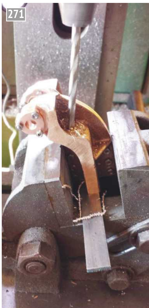
7. The last machining job for the trunnion was to drill the holes for the spring hanger bolts to pass through, which were drilled at 15 degrees to the vertical. This was a job for the tilting vice and the digital angle scales. This just left the final profiling of the brake trunnion around the bearing housing to finish.
