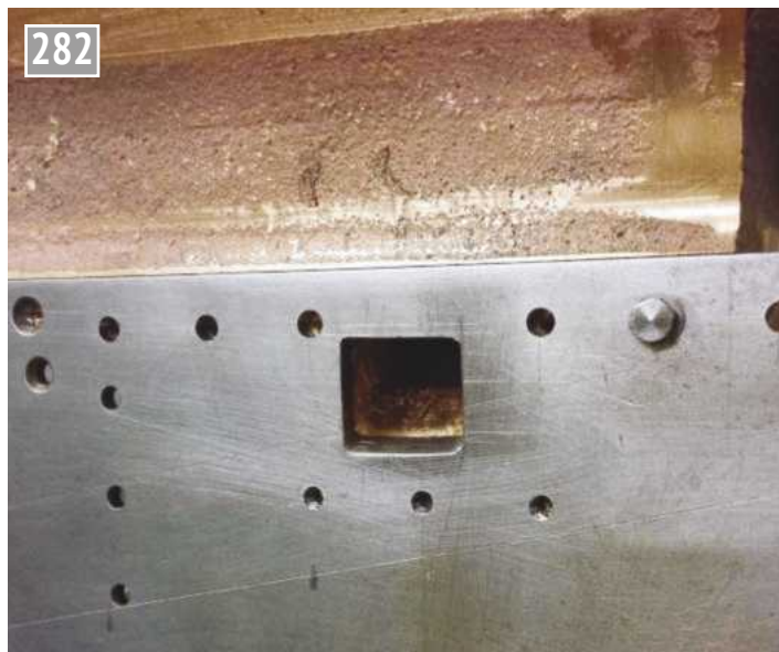
18. Finally, I bit the bullet and cut some metal, only on one side so far but here was the result. I do like Don's design, love how the slot is angled to match the casting, which should help in the free flow of the exhaust gases. I've cleaned up the inside of the exhaust opening a bit but will do a little more - I need to make something up to reach in further as there's a flash line along the upper length of the tube between the two cylinders that needs removing.
