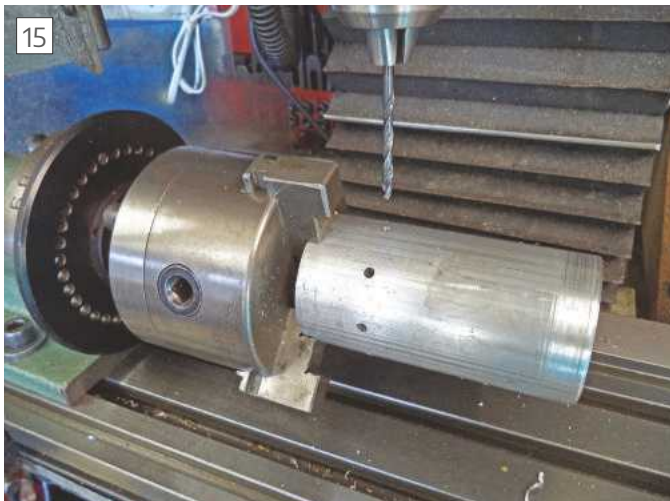
Drilling 4mm ventilation holes using spin indexer
