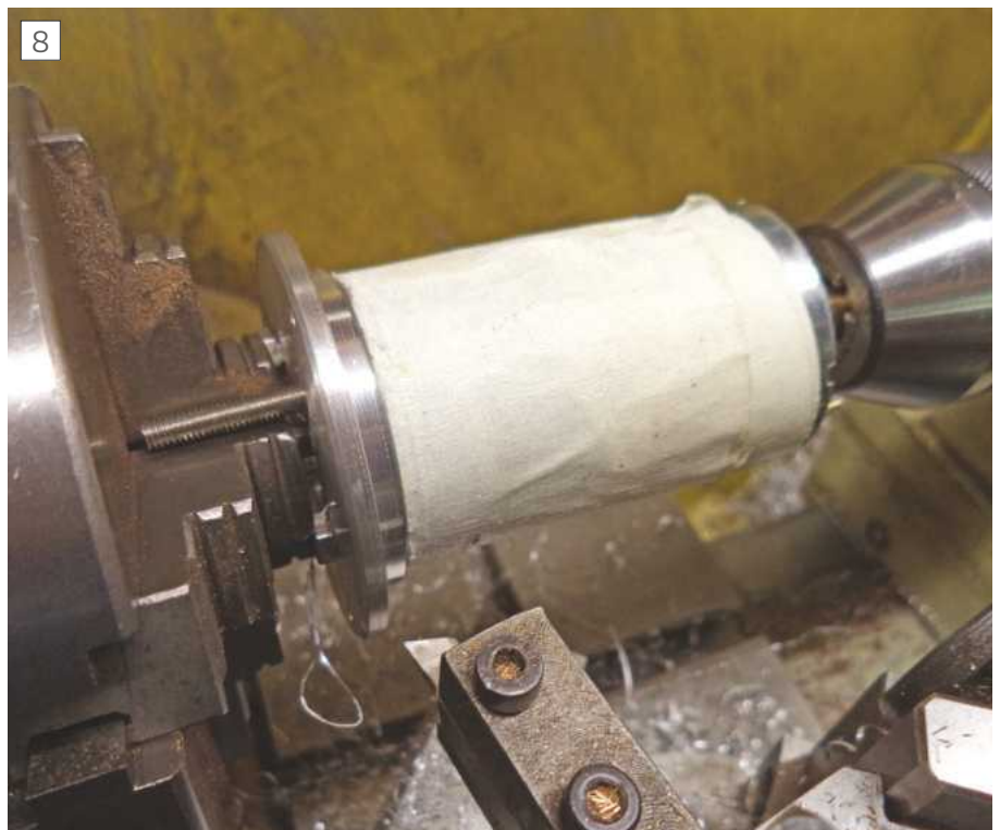
Machining end cap true to motor spindle
