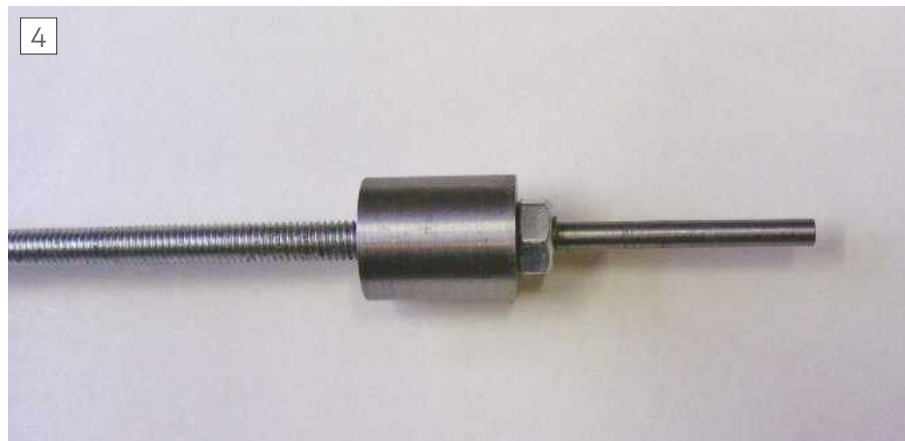
Showing the magnetic probe screwed into the stop.
