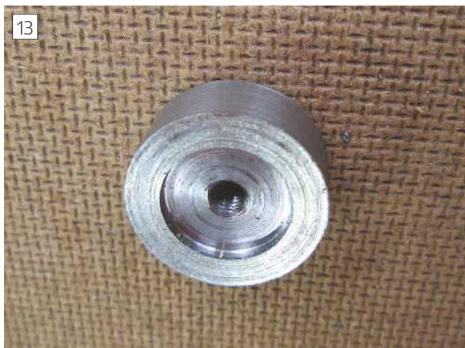
Cup to take load from screw and protect vice jaw
