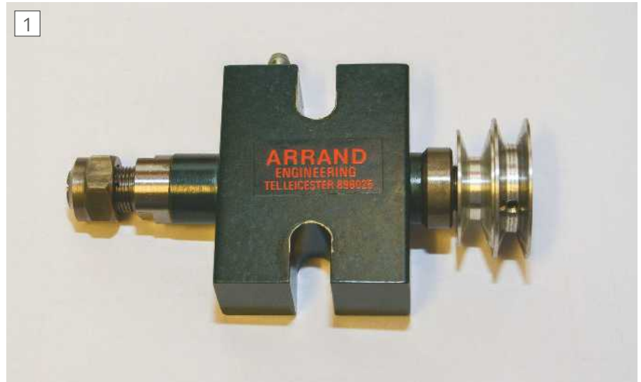
My original Light Milling Spindle made by Arrand Engineering. The design of this spindle appears to have been based on that described by J.W.E. Message in Model Engineer 28 February 1957, pp321-324.
