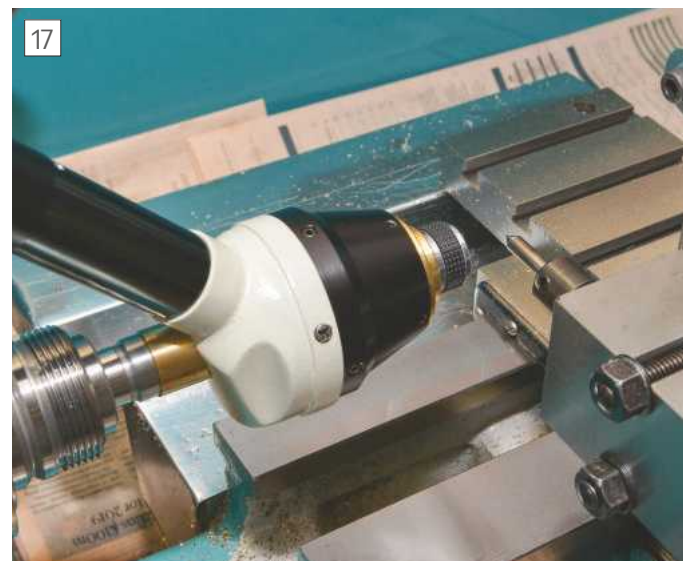
Checking the centre height with a microscope from the lathe mandrel. Easy but typically one does not want to remove the chuck with a turned part in order to set up the milling spindle.
