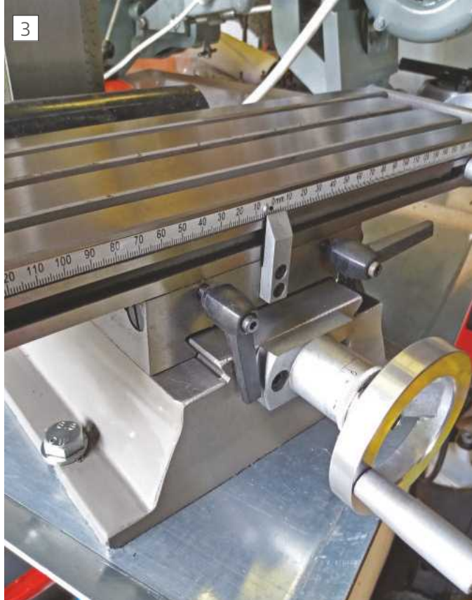
The handles can catch on the base casting.
