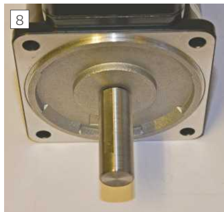
It would clearly be preferable to buy a motor with a plain shaft but the problem is solved using by turning and boring a sleeve extension secured with Araldite. Remember to mill a small flat along the sleeve for the pulley grub screws.
