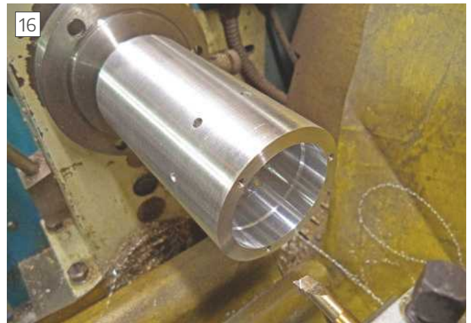
Assembled Body and Arbour in lathe head stock for finishing the 45mm diameter for a true close fit on end cap
