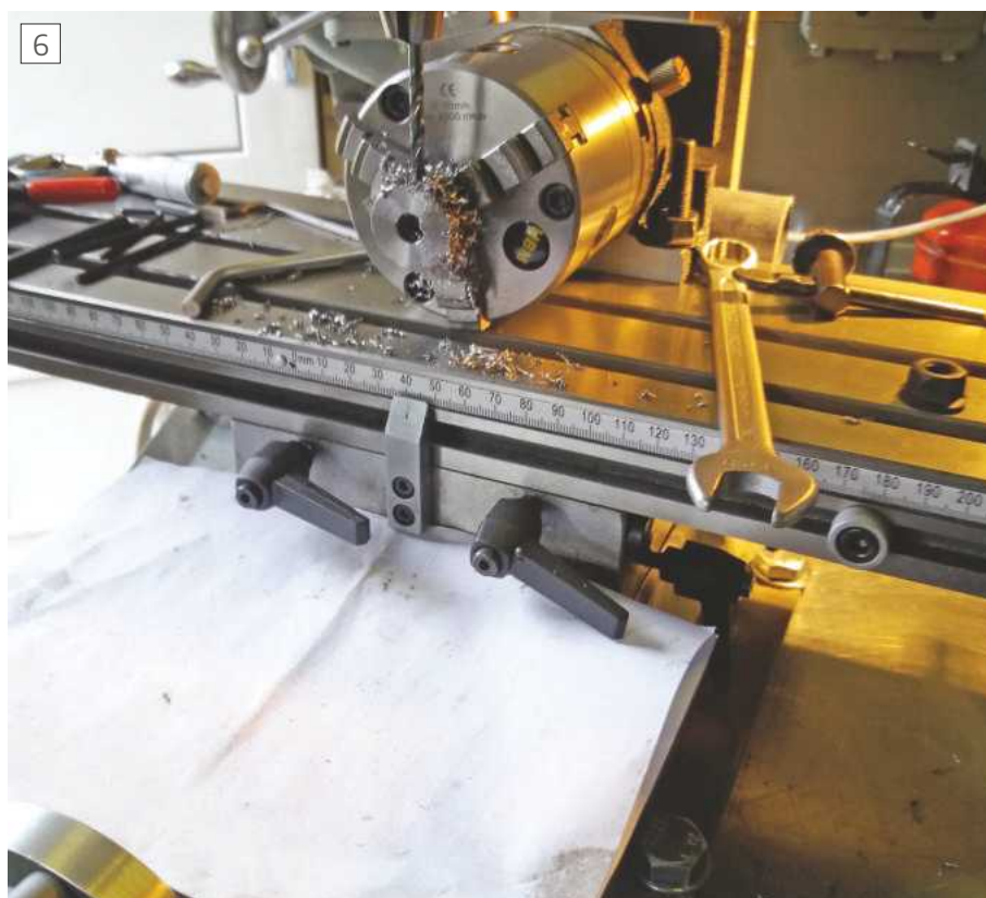
Trial with a sheet of kitchen roll shows how a rubber cover can fill the gap.
