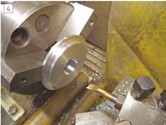
Machining end cap using soft jaws
