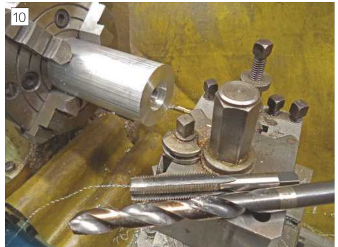
Drilling tapping and boring to take M3 Arbour
