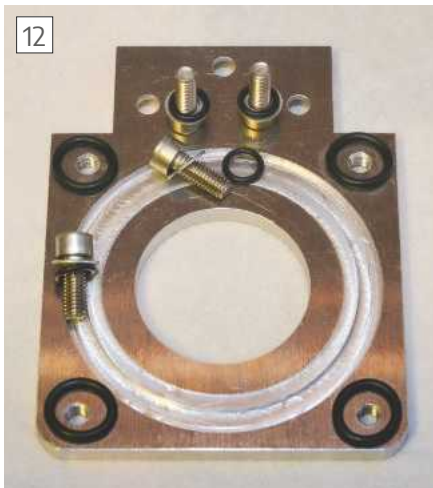
Rubber O rings mounted between the motor and motor mounting plate will reduce noise as they form a resilient mount.
