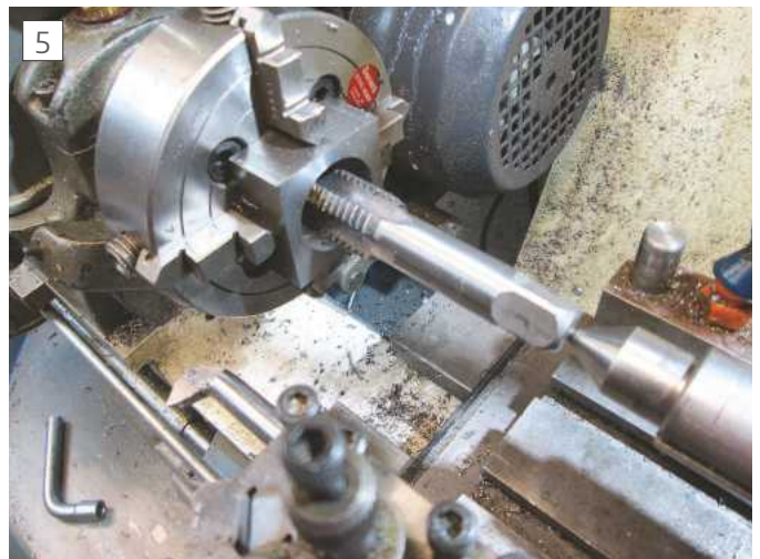
5 Starting the tap whilst work still mounted on the lathe
