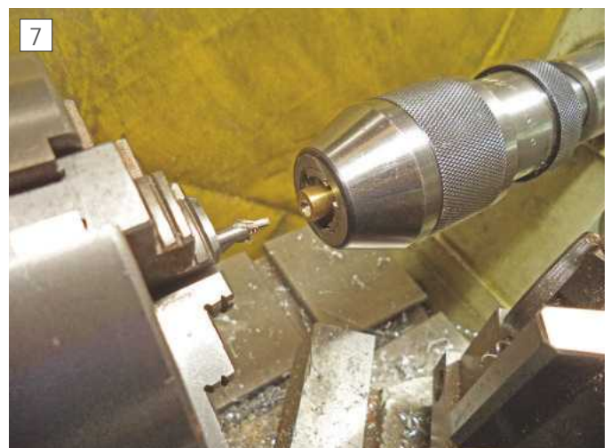
Making the female centre with centre drill held in lathe chuck
