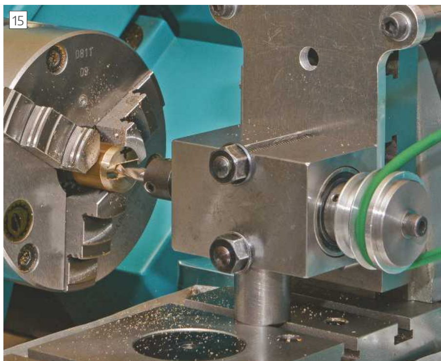
Checking the accuracy of the spacer cylinder by milling a slot in a scrap of faced and skimmed brass.
