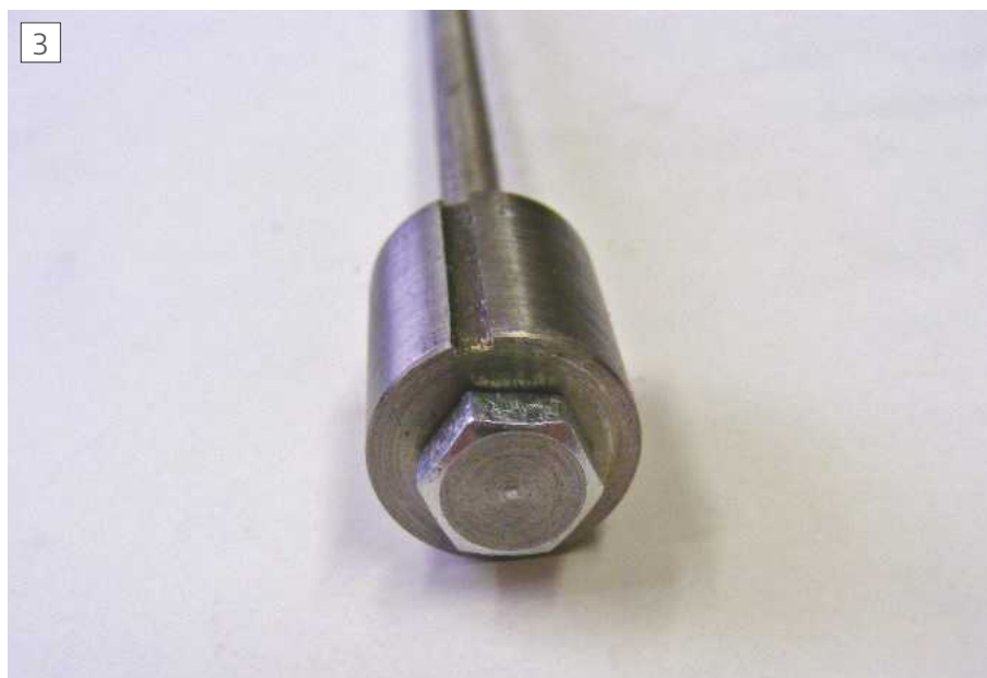
Showing a hex head screw blanking the hole in the stop.
