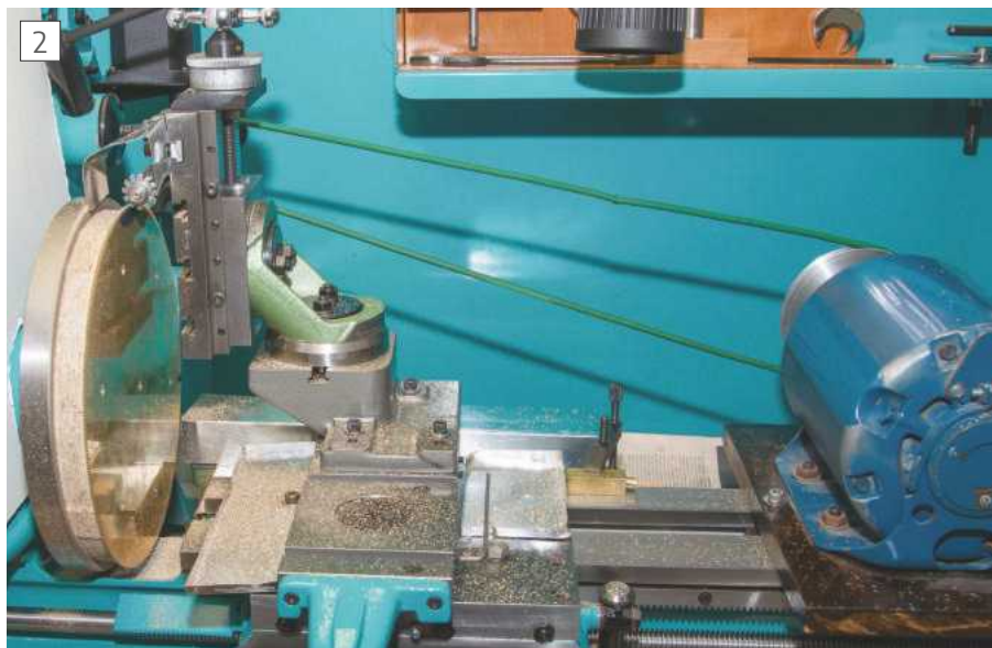
Cutting a 400 tooth clock wheel with the motor strapped to one end of the bed and the Light Milling Spindle mounted on a vertical slide with a raising block. Note the long drive belt, the brass block and clamp used as a stop on the lathe bed, and the card shielding to stop the chippings going everywhere!
