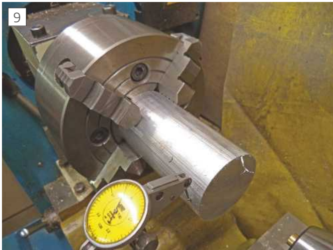
Clocking body true in four jaw
