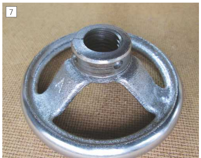
7 Drilled locating sockets for grub screw ends
