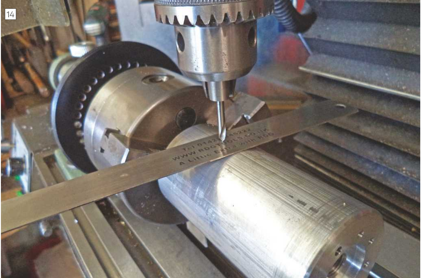
Using the old ruler trick to align mill on centre
