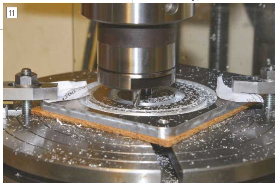
Below: Milling out the centre of the motor mounting plate.
