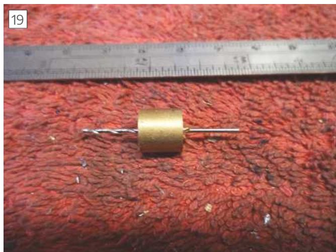
1mm drill through a 10mm thick piece of brass
