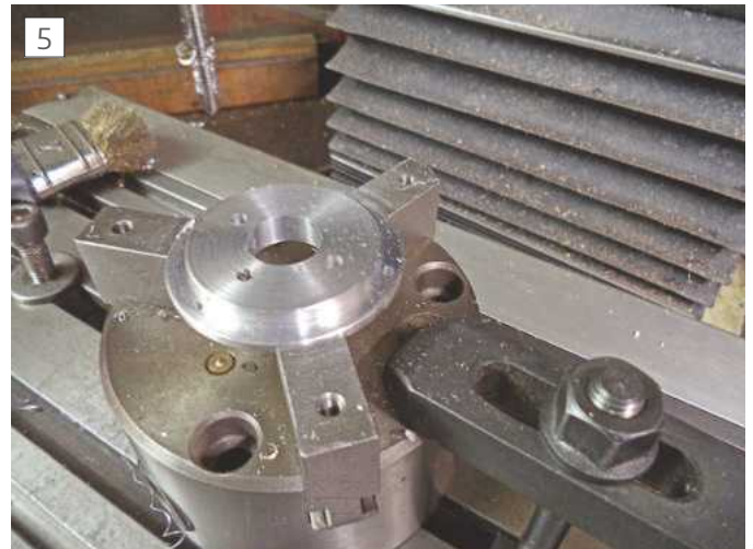
Drilling the end cap using PCD function
