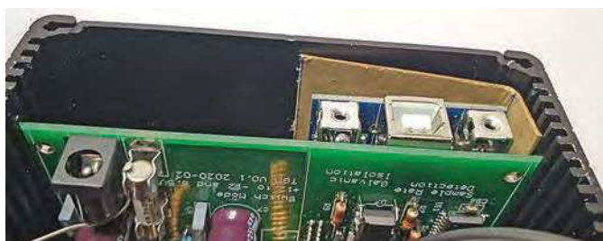
The pre-assembled USB Streamer PCB plugs into the two 12-pin header sockets on the underside of the PCB.
