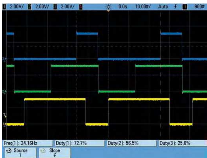
Scope 2: this demonstrates using the PCA9685 module to produce three different PWM waveforms with different rise and fall positions, with each duty cycle being fully adjustable. The main restriction is that the repetition frequency of all outputs must be the same.
