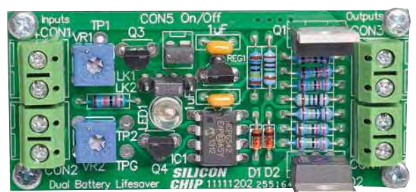
Fig.2: the PCB has been kept as small as possible while still being easy to build, handling a decent amount of current and providing for easy wire attachment and mounting. Assembly is straightforward but make sure that the IC, terminal blocks, MOSFETs, diodes and LED are correctly orientated. Use the component overlay above in conjunction with the same-size photo at right to assist you in component placement. Note that the values of RL1, RL2, RU1 and RU2 need to be chosen from the table overleaf.
