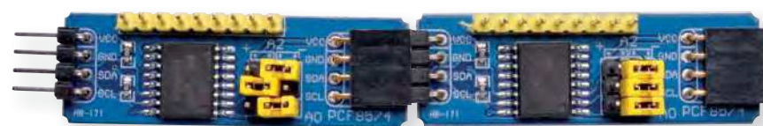
The PCF8574 modules are designed to be stacked end-on-end, meaning that it's trivial to connect multiple such modules to a single microcontroller. Note that the address jumpers are set here to give each module a different I 2 C bus address, to avoid conflicts.
