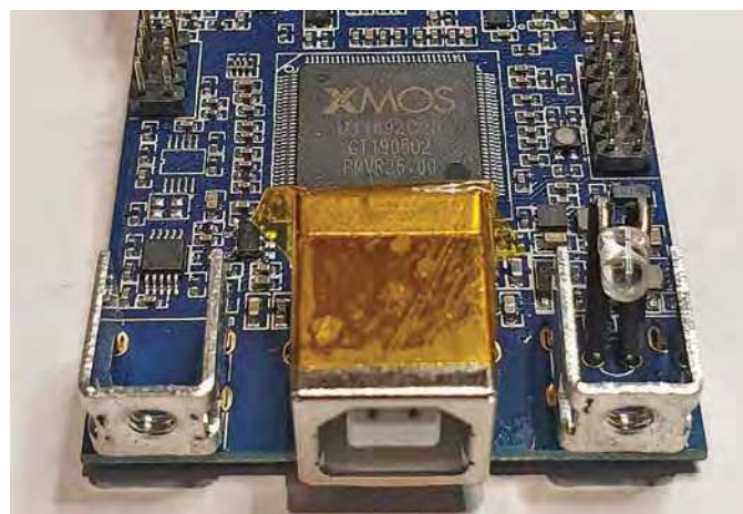
A section of Kapton tape on the USB socket ensures it can't short to any components on the main PCB.
