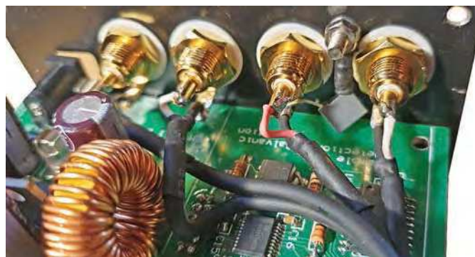
A 10nF capacitor between the input grounds and rear panel earth lug minimises hum pickup.
