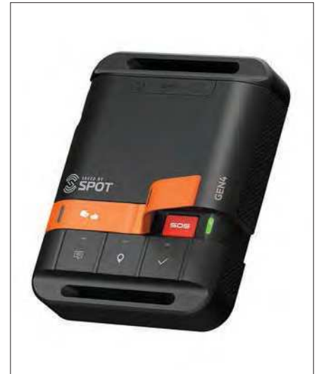
The SPOT Gen4 is a portable messenger / SOS pager that summons help via the Globalstar LEO satellite network. Flexible tariffs are available for users.
