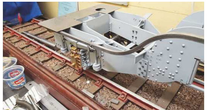
6. And here we have the rear section. The outriggers when fitted will sit in the 'S' bend. During construction I kept a close eye on the valance position to ensure that it was matching up to where the rivets sit along the running boards. In the picture the valance disappears under the cab floor and this needs to align so that the rivets/screws that run along the cab floor are central to the top of the valance plate.
