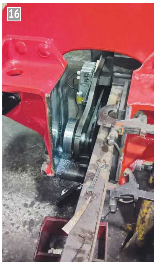
Bogie hornguides being machined to correct the alignment viewed from between the frames.
