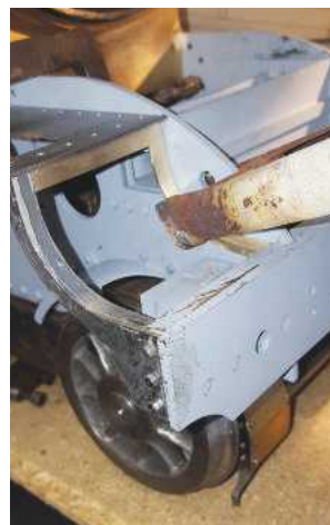
12. I haven't bolted the part in place here yet as I'll need to remove the valance/boards first to drill the holes but I will show how the part fits as an aid for anyone else at a similar stage on their own builds. Mind you, I'm sure that this can be done a number of different ways - this is just my chosen method.
