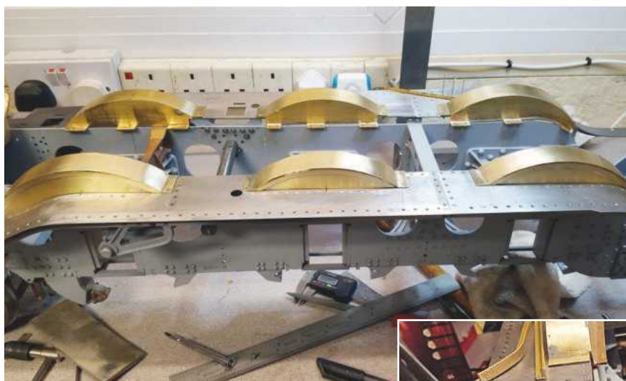
16. This picture shows the rear brackets ready for fitting to their respective supports. Note that I have already marked the other side ready for cutting. I need to take everything apart again to fit the right-angled supports and so will probably do all of the supports together once all the other parts involved have been done. The top inner corner of the rear splasher needs to be cut back at an angle to allow clearance of the boiler and its cladding. Since this is a very close fit with next to no gap I'll leave this until the boiler has been placed on the frames and checked for clearance. The driver and leading splashers aren't as close to the boiler and thus do not need cutting back.
