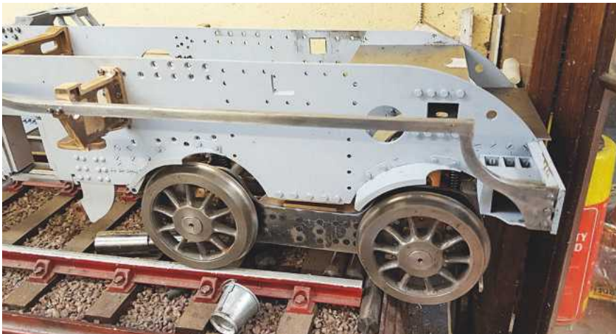
2. This picture shows the laser cut parts assembled, I did the curved top sections by hand using whatever radius bar was nearby to help shape the parts to match the valance profiles.
