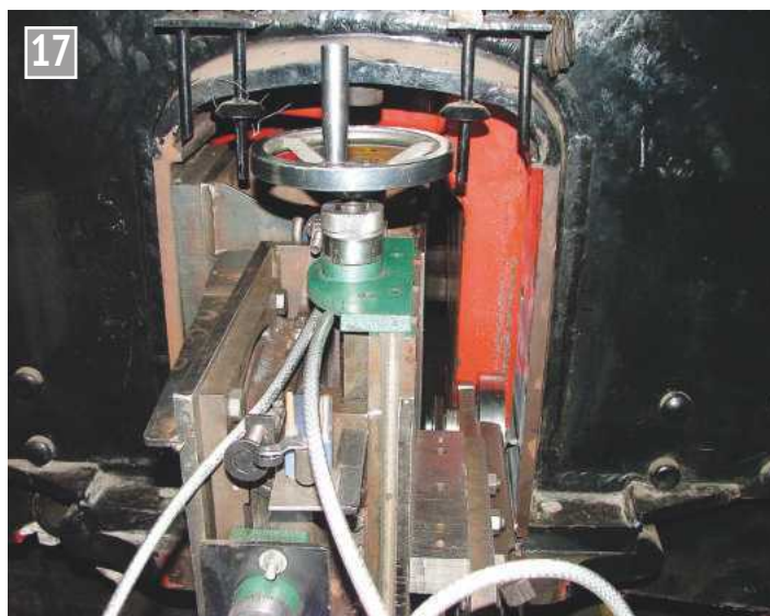
Locomotive hornguides being machined. The cutting tool can be seen lower right, with the swarf being sprayed against the valve gear oil bath behind it. In the centre of the photograph one of the limit switches can be seen.
