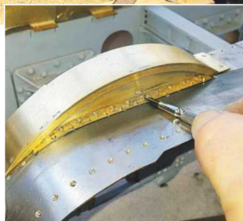
20. Continuing on with the rear splasher exterior brackets. I had to reshape a new section of brass right angle as naturally the holes for the previously used 12BA screws were too big for the now preferred 14BA items. I drilled the countersunk holes, curved the angle and fitted the screws/nuts, then soft soldered them in place with the threads, then cut down.
