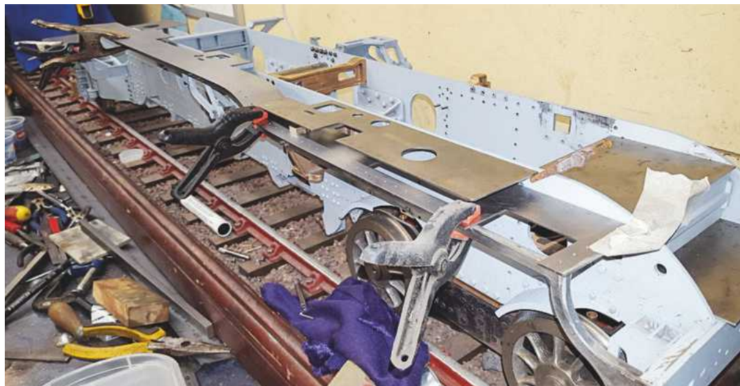
8. Once the bracket was back in position I laid out the running board sections and the long valve travel cover to see how things were going. The rivet holes are running down the valance nicely so I know that these parts will all go together as they should. The front edge of the running board matches the inner section for overhang so the extra length of the boards to allow for the curves is spot on.
