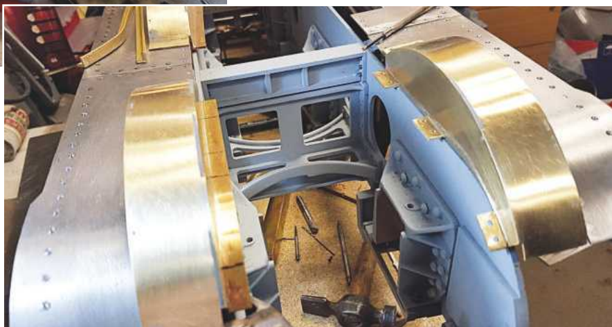
15. All six splashers have now been fabricated, the bulk with silver solder with the front trims attached with soft solder. I still have a lot of work to do here to complete this stage, more than I imagined as the closeness of the parts makes drilling impossible without taking everything apart first. The trailing splasher is further advanced than the others as hopefully can be seen in the picture. The front lip has been trimmed to size, drilled and countersunk to accept the two 10BA screws that secure it to the running board. The rear lower edge of the face trim has been cut to fit the curve of the running board as it slopes back, the back supports have been cut and drilled to accept the 8BA bolts and the main support that runs under the board has been riveted in place using 1/16 inch alloy countersunk rivets and bolted to the splasher with 8BA bolts.
