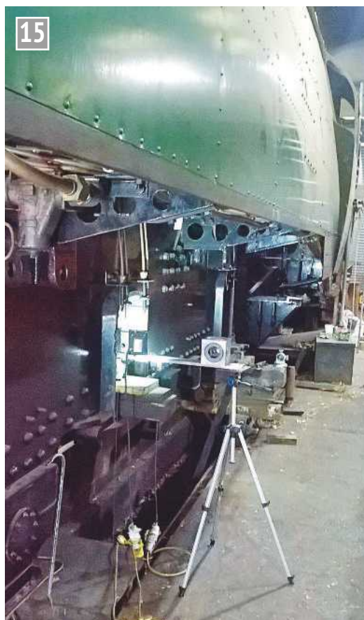
The optical prism is set at right angles to the axis of the locomotive and sighted through a telescope mounted on the cylinder.
