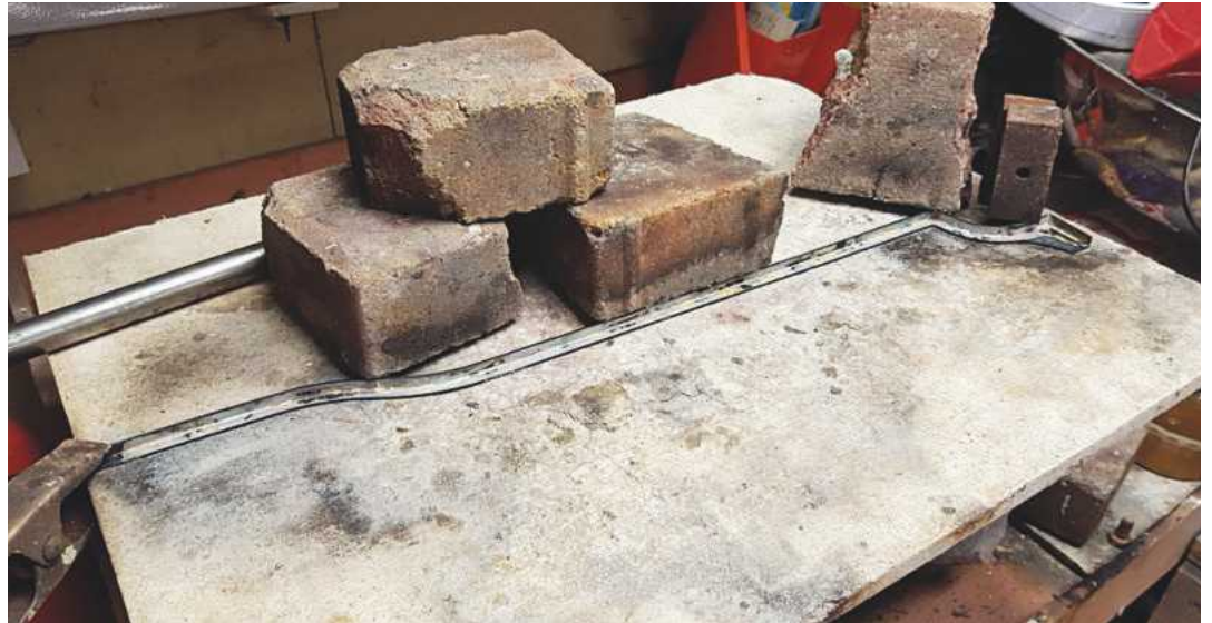
3. Next was to solder all the parts together. I was in two minds here whether to use soft or silver solder, silver being the best option for its strength and soft being the safe option in that these are very long (nearly 4 feet) delicate parts that could well twist/buckle if not very careful with the heat. I bit the bullet and went for silver solder. I had to do this in a number of steps due to the valances being far longer than my heating hearth, which made things even more tricky. As can be seen the valance is held at either end by a clip/weights and bricks were laid at intervals along the length to hold everything in place. All joints were given a good coating of flux and 0.75mm 55% solder was cut in strips and laid spaced out along the length. I wanted to be able to see the solder flow and also have easy access to the job so I first set the heating board up high on the hearth and I also heated the job from what really is the wrong side, that is heat to the side with the solder on. However, by being careful in heating, starting first from one end at the back just to get things going, it was a straight forward exercise to heat the job without too much heat directly on the solder as I moved along. To be extra safe I didn't allow the steel to heat too much where it was hanging over the edge of the board. Each section was left to cool and then the job was moved along the board to the next section.
