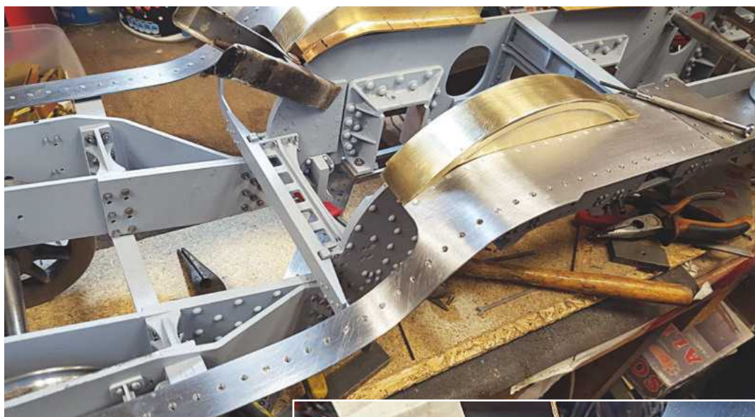
18. Here we have the long valve cover in place to check for position. I needed to shorten it a little along the rear edge as it was a little long. Later I'll fabricate the upright sections but for now it's just sitting on some steel stock so I can check all is as should be.
