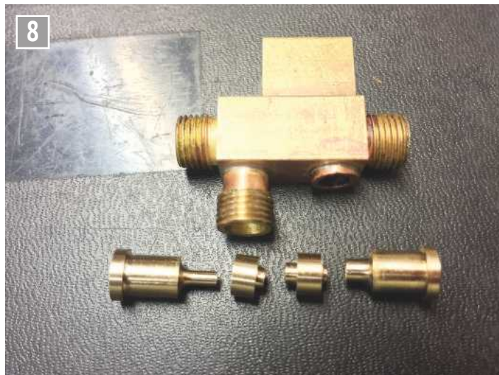
Injector, showing cones.
