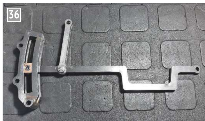
Lifting link assembly showing peened pin.
