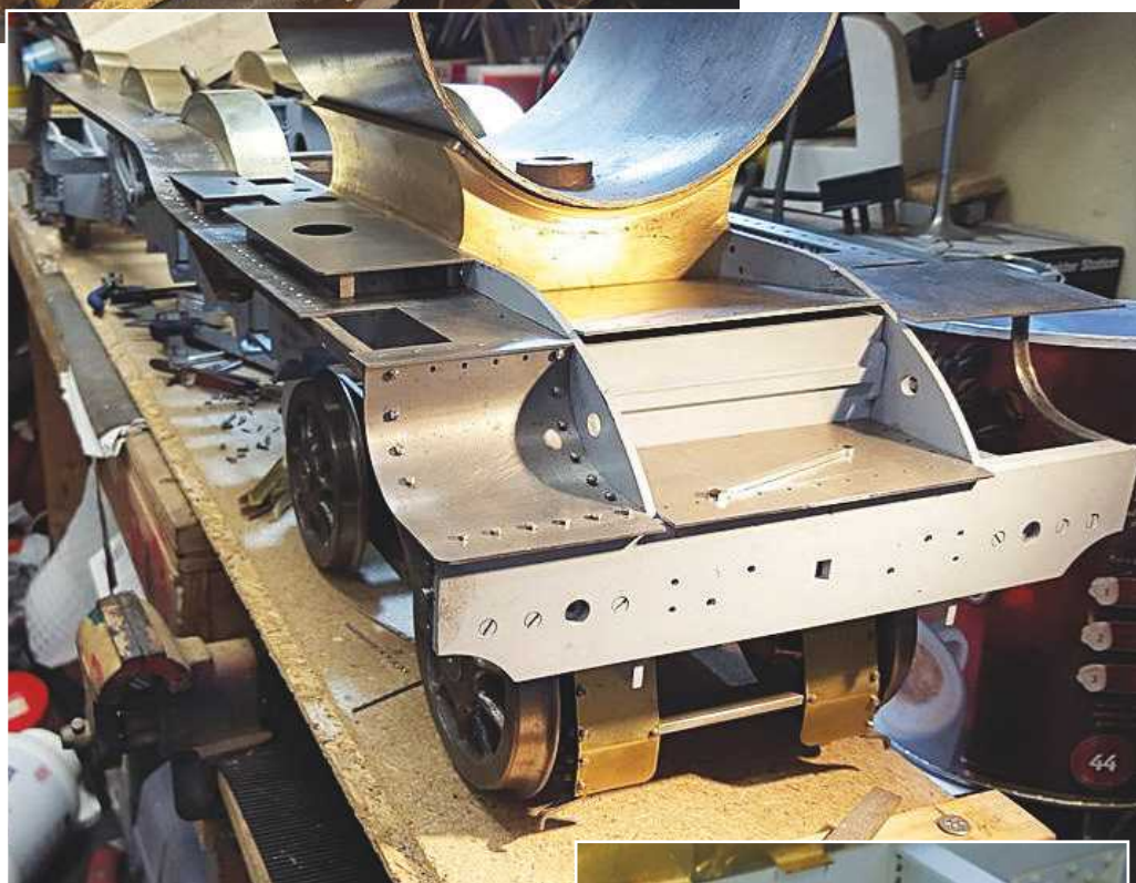
18. Here we have the long valve cover in place to check for position. I needed to shorten it a little along the rear edge as it was a little long. Later I'll fabricate the upright sections but for now it's just sitting on some steel stock so I can check all is as should be.
