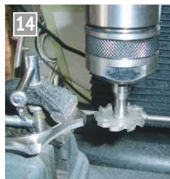
Machining the slot in the brake shoe.
