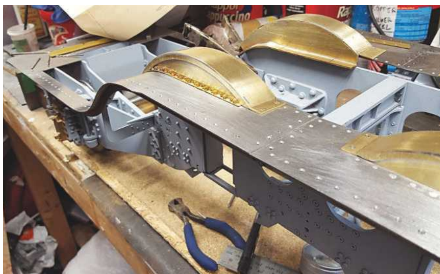
19. Lastly, the extra right angle along the splasher/running board joint. I have used 12BA bolts but may change these to 14BA as they look a little large to me. The bolts are fitted as dummies with the drilled holes countersunk from underneath and filed down.
