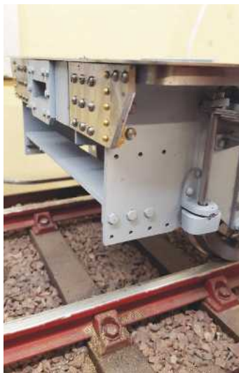
7. Lastly for the valance fixing, this picture shows how the valance curves around the back of the cab floor and is secured behind the drag beam.
