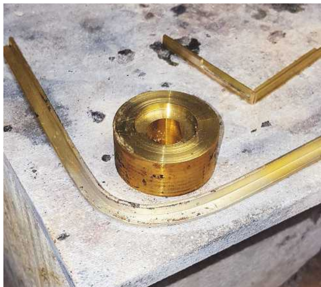
11. Using some rusty blocks I clamped the sections in place for two of the axes with the third curved part lying flat on the board. I mixed up a semi-thick flux paste and silver soldered the parts together, ensuring that the curved section was at the correct angle. I drilled the mounting holes for securing to the frames first and the 10BA tapped holes for the boards will be done in situ.
