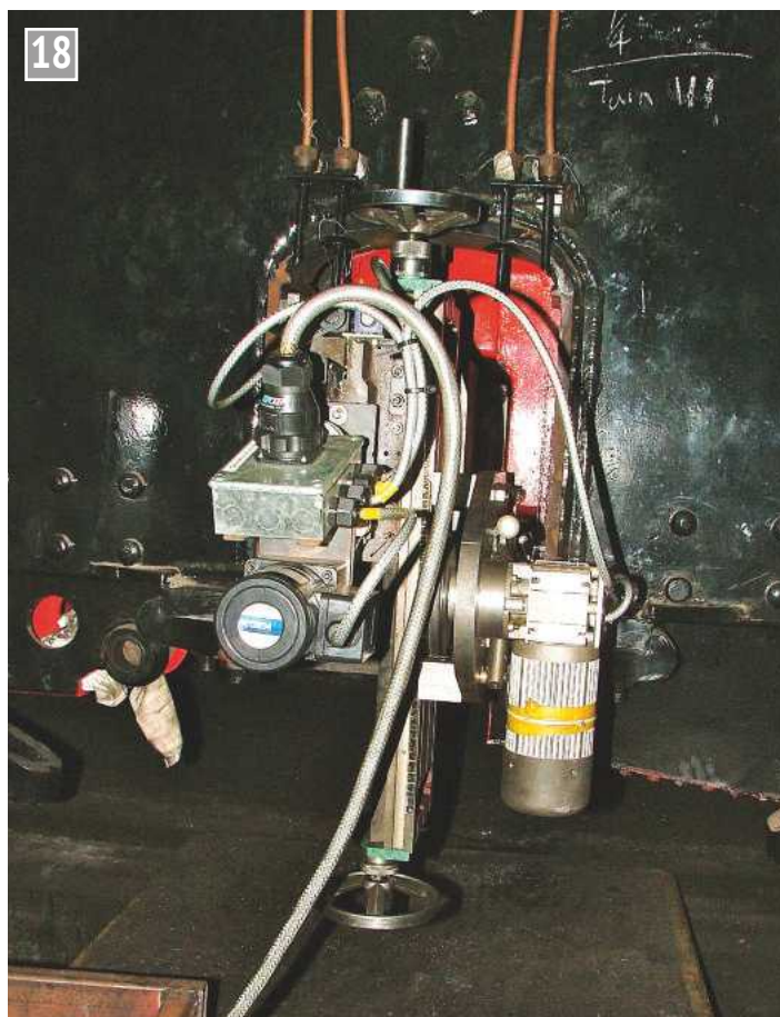
General view of the machine in position, after the addition of the powered cross feed and associated controls.
