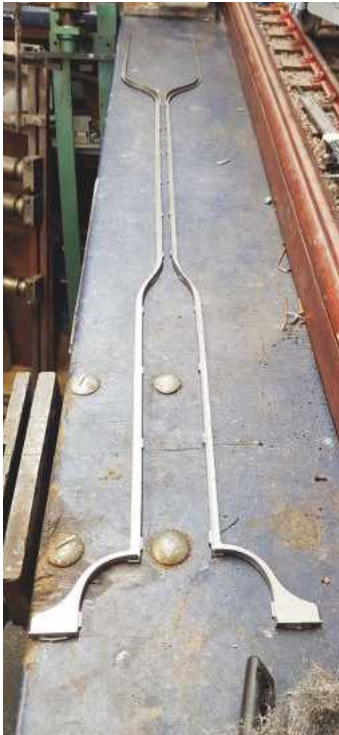
2. This picture shows the laser cut parts assembled, I did the curved top sections by hand using whatever radius bar was nearby to help shape the parts to match the valance profiles.
