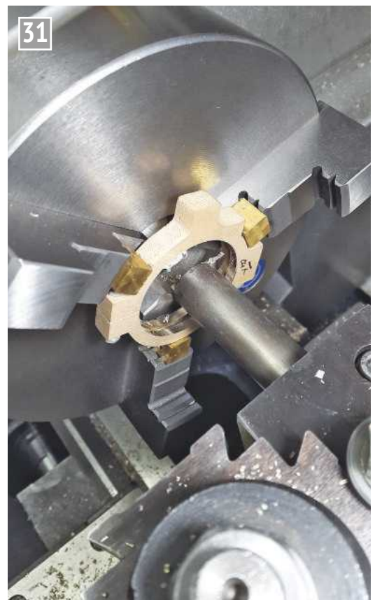
Machining the eccentric strap groove.
