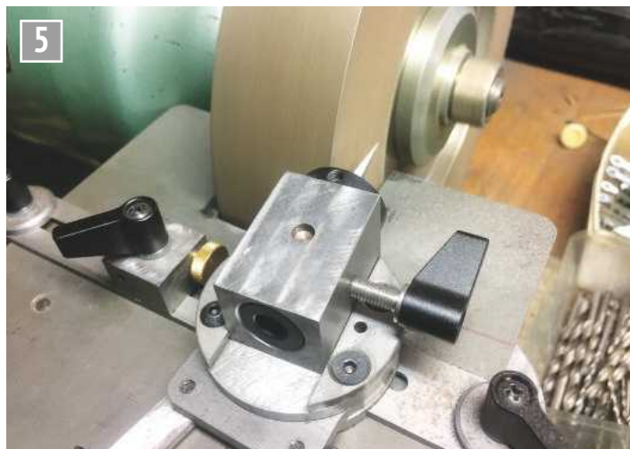
Grinding a three-sided reamer.
