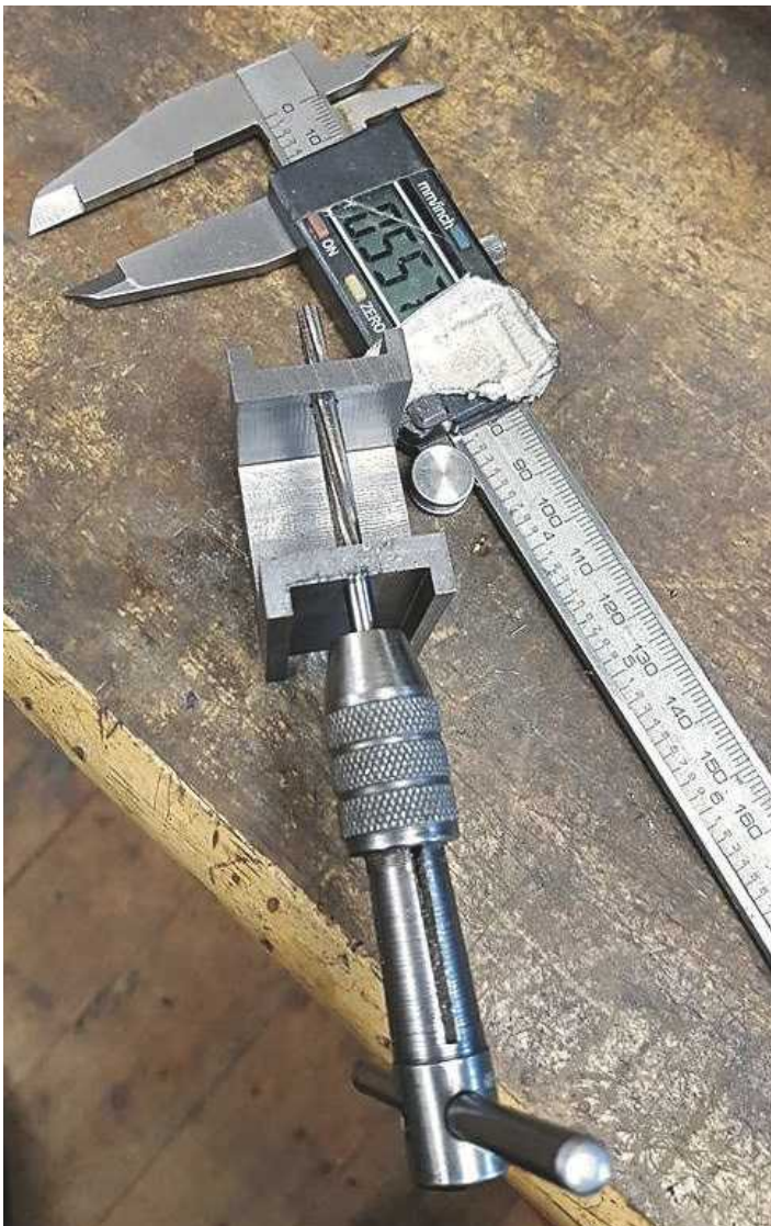
5. I then reamed the spring buckle pin hole to size.
