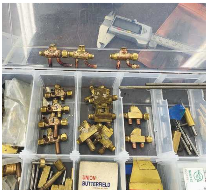
A special box for all the injector bits; jigs, spacers and tooling.
