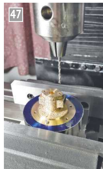
Drilling the cylinder gland stud holes
