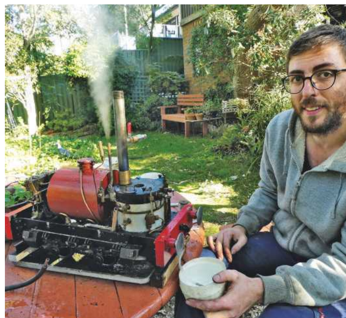
Andrew injector testing using a 5 inch gauge model Sentinel locomotive.
