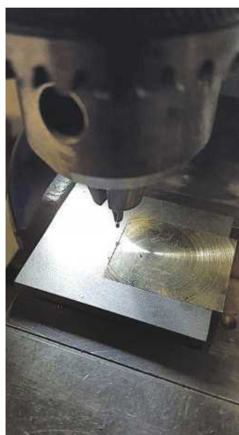
11. After plotting the right-hand side crank box centre (my datum) and then setting the vice, I spotted a small hole with a centre drill, as shown here.
