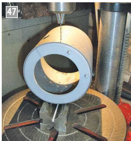
Drilling rivet holes in the smokebox.
