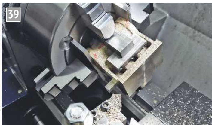
Facing the valve surface.
