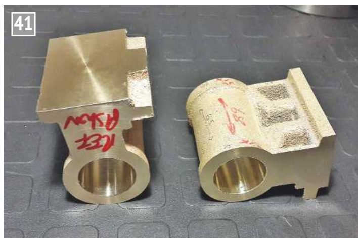
Cylinders ready to check piston fit.
