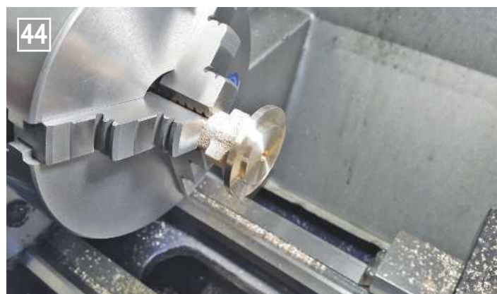
Machining the piston rod side end caps.
