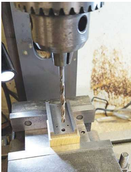
FAR LEFT: 7. Here are the keep blocks having been machined to size for the axlebox slots. The two extra brass blocks are spares.
