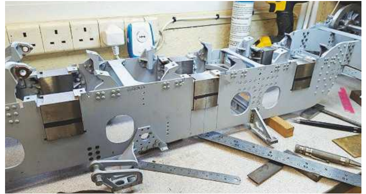
4. This shows the boxes marked ready for having the keep slot machined. This was a straightforward operation and was followed by drilling the oilways into the axlebox. The spring buckle pin holes are on the same centre line as the oilways so I drilled those too using packing to stop any flexing of the job. The last drilling job in this set-up was the \frac{1}{16} holes for the keep retaining pins. At first, I thought of trying to drill these straight through like the spring buckle pins but being so small there would most likely be some deflection. Also, I had no guarantee with the equipment to hand that if I drilled the holes separately through both sides that they would match perfectly the keeps once drilled. Therefore, I decided to just drill one side and when the keeps are machined for a tight fit in the slots I'll drill through these two reference holes, through the brass keep and out of the other side of the box.
