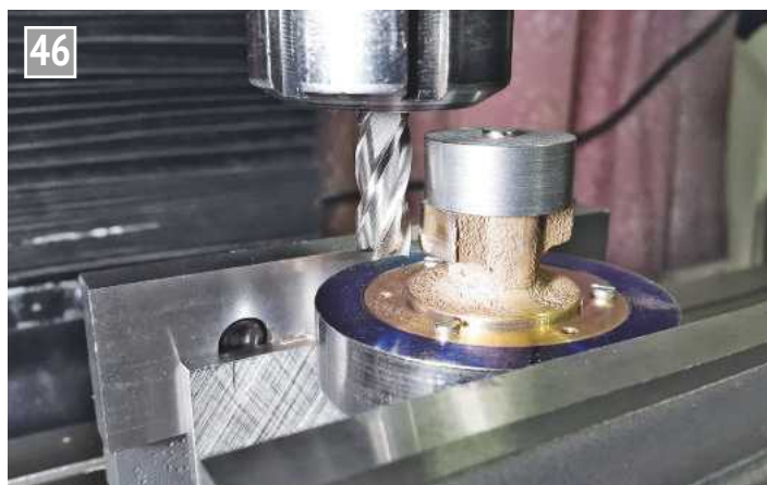
Machining the crosshead slider rests.
