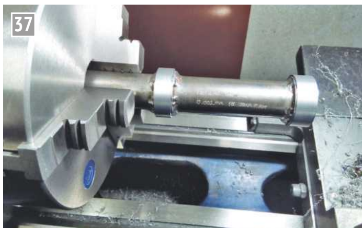
Lathe bed twist check - test bar.
