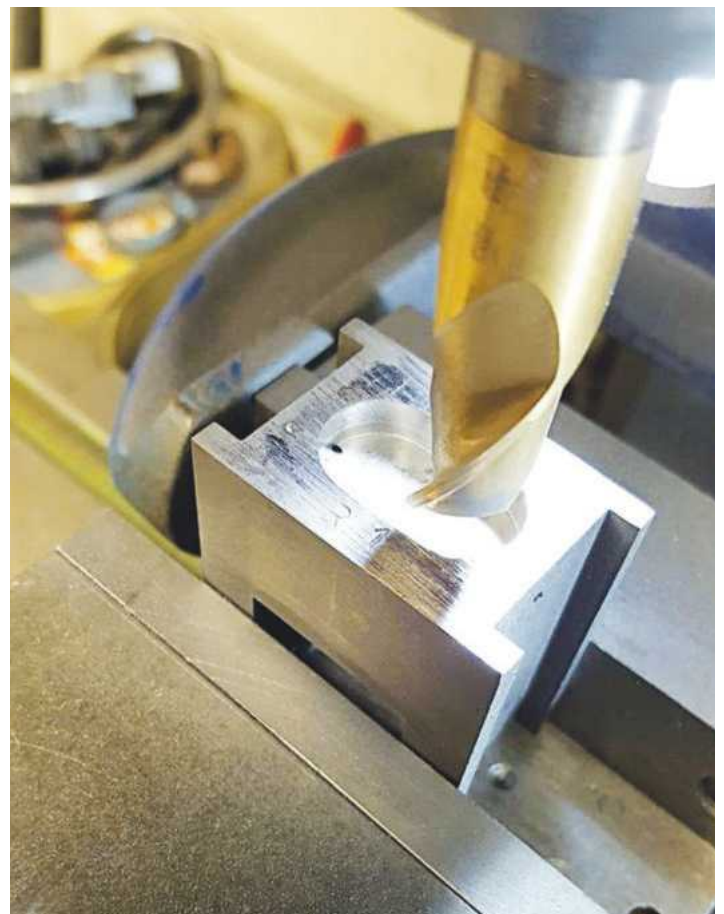
6. Next was to machine the oil reservoirs on top of each box. You can just see one of the oil-way holes breaking through as it should.
