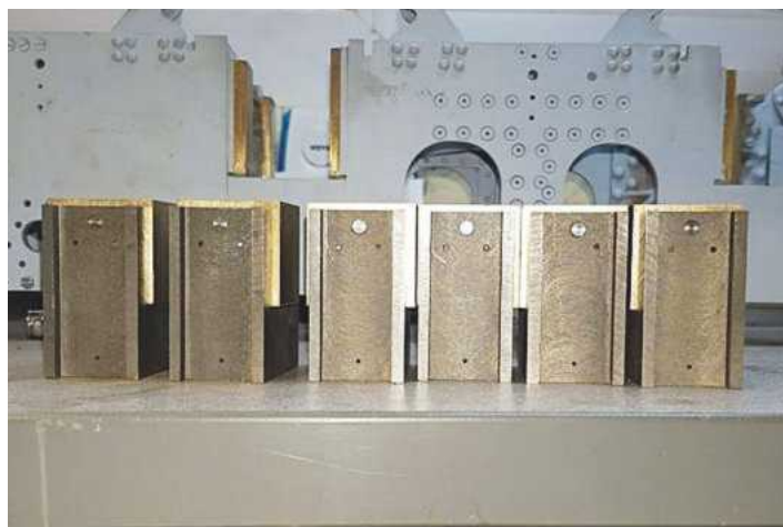
RIGHT: 9. Here are all six axleboxes, with keeps, retaining pins and spring buckle pins fitted.
