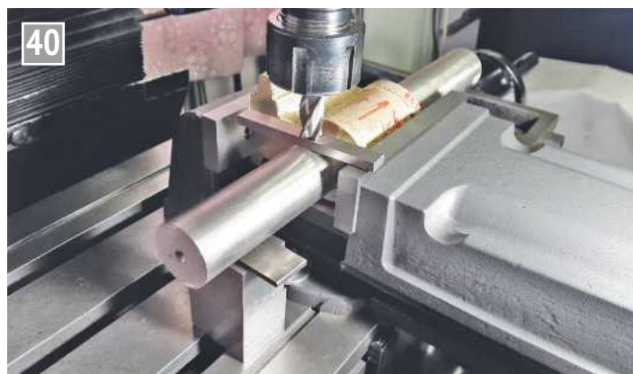
Milling the frame cutout.
