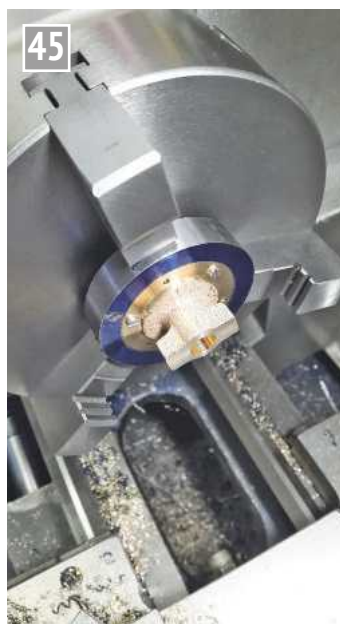
End cap machining in jig.
