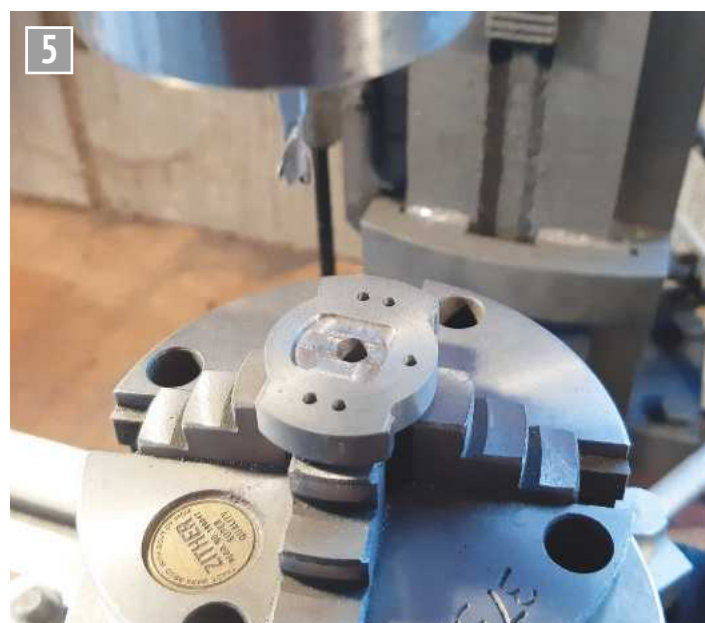
Milling the port block.
