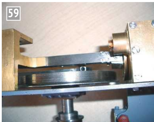
59 Clearance problem on the crosshead.
