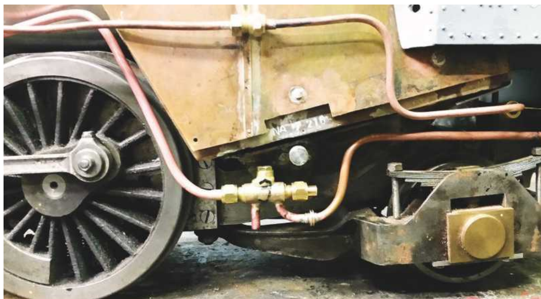
One of Andrew's 14 oz injectors test fitted to a 3 1/2 inch gauge Britannia under construction.
