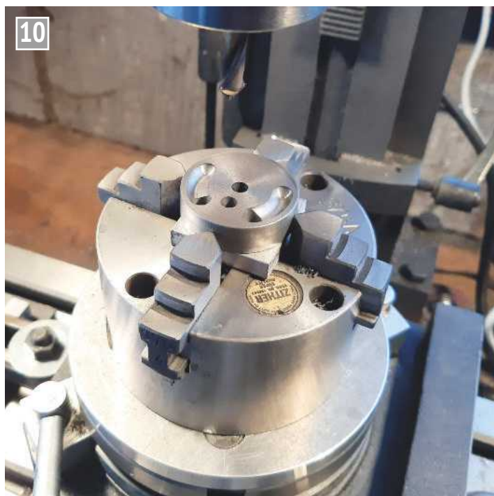
Milling/drilling the flywheel/crank.
