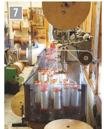
Twine making machine in Outhwaite's ropeworks.
