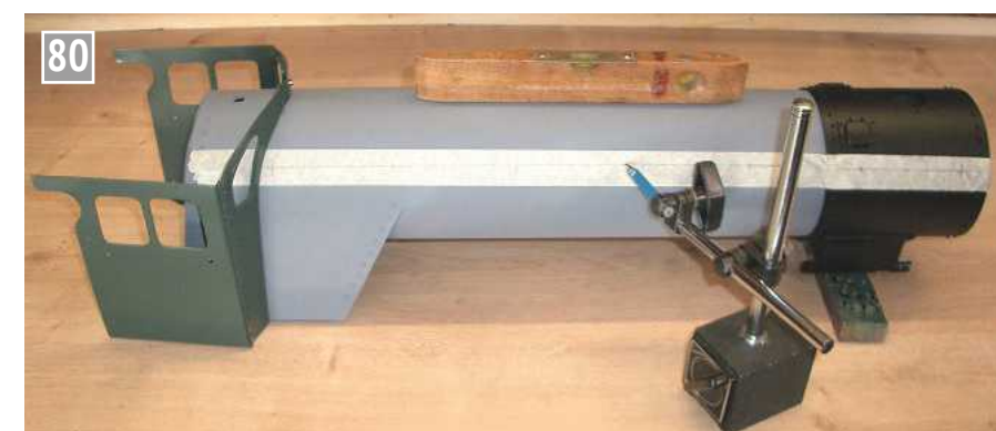
80 Marking out for the handrail stanchions.
