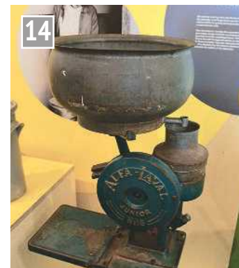
To make butter high fat cream is separated out using similar machines. It was difficult to make a machine that ran at the steady speed required.
