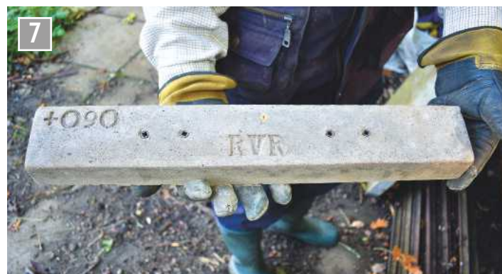
One of the new concrete sleepers with the gauge widening dimension clearly shown.
