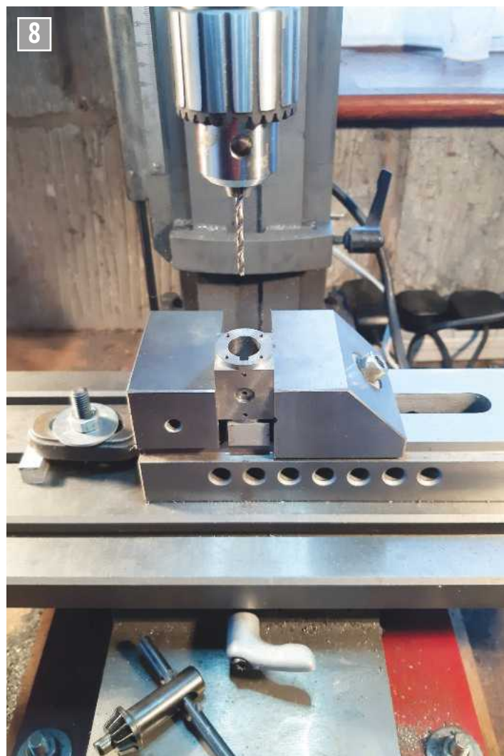
Drilling the port holes.
