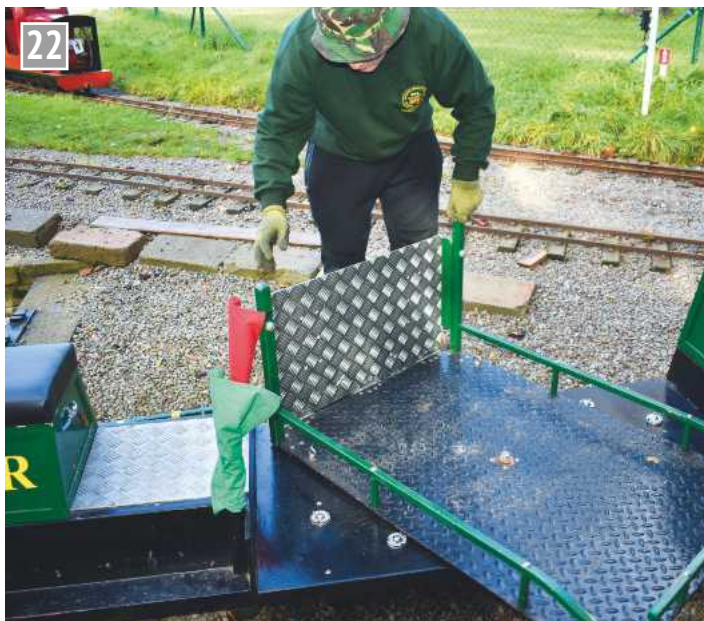
22 The club-built disability carriage demonstrating the swivel action of the platform.
