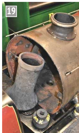
The massive blast pipe on the Garrett.
