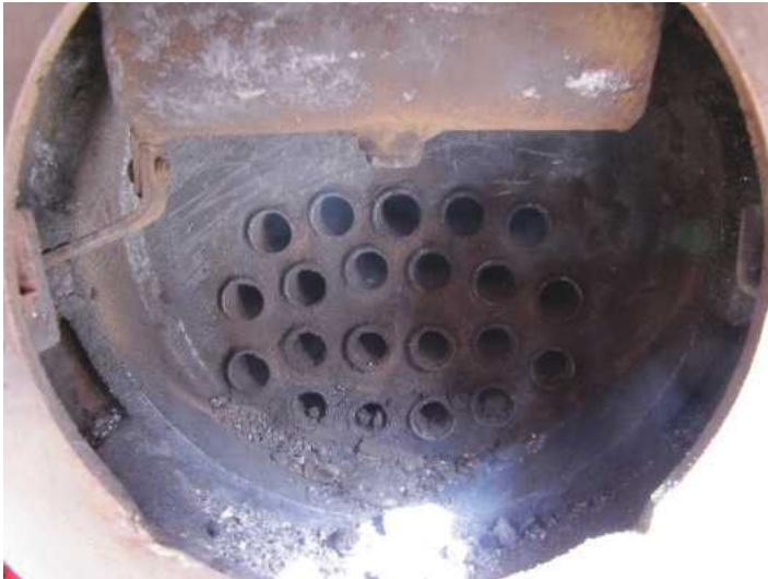
The silencer baffle is visible inside the smokebox above the tubes.
