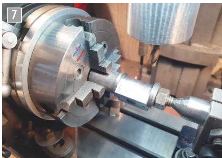
Machining the front of the cylinder.
