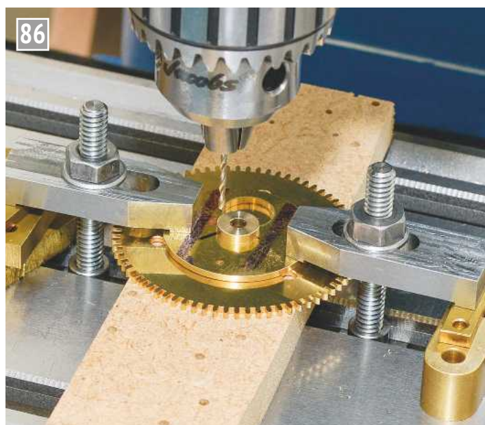
Drilling through the washer and hour wheel.
