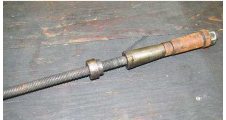
The tube expander made overnight to allow Richard to continue to steam up.
