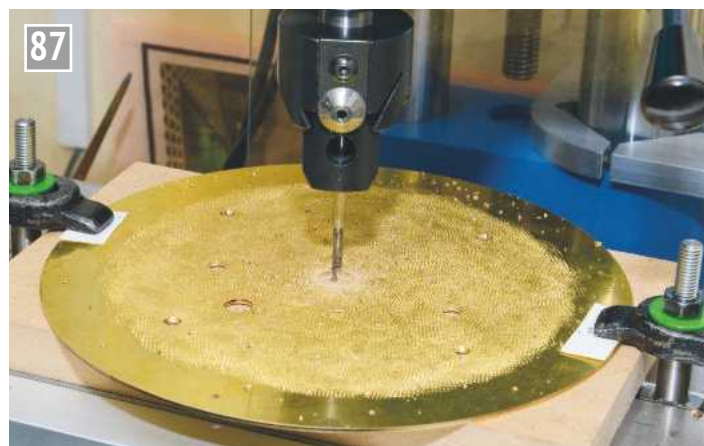
Opening up the centre hole in the front face.
