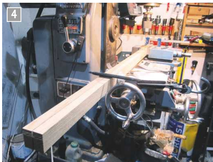
Drilling the bolt holes.
