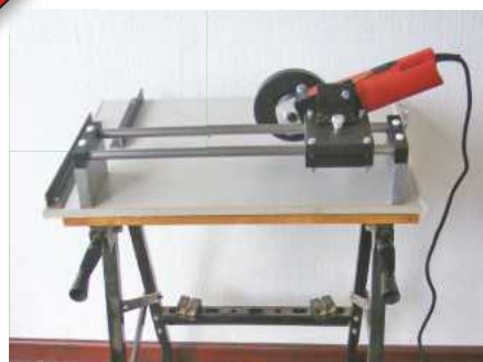
Mike Cox makes a sliding holder for an angle grinder.
