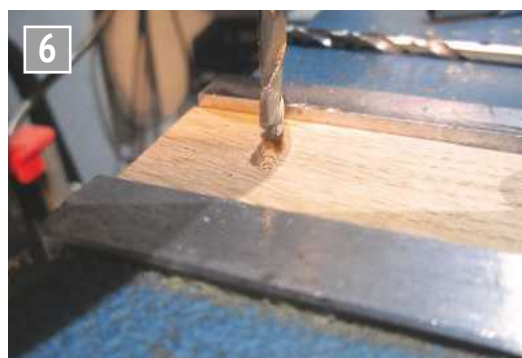
Milling the slot.
