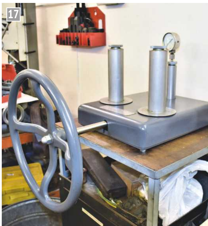
The dead load tester ready for testing pressure gauges.
