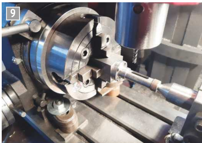
Milling the slot in the big end guide.
