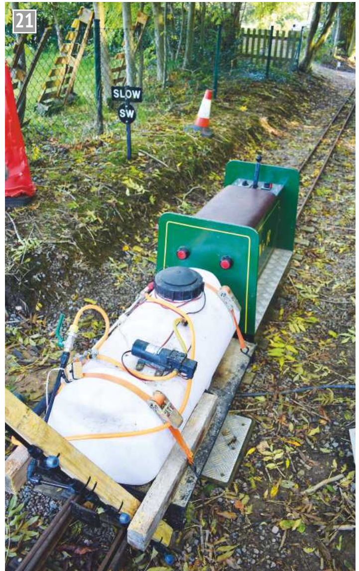
21 The weed killing tank wagon and its dedicated engine.
