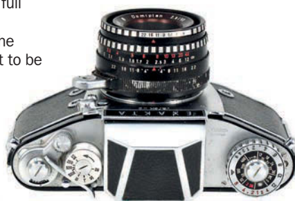
View from the top, showing the delayed action knob on the right that doubles as a slow speed setting device
