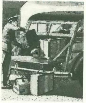
**EVEN WITH** all 8 passengers seated, there is still room for luggage. The end-gate is sturdily built—it will support as much as 400 lbs. Both gates, upper and lower, close tightly and may be locked.
