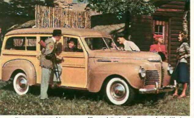
WORK OR PLAY, this smart new Plymouth Station Wagon completely fills the bill. The big, handsome body of natural-finish maple and ash is built on the long wheelbase, De Luxe Plymouth chassis, giving it a remarkably smooth ride. Auxiliary seats are quickly removable and interchangeable.
