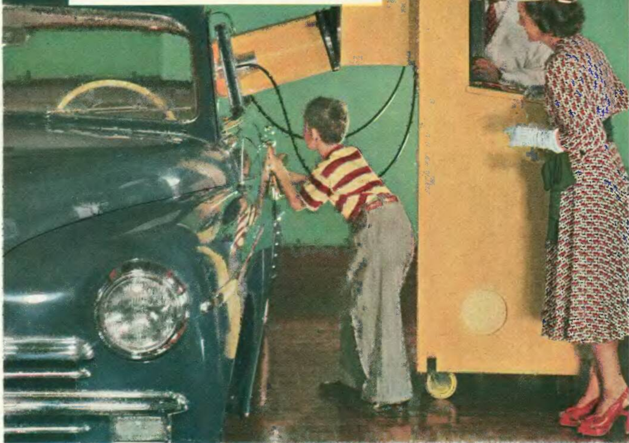
Body seal test of new Plymouth car, practical imagination at work at Chrysler Corporation
