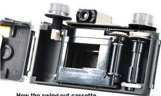
How the swing-out cassette holder helps to make film loading easy
